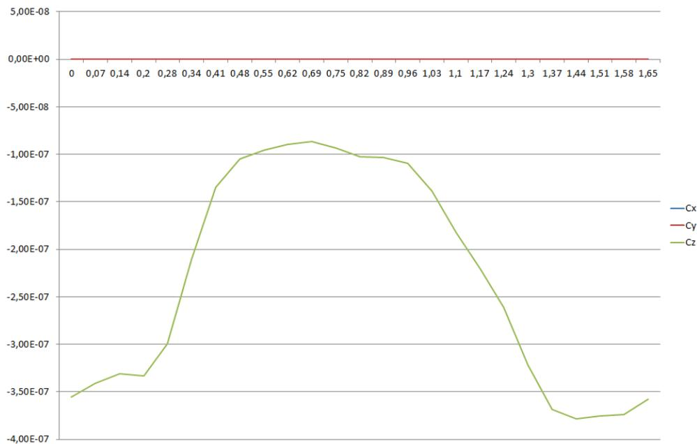
Figure 14.9: ESABASE results of the aerodynamic torque, expressed in the satellite reference frame. The x-axis of the diagram is the time in hours, while the y-axis is the torque in Newton meters.
