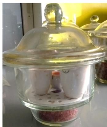
Figure 24: Desiccator with crucibles
