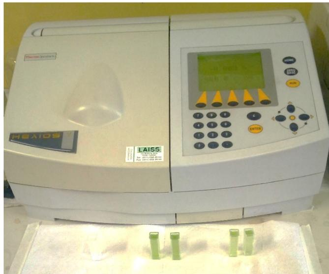
Figure 22: Spectrophotometer and cuvettes
