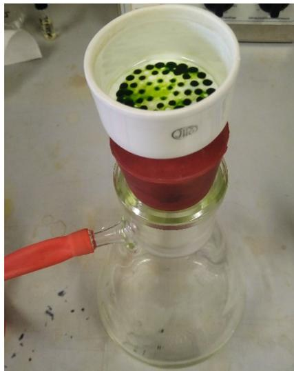
*Figure 25: Paper filter and Buchner funnel*
