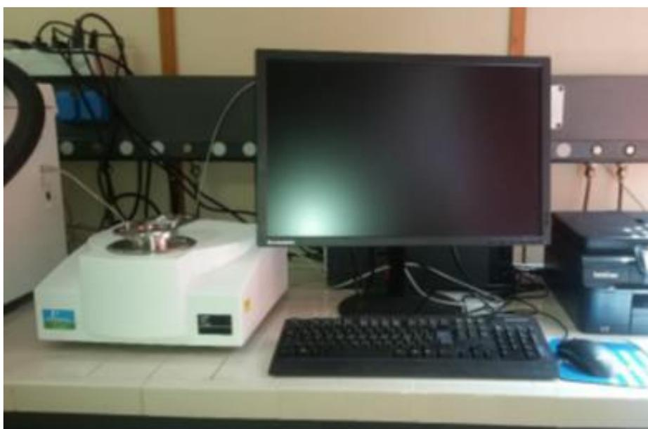
*Figura 27: Simultaneous Thermal Analyzer (STA) 6000*
