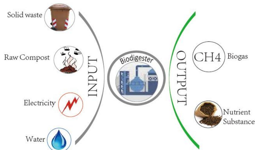
Map 56: Input - Output of Biodigester
