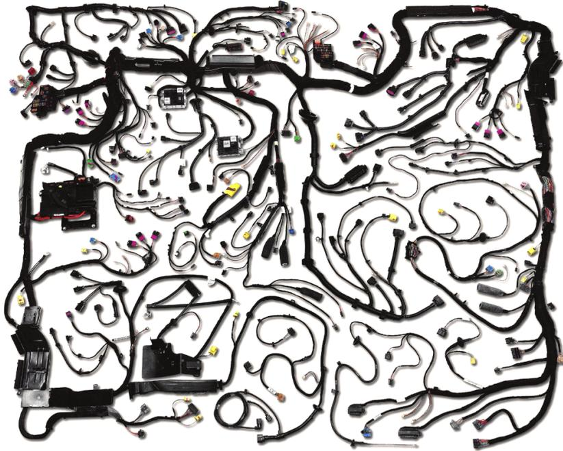
Figure 2.1: Typical wiring harness in a car.
