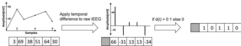
**Figure 1.6:** Starting from the raw iEEG signal I evaluate the temporal difference; later I construct the Local Binary Pattern code of 1 and 0, depending if differences is positive or negative.
