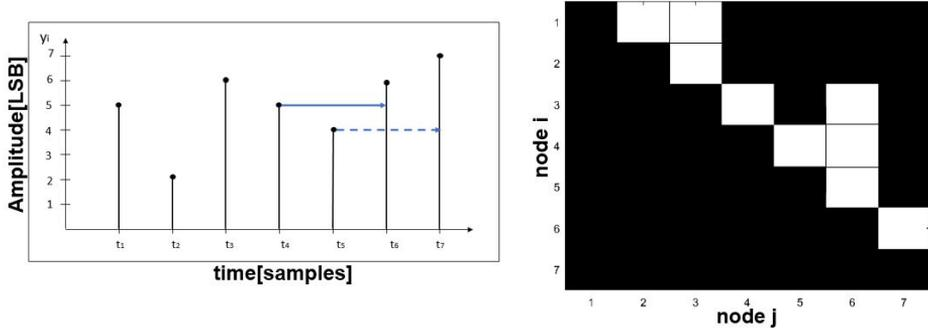
**Figure 1.4:** The procedure to construct the dHVG matrix is simple: let’s take a single time sample and compare it to all the successive ones: if there is no points in between with value higher than the one of the two time samples under analysis, a link is drawn (continue row in left graph); otherwise, a continue horizontal line can’t be drawn between the two time samples, because there is an higher  $y_i$  in between. Hence, there is no link between the two points.
