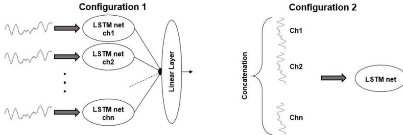
**Figure 3.5:** Long-short term memory configurations. In the first configuration, a single LSTM is used for each channel and the output are then merged through a Linear Layer. In the second configuration, the LSTM works on a bigger time window, created with the concatenation of all the input channels.
