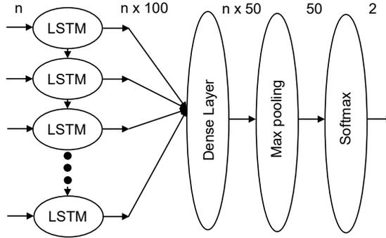
**Figure 3.6:** Long-short term memory architecture. The networks directly infer on raw iEEG data without any additional preprocessing stage. The two configurations used are build on top of that model, replicating it or feeding with bigger windows. The model is composed by a first LSTM layer with 100 neurons, a dense layer that reduces the dimensionality of the space to 50, a Max Pooling stage which has 50 features as output and a last softmax layer for the prevision.
