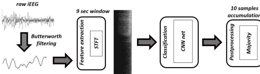
**Figure 3.7:** High level pipeline based on Convolutional neural network: in figure 3.9 can be found a much more detailed explanation of the network.
