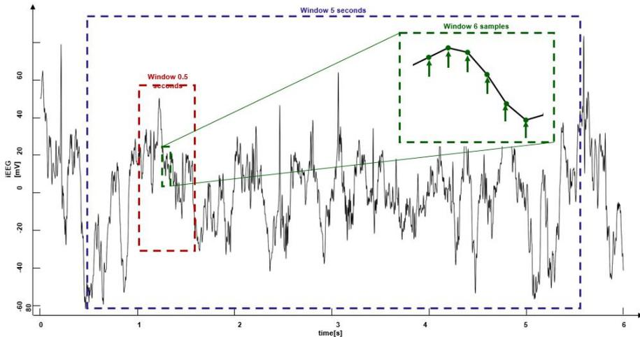
**Figure 2.2:** iEEG signal of a single channel. In green the window of points used to construct a single LBP symbol, shifted of 1 sample at a time (256 symbols inside a window of 0.5 seconds); in red the 0.5 seconds not-overlapping window used to construct the histogram; in blue the bigger time-window (5 seconds length, 0.5 seconds shifting) used to compute the final prevision.
