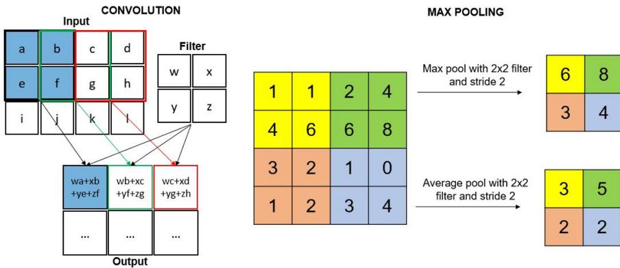
**Figure 3.8:** On the left a convolutional layer with a single filter and a 2D input is represented. On the right, the max and the averaging pooling for a 2D input are shown.
