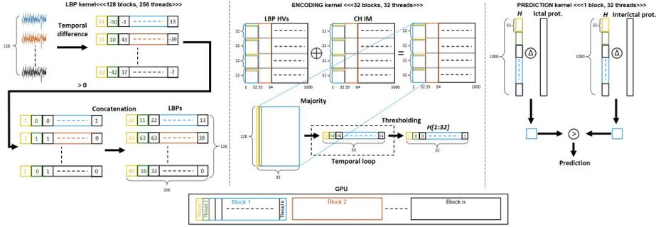
**Figure 5.2:** Parallelization of the algorithm on a GPU. For each kernel, 2 threads and 2 blocks are highlighted to show the distribution of the operations inside the GPU.
