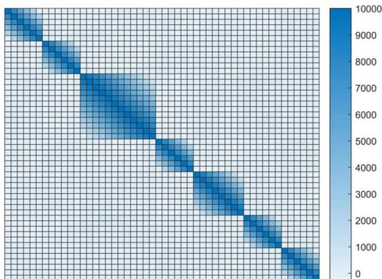
**Figure 2.8:** IM designed to encode the similarity between electrodes in five 6-electrodes strips, one 8-electrodes strip and a 12-electrode one.
