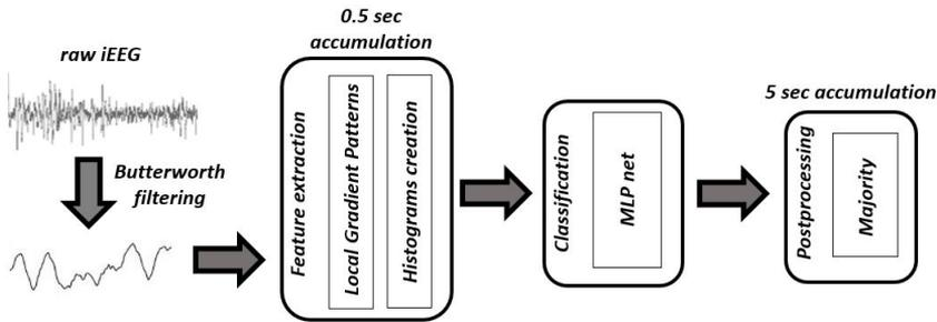
**Figure 3.2:** Pipeline for the MLP: the steps are again similar to the ones of figure 2.1, with a changing in the symbolization for the preprocessing, changing the local binary patterns in local gradient patterns.
