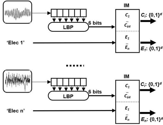
**Figure 2.3:** In this stage I extract from each electrode the LBP code and the electrode name (i.e. the ID). After that, I project them in the hyper-space through two item memories properly constructed.
