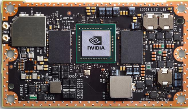
**Figure 5.1:** Jetson Tx2 platform, an AI supercomputer features NVIDIA Maxwell architecture, 256 NVIDIA CUDA cores, 64-bit CPUs, and a power-efficient design.
