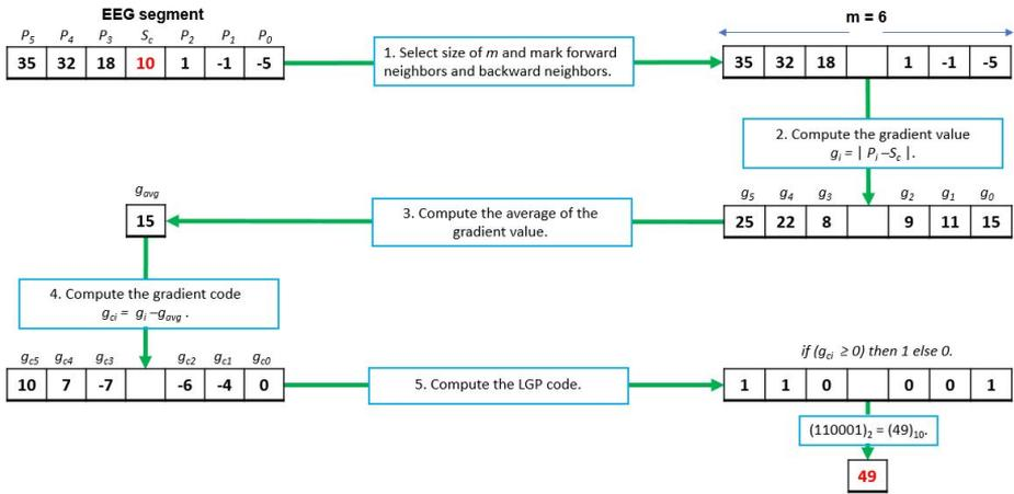
**Figure 1.8:** Shows all the step for the construction of LBP code for a single time sample  $S_c$ .
