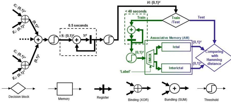
**Figure 2.4:** Starting from the hypervectors of name and values of electrodes, the classifier construct  $S$ : this hypervector encodes the spatial information among all the electrodes. After that, all the  $S$  in a window of 0.5 sec are added and the *histogram*  $H$  is created. Finally, there is a split: during the training phase all this  $H$  will contribute to construct the AM; conversely, during the test, the classifier gives an initial label to the window.
