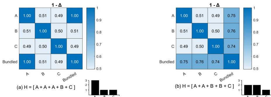
**Figure 1.3:** Similarity between three atomic vectors and two different encoded histograms. (a) symbol  $A$  occurs more than 50% of time, whereas (b) no symbol occurs more than 50% of time.
