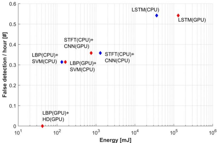
**Figure 5.3:** Comparison of my algorithm with state-of-the-art methods in terms of energy and false detection / hour. Energy per classification is plotted on the x-axis, mean false detection/hour on the 18 patients is on the y-axis.
