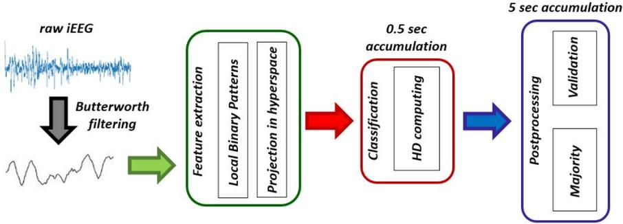
**Figure 2.1:** Binarized seizure processing chain: (1) Feature extraction generates a 6-bit LBP code for each electrode and projects these codes into  $d$ -dimensional space; (2) HD processing constructs vector  $H$ , which represents the histogram of 0.5s recording; (3) As postprocessing, a simple patient-dependent majority voting decides based on the last 10 labels; for the long time recordings a validation of that window as been added to reduce the false alarms.
