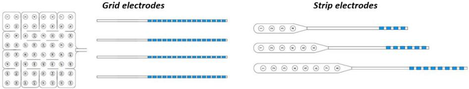
**Figure 2.9:** Grid and strip electrodes. After surgical implantation, the electrical activity is recorded through the blue pins on wires that come out from the heads. Patients with this type of electrodes are under constant monitoring.
