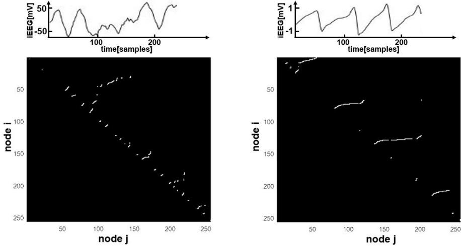
**Figure 1.5:** On the left the connection matrix for the interictal signal shown above, on the right for an ictal signal. In both the connection matrix the superdiagonals have been removed; in fact, since I want to compare the two connection matrix, is meaningless to keep a constant bias.
