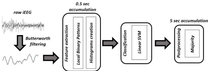
**Figure 3.1:** Pipeline for the SVM: the steps are identical to the ones of HD computing, only with a substitution of the classification paradigm.
