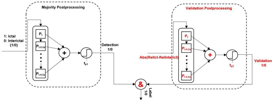
**Figure 2.6:** Both windows of postprocessing of the algorithm: the left one, a majority on the last ten samples, is used for both the datasets; the validation postprocessing has been added to avoid a high number of false detections.
