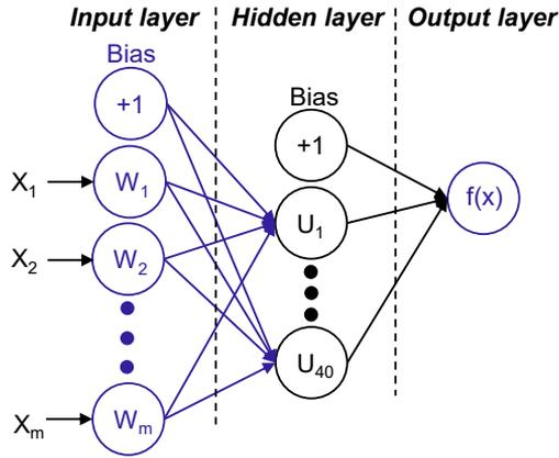
**Figure 3.3:** Multi Layer perceptron net is a fully connected net: the input layer is composed by  $m$  nodes, where  $m = \#(\text{channels}) * \#(\text{LBP}_{\text{codes}})$ , the hidden layer is composed by 40 neurons, the output estimate the probability of the input to belong to the ictal class.
