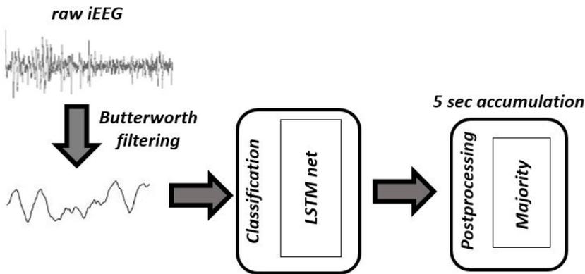
**Figure 3.4:** The pipeline based on the long-short term memory pipeline is simpler: the net directly works on the raw signal, extracting automatically the features from the signal.
