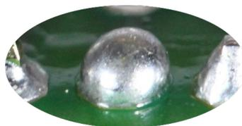
Figure 15: PCBA Defect - Solder Excess
