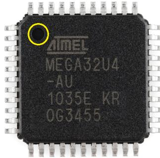
Figure 21: IC Device - Polarization Mark
