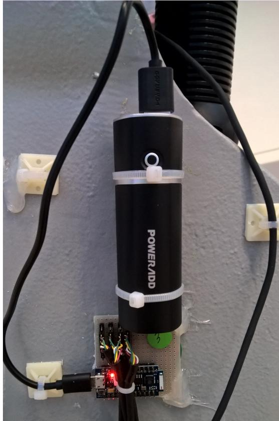
Figure 4.7: Breadboard with connected micro-controller, wire terminals and power supply.
