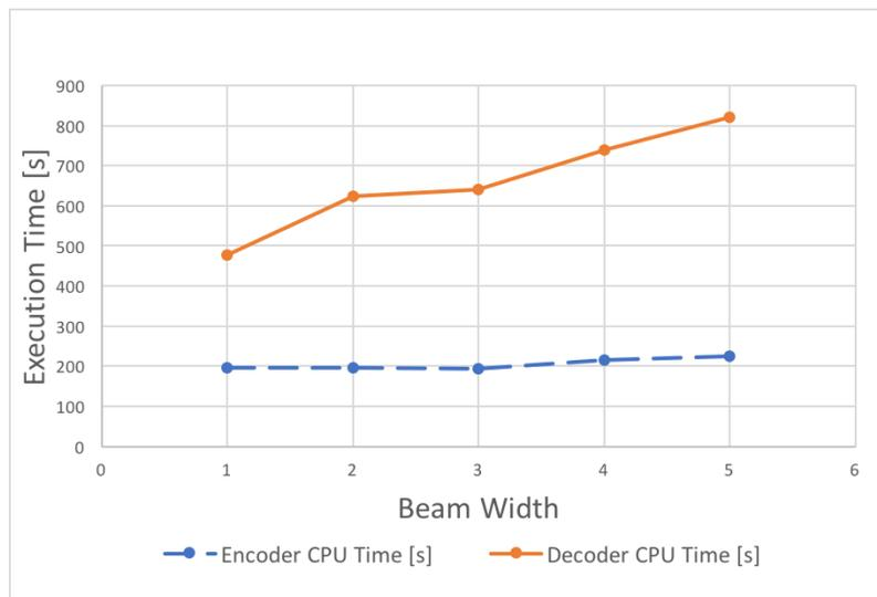
Figure 4.5: OpenNMT Beam Search complexity trend DE-EN model
