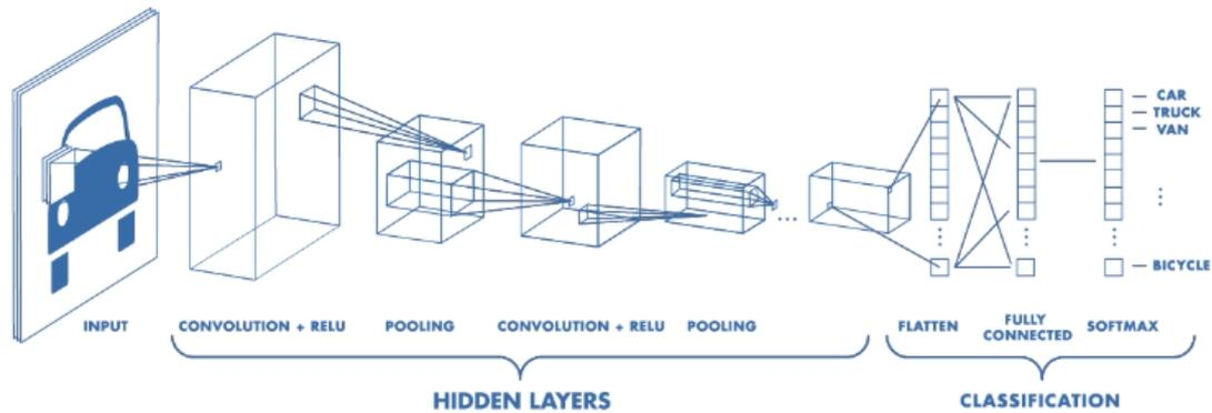
Figure 2.7: Architecture of CNN, source: <https://.it.mathworks.com/videos/introduction-to-deep-learning-what-are-convolutional-neural-networks>
