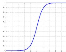
Figure 2.3: Tanh activation function and graph respectively
