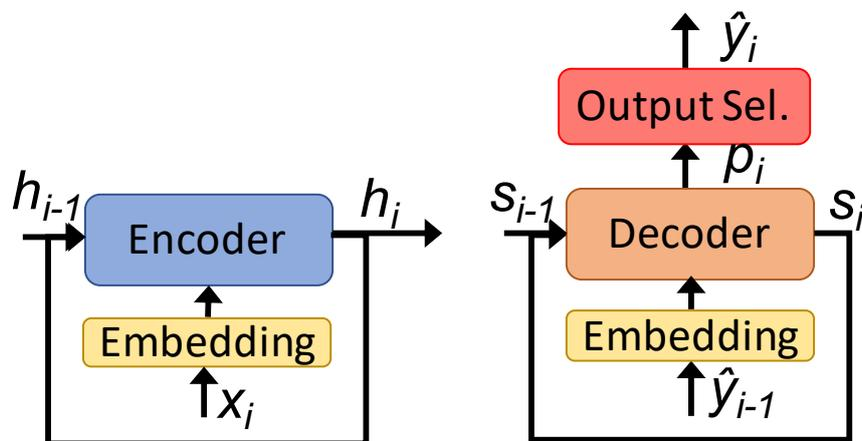
Figure 2.13: Encoder-Decoder RNN architecture
