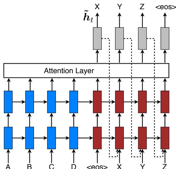
Figure 2.17: Input Feeding approach, picture taken from [2]
