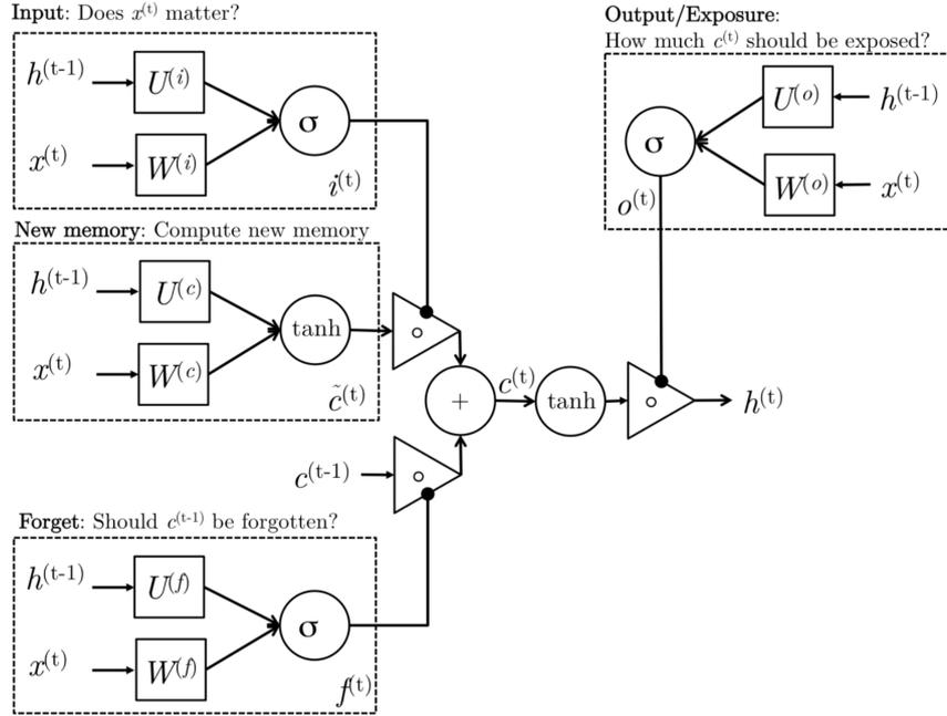
Figure 2.10: LSTM architecture, picture taken from [1]
