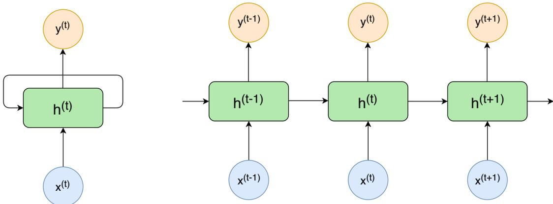
Figure 2.8: Recurrent Computational Graph
