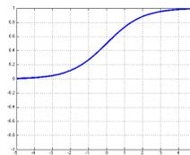
Figure 2.2: Sigmoid activation function and graph respectively
