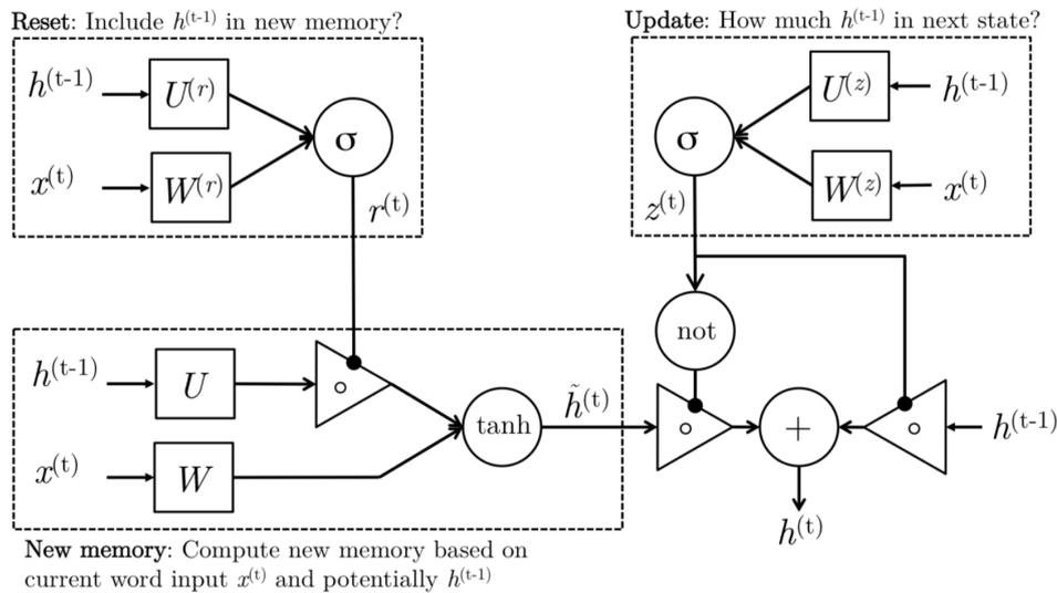
Figure 2.11: GRU architecture, picture taken from [1]
