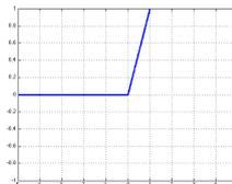
Figure 2.4: ReLU activation function and graph respectively
