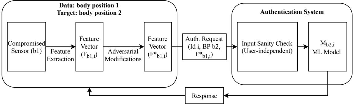
Figure 5.2: Evasion with user data as starting point. The adversarial instance is crafted modifying  $F_{b_1,i}$ , which is a genuine sample of user  $u_i$  collected from body position  $b_1$ . The feature vector  $F^*_{b_1,i}$  is attached to an authentication request for user  $u_i$  and body position  $b_2$ . If the attack is successful  $F^*_{b_1,i}$  is recognized as  $F_{b_2,i}$  and the adversary gains access to the system.
