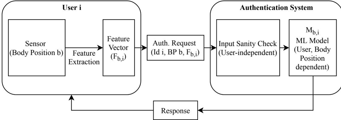
Figure 4.1: Authentication Process for user  $u_i$ . From a sensor in body position  $b$ , features  $F_{b,i}$  are locally extracted. The authentication request  $AR(i, b, F_{b,i})$  containing the user identifier  $i$ , the body position  $b$  and the feature vector is submitted to the authentication system. The request must pass an input sanity check before being evaluated by the model  $M_{b,i}$ .
