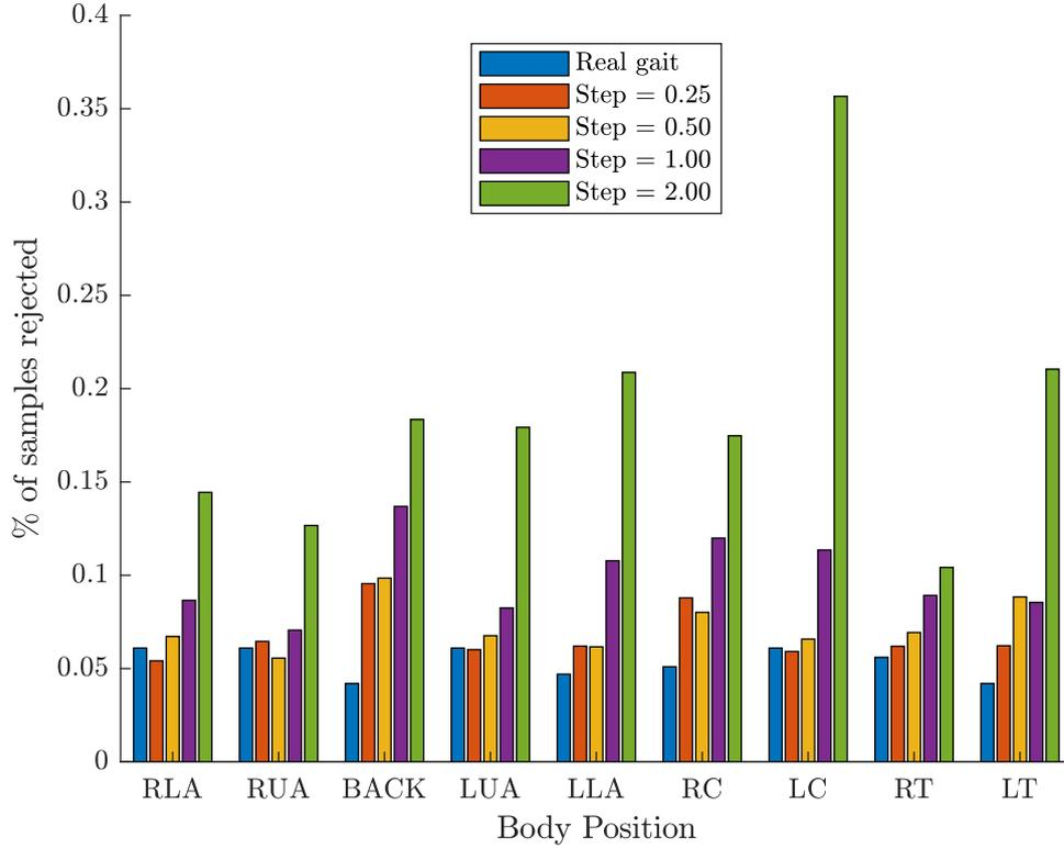
Figure 6.3: Adversarial samples rejected by body position and maximum step size. Comparison with real gait data.
