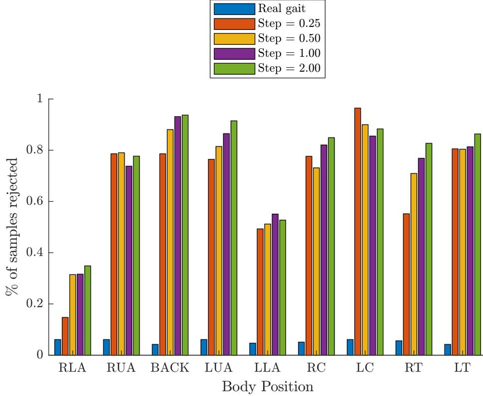
Figure 6.7: Adversarial samples rejected by body position and maximum step size. Comparison with real gait data.
