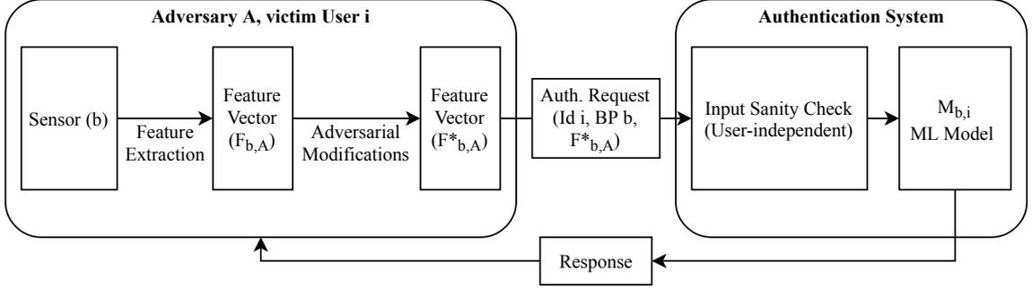
Figure 5.1: Evasion with adversary data as starting point. The feature vector obtained from a sensor placed on the adversary  $A$  in position  $b$  is modified to obtain an adversarial instance  $F^*_{b,A}$ . The sample is attached to an authentication request with identifier  $i$  of user  $u_i$  (victim), which is then submitted to model  $M_{b,i}$ . If the attack is successful  $F^*_{b,A}$  is classified like a genuine sample  $F_{b,i}$ .
