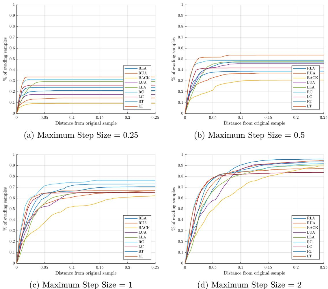
Figure 6.5: Comparison of the performance for different step sizes and different targets (body positions). Each points shows, given a distance threshold, the percentage of samples evading the model, for each body position.
