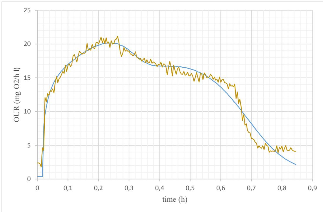
*Fig. 7.8 Observed OUR (brown line) and Simulated OUR with Calibrated Parameters (blue line) – Input Acetate 54.703 mgCOD/l*
