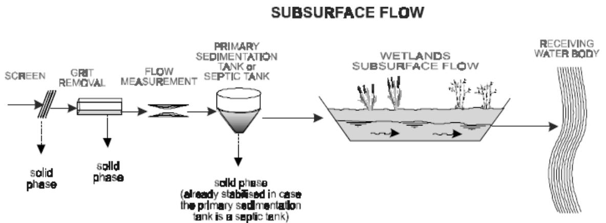
Fig. 2.2 Scheme of a typical Subsurface flow Wetlands
