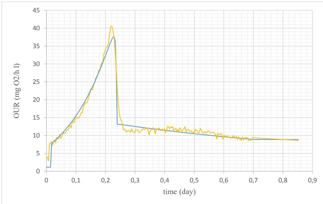
*Fig. 7.4 Observed OUR (brown line) and Simulated OUR with Calibrated Parameters (blue line) – Input Acetate 149 mgCOD/l*
