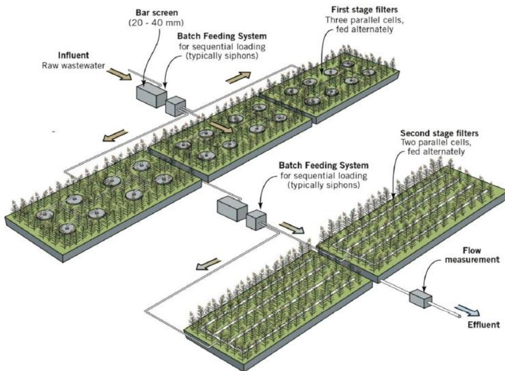
*Fig 3.5 Scheme of typical French Vertical Flow Wetland (Dotro, Günter, Molle, Nivala, & Puigagut, 2017)*
