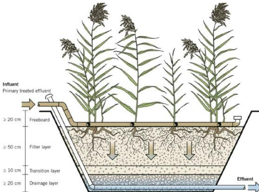
*Fig. 3.4 Scheme of typical Vertical Flow Wetland in Europe*
