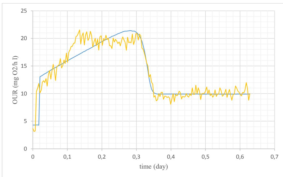
*Fig. 7.5 Observed OUR (brown line) and Simulated OUR with Calibrated Parameters (blue line) – Input Acetate 232 mgCOD/l*
