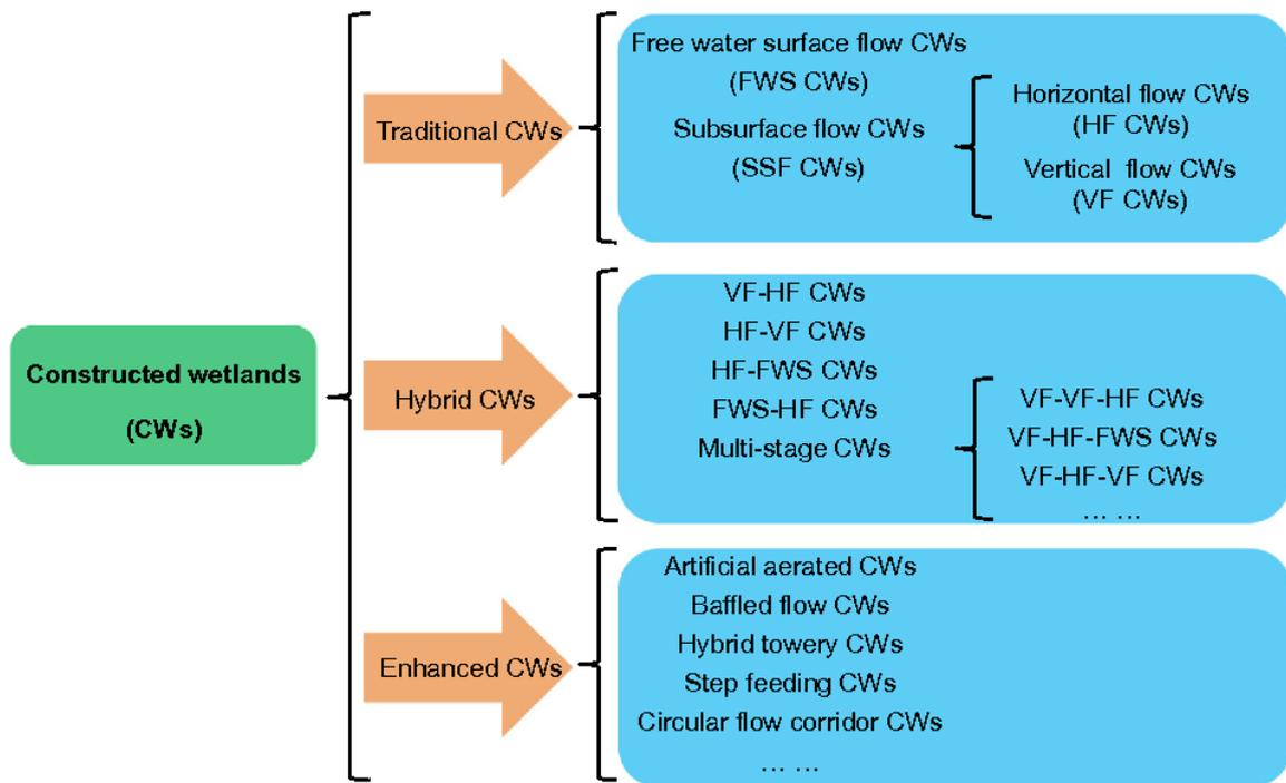
Fig. 2.1 Schematic representation of Wetlands Classification, (Wu, et al., 2014; Wu, et al., 2014).
