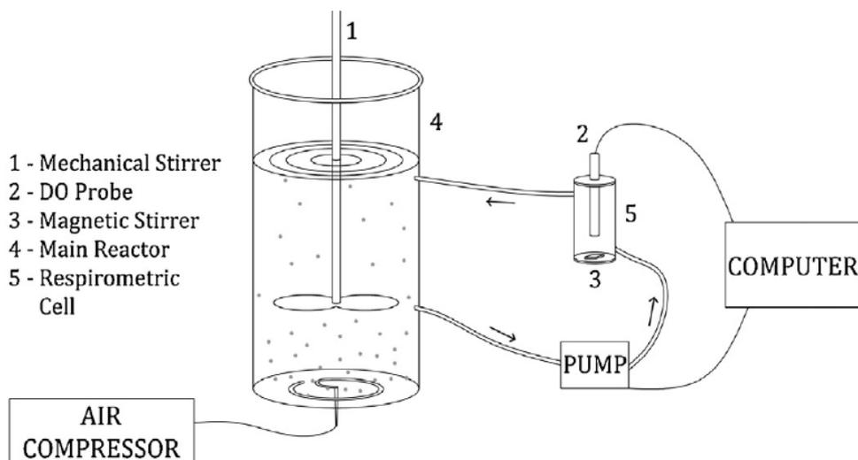
Fig. 6.1 Schematic representation of first type of Respirometry
