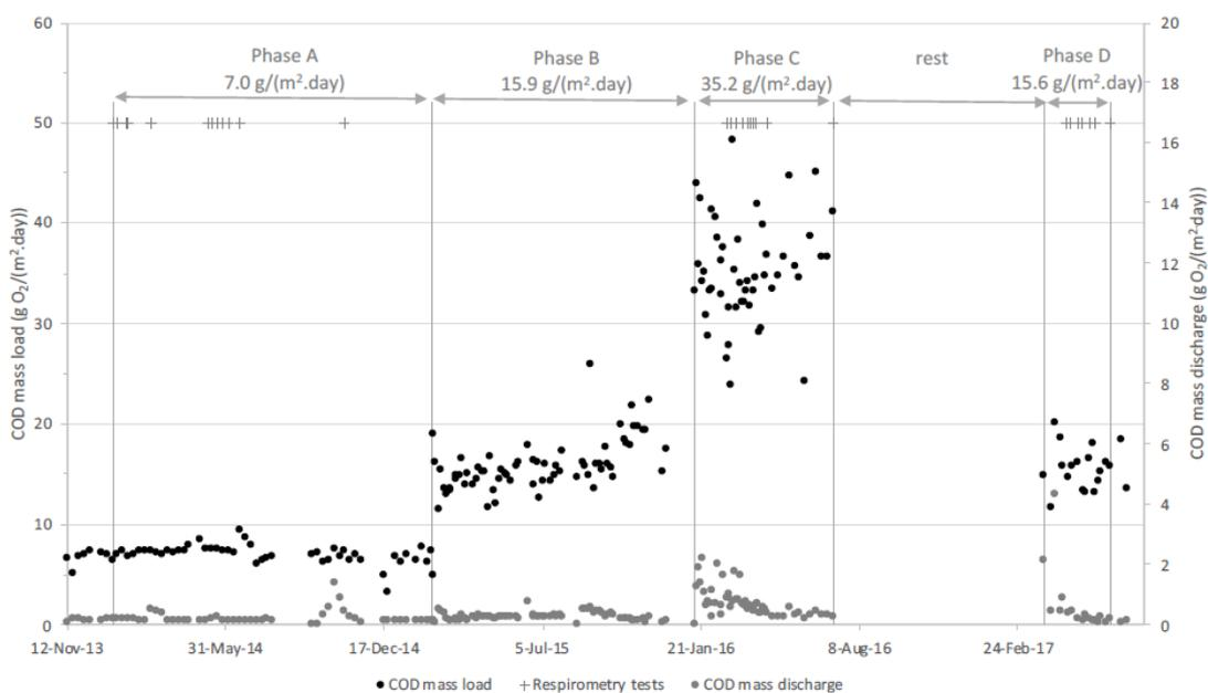
Fig. 6.3 COD mass loading rate (ML) applied to the experimental Wetland during the experimental phases of the study.
