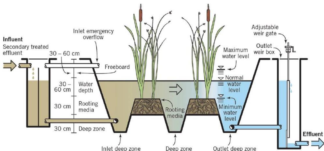
*Fig. 3.6 Scheme of Free Water Surface Constructed Wetland (Dotro, Günter, Molle, Nivala, & Puigagut, 2017).*
