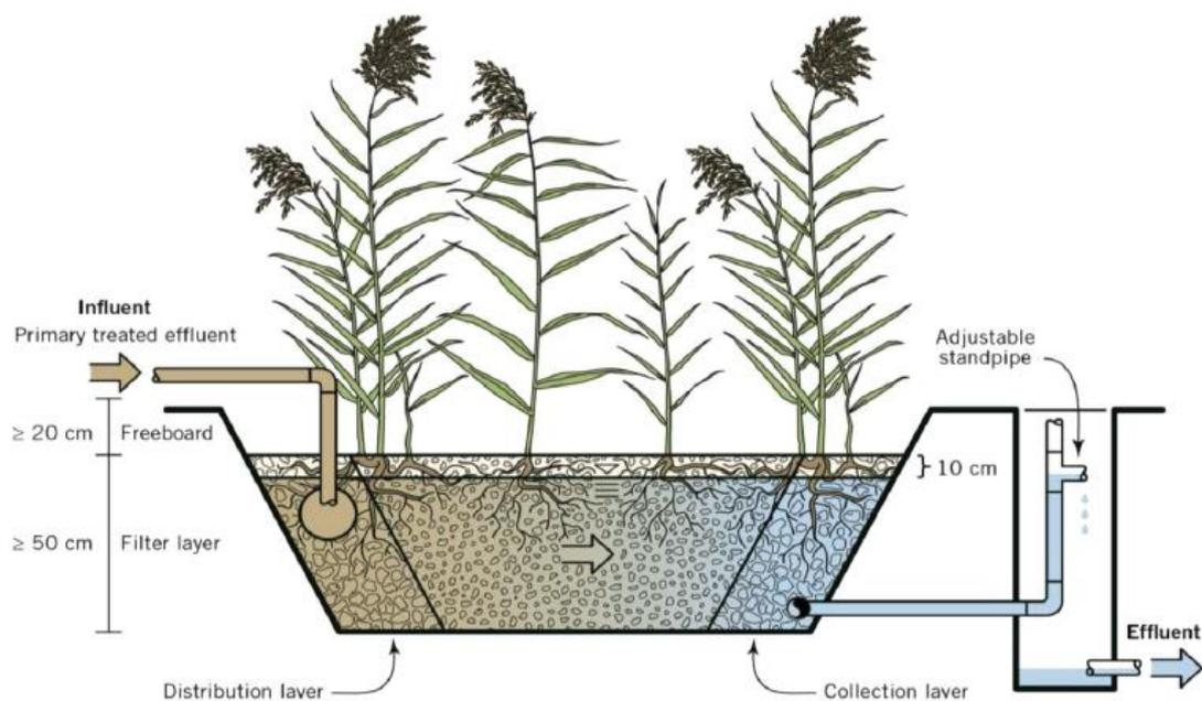
*Fig 3.2 Schematic representation a typical horizontal subsurface flow*
