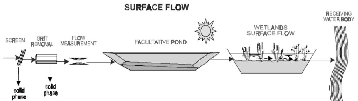
Fig. 2.3 Scheme of a typical Surface flow Wetlands
