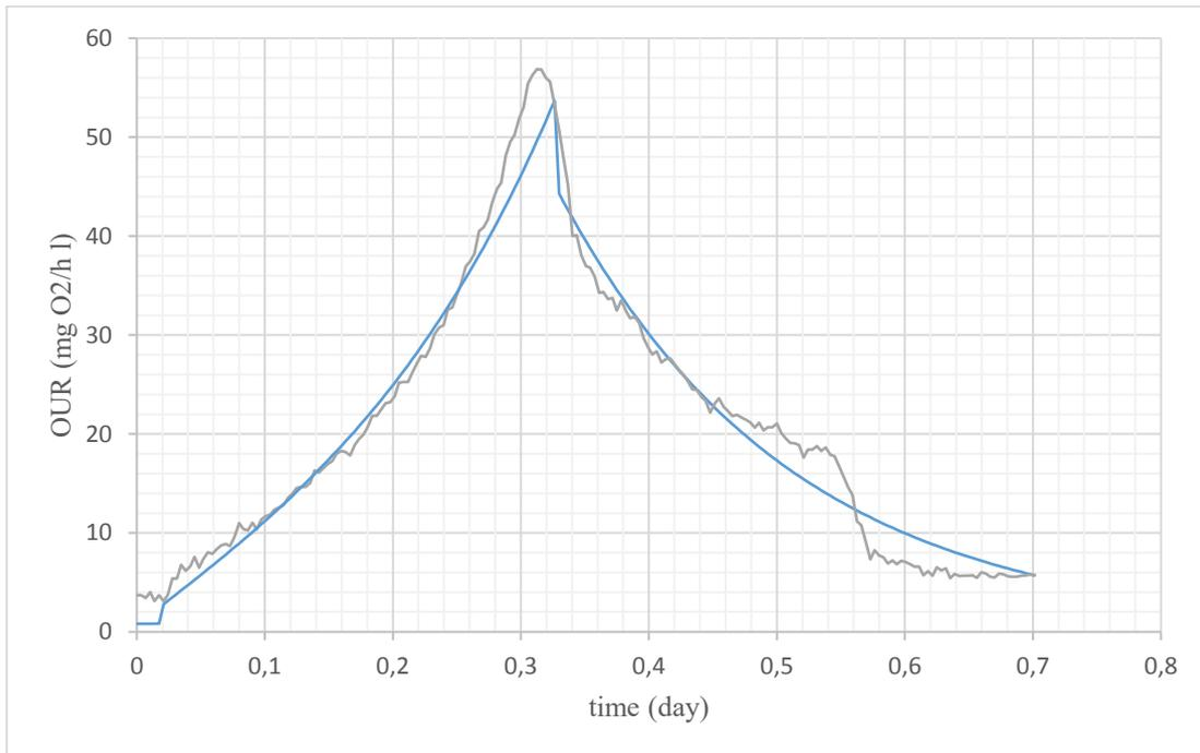
*Fig. 7.3 Observed OUR (grey line) and Simulated OUR with Calibrated Parameters (blue line) – Input Acetate 143 mgCOD/l*
