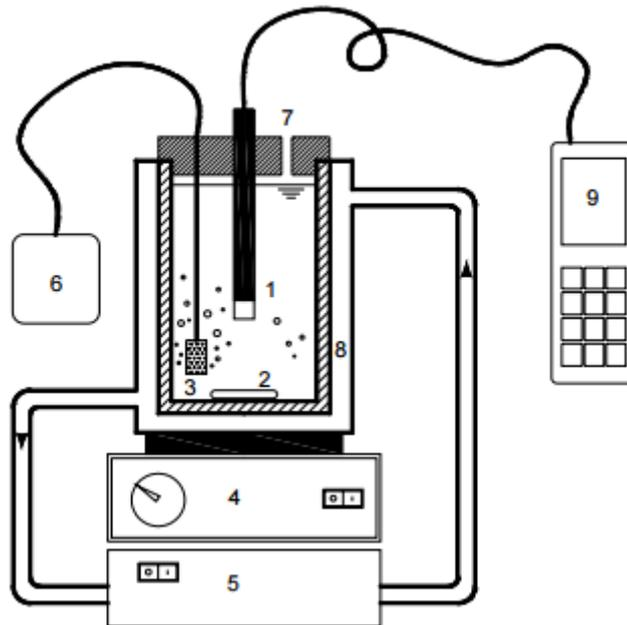
*Fig. 4.3 Respirometric Tests System*
