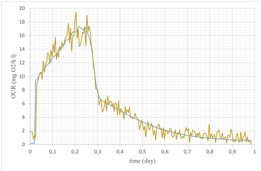
*Fig. 7.7 Observed OUR (brown line) and Simulated OUR with Calibrated Parameters (blue line) – Input Acetate 54.703 mgCOD/l*
