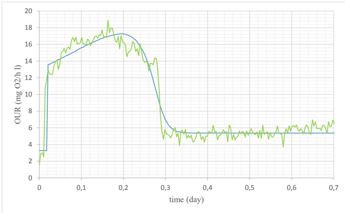
*Fig. 7.6 Observed OUR (brown line) and Simulated OUR with Calibrated Parameters (blue line) – Input Acetate 285 mgCOD/l*
