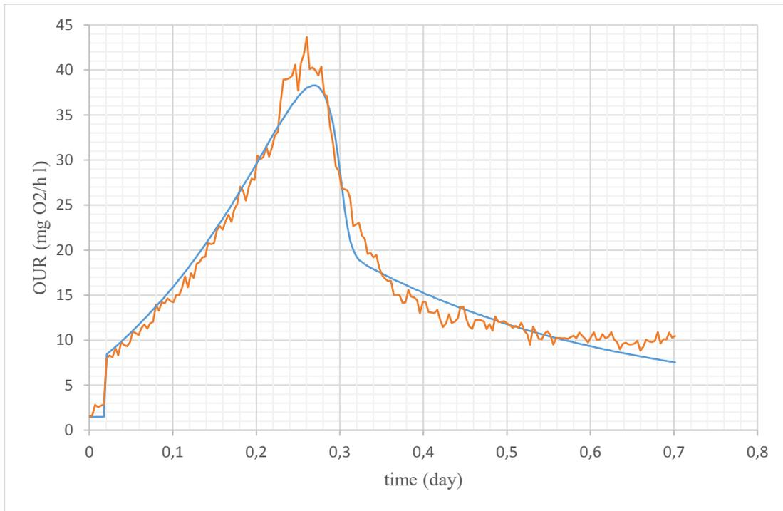
*Fig. 7.2 Observed OUR (brown line) and Simulated OUR with Calibrated Parameters (blue line) – Input Acetate 149 mgCOD/l*
