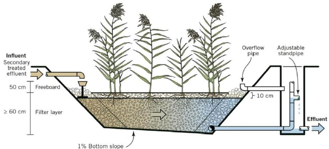
*Fig. 3.3 Schematic representation of HSSF Wetland in tertiary treatment of domestic wastewater*
