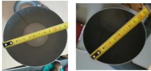
Figure 4.13: Two used cylinders with diameter of: 10 cm and 12 cm
