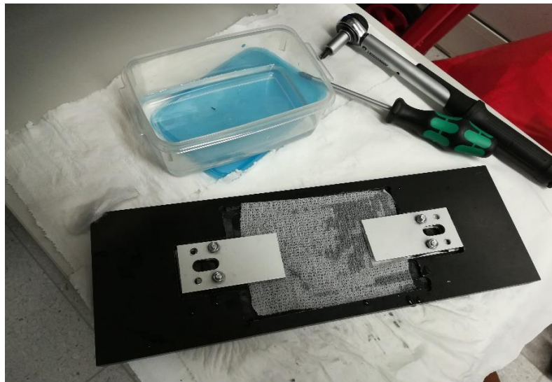
Figure 2.5: Workstation for the Grab test. There are: the box with the distilled water, the PVC support with the sample and the clamps
