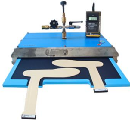
Figure 4.4: Trublu calibration device 64
