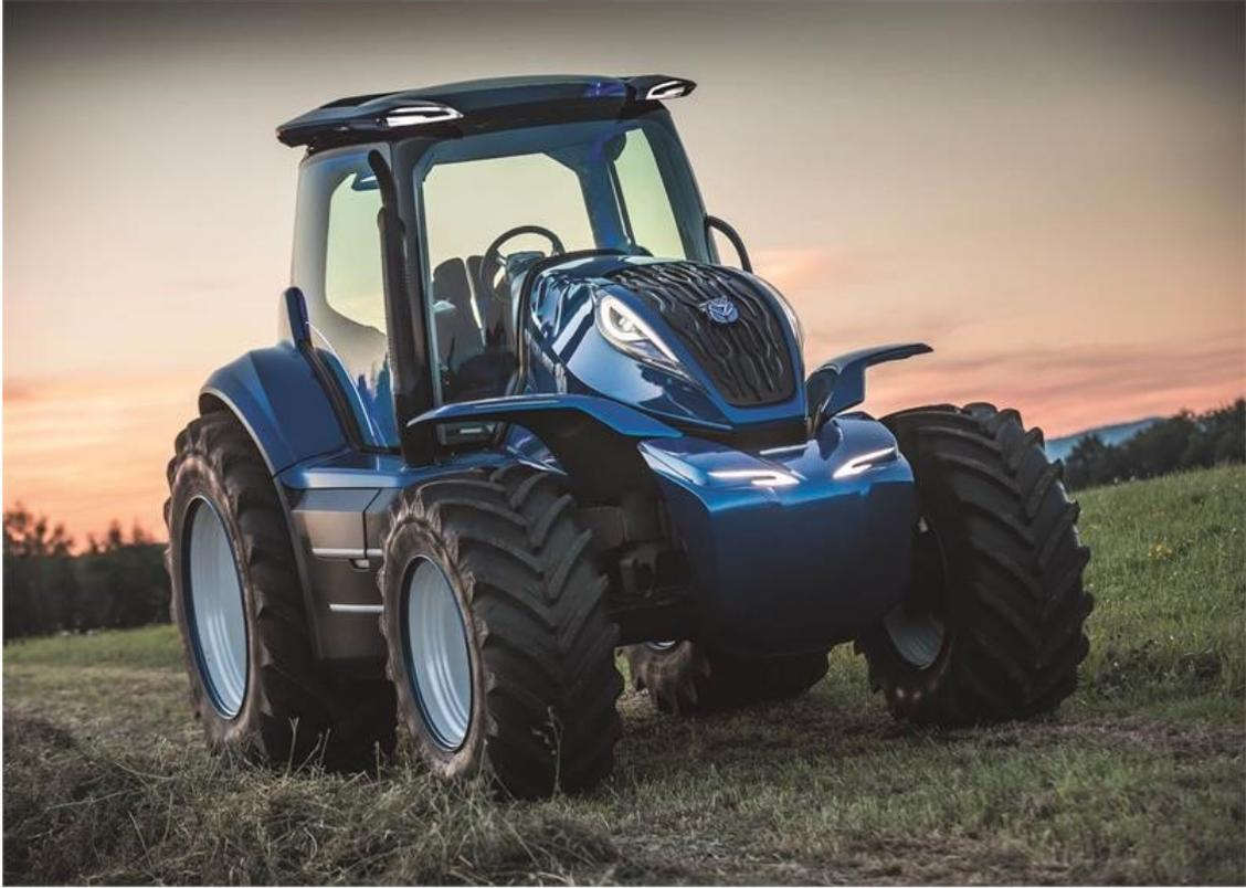
**Figure 1.3:** Tactor equipped with NEF67 CNG engine
