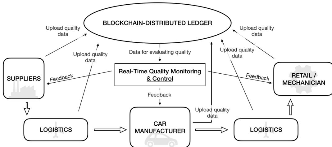
Figure 6.4. Real-Time Quality Monitoring and Control Framework
