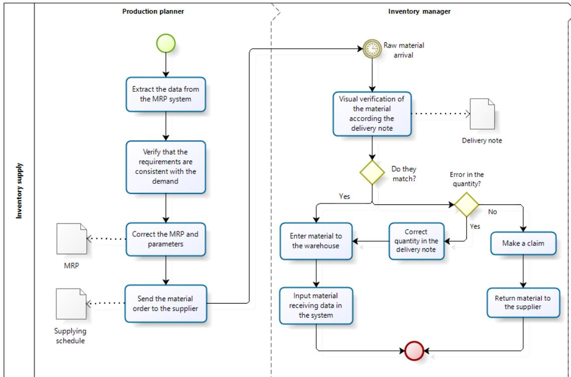
Figure 4.2 Flow chart of the inventory replenishment process
