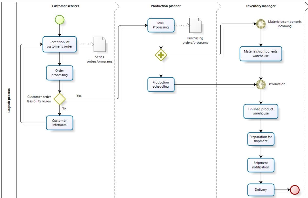
Figure 3.1 Flow chart of logistics process
