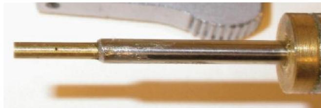
*Figure 3.13 - FRAPP probe, L. Toni et all [4]*
