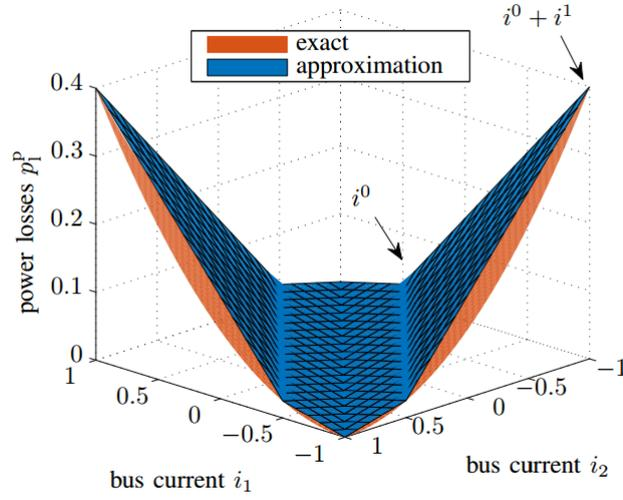
Figure 4.1: Example of the loss approximation in a line between two buses [36].
