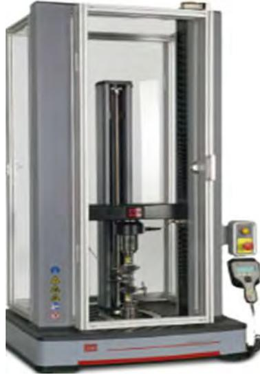
Figure 3.10: MTS Criterion Model 43 tensile testing machine (courtesy of MTS)
