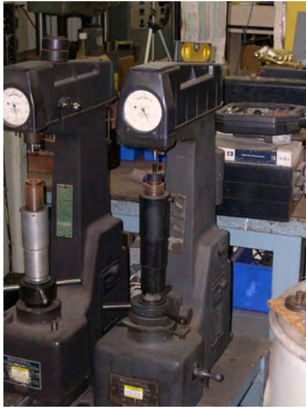
(a) Wilson 4JR Rockwell hardness testing machine
