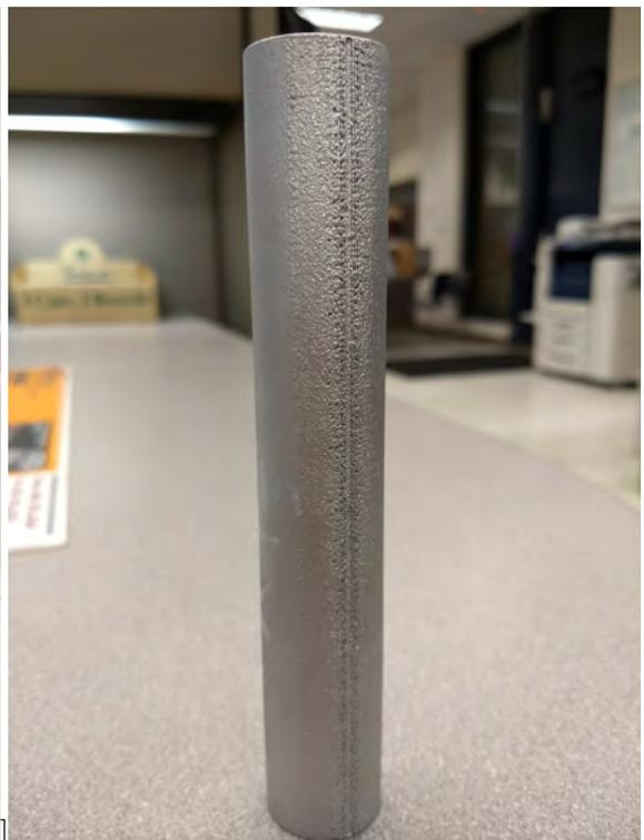
(b) Evidence of build supports on XY-plane rod
