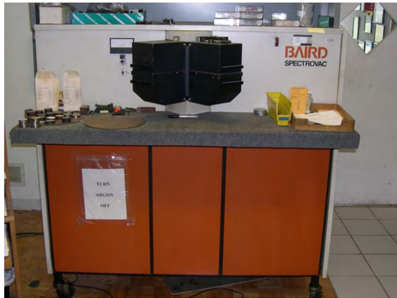
Figure 3.13: Baird Spectrovac DV-3 setup
