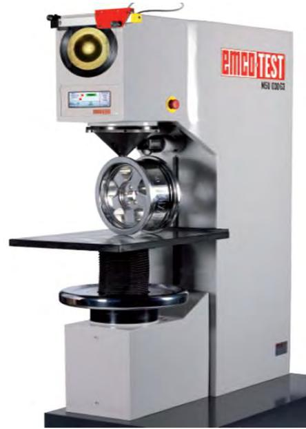
(b) EMCOTEST M5U 300/030 Brinell hardness testing machine
