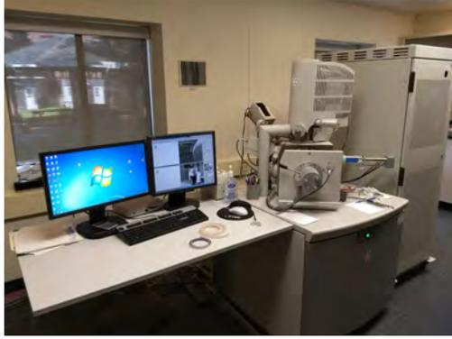
(a) SEM machine with post processing hardware
