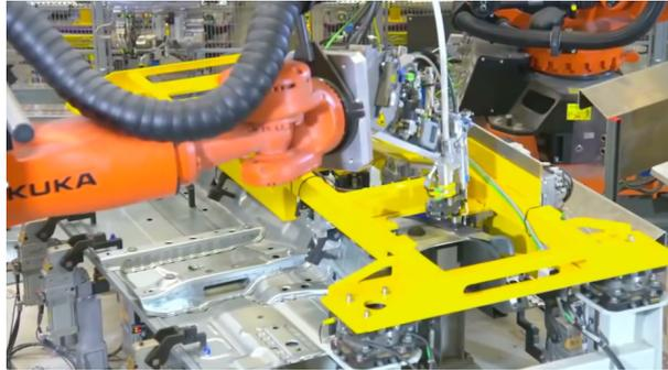
Figure 2.4: *Fully-automated blind rivets installation between the CFRP central tunnel and the aluminum platform (source: BMW)*
