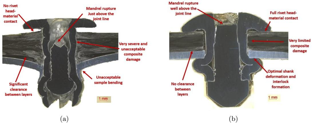
Figure 7.12: Macrography results comparison (2.7 CFRP - 1 mm A6016): a) supplier A sample b) supplier B sample
