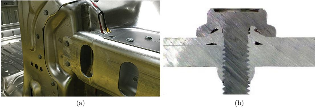
Figure 1.3: *a) Friction- drilling screws in Ford F-150 body assembly (courtesy Weber Screwdriving Systems Inc.) b) Friction drilling screw section and head undercut function (source: EJOT)*
