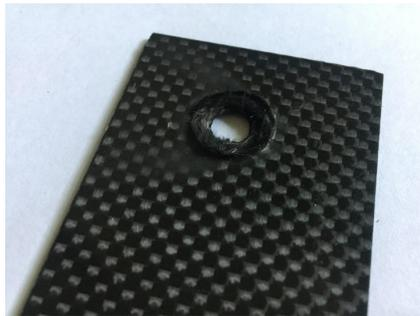
Figure 4.16: *1.6 mm CFRP - 3.1 mm A6061 inlet section of the sample after the rivet removal ( $f=150$  mm/s,  $rs$  6500 rpm)*
