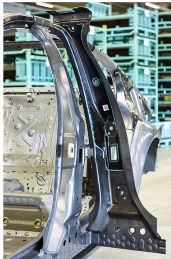
Figure 2.2: *Example of L&L Products customized epoxy film adhesive for BMW [11]*
