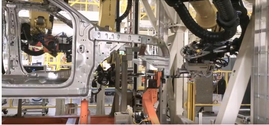
Figure 2.9: *F-150 line: the aluminum body is assembled by means of self-piercing rivets (Photo by Austin Weber)*
