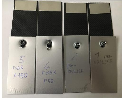
Figure 4.27: Comparison between failed samples joined by means of FSBR (4 and 5) and reference samples (1 and 2)
