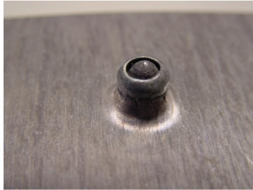
Figure 3.27: *Material sleeve resulting from the riveting process of aluminum (2 mm) to magnesium (2 mm) [44]*
