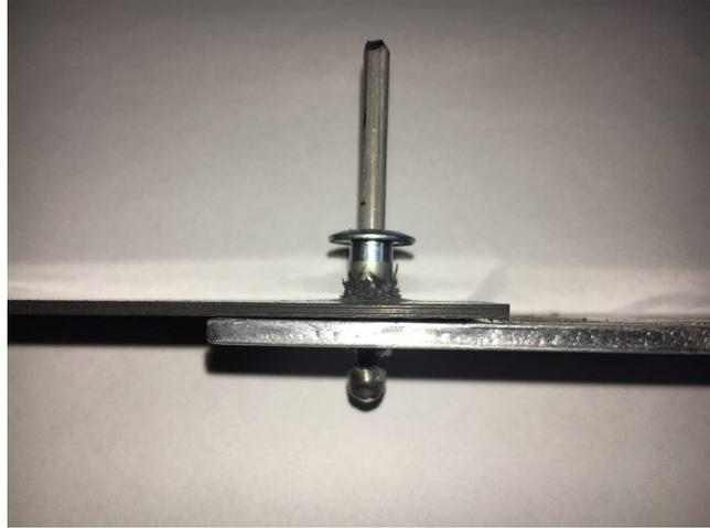
Figure 4.18: *Maximum achieved penetration depth for a 1.6 mm CFRP - 3.1 mm A6061 riveted sample characterized by a quality problem ( $f=150$  mm/s,  $rs$  8500 rpm)*
