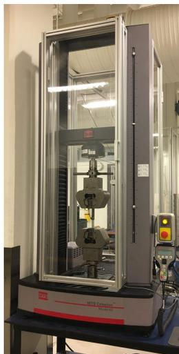
Figure 4.20: *MTS Criterion model 43 tensile testing machine*
