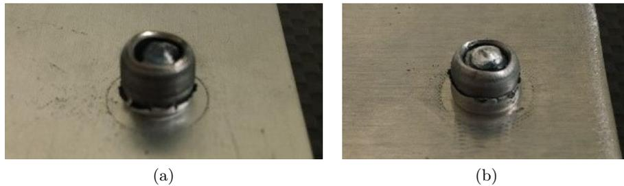
Figure 4.10: *Comparison of formed material sleeves on the connection blind side: a) 1.6 mm CFRP - 1 mm Al b) 0.8 mm CFRP - 3.1 mm Al*
