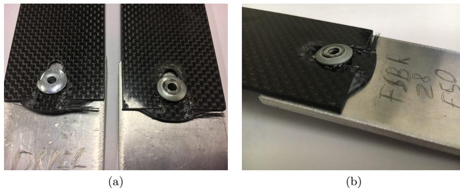
Figure 4.28: a) Composite layer shear out failure in samples joined with standard drilling (left) and FSBR (right) (0.8 mm CFRP-3.1 mm A6061) b) Composite surface damage under the rivet cap due to the fastener stir action (1.6 mm CFRP - 3.1 mm A6061)
