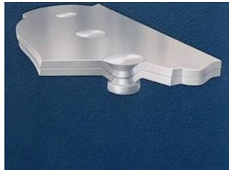
Figure 1.7: *Section of metal sheets joined with flush rivets [7]*
