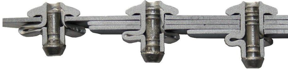
Figure 1.12: Section of Trifold rivets used to join a different number of metal plates
