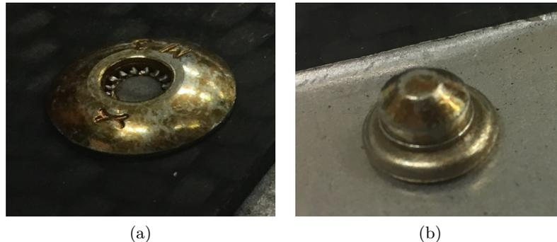
Figure 7.8: *Yellow zinc coating non-homogeneity for supplier B samples*
