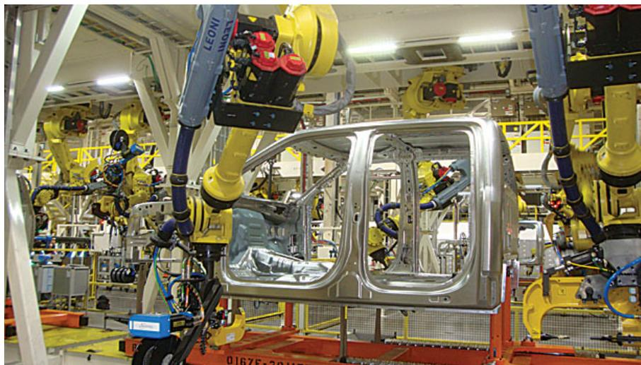
Figure 2.8: *F-150 line: the aluminum body is assembled by means of self-piercing rivets (Photo by Austin Weber)*
