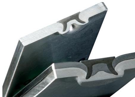
Figure 1.9: *Section of metal sheets joined with self-piercing rivets*
