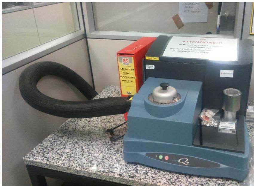
**Figura 5.1:** DSC “TA instruments Q20”
