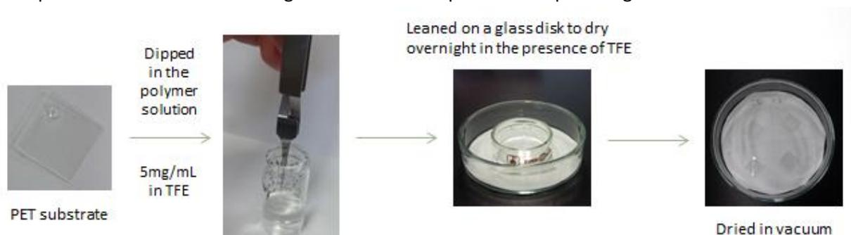
Figure 5.2: dip coating process
