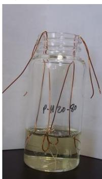
**Figure 5.5: Immersion of coated samples in BSA solution**
