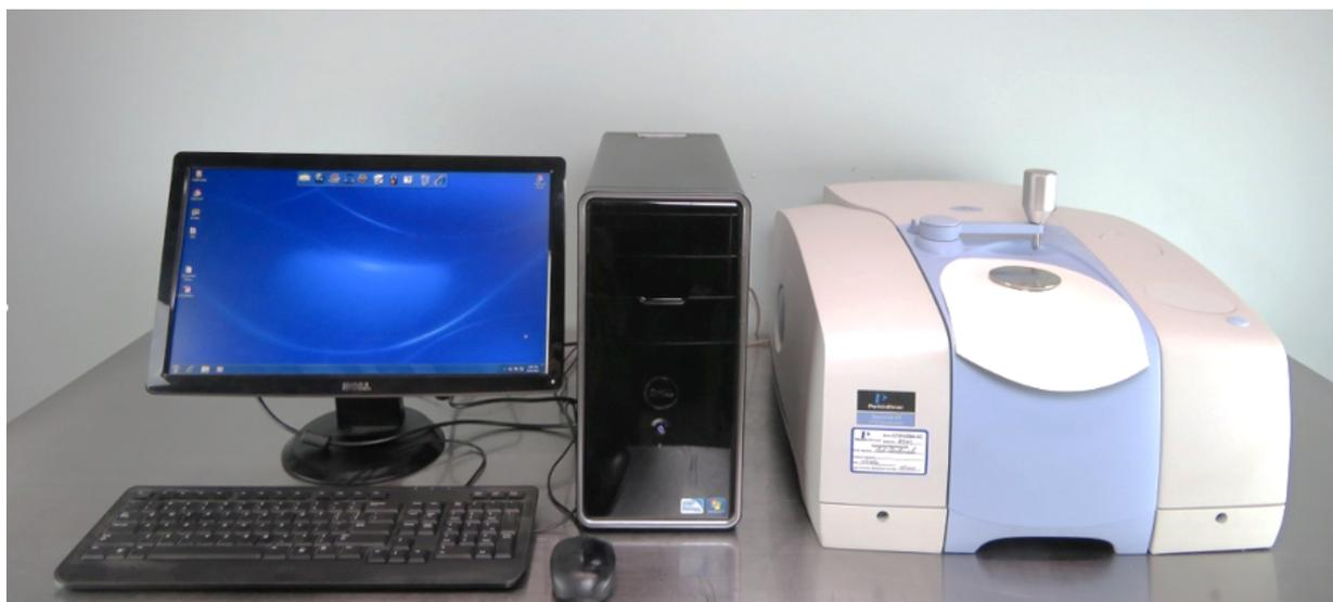
**Figure 3.4:** ATR-FTIR instrumental apparatus.
