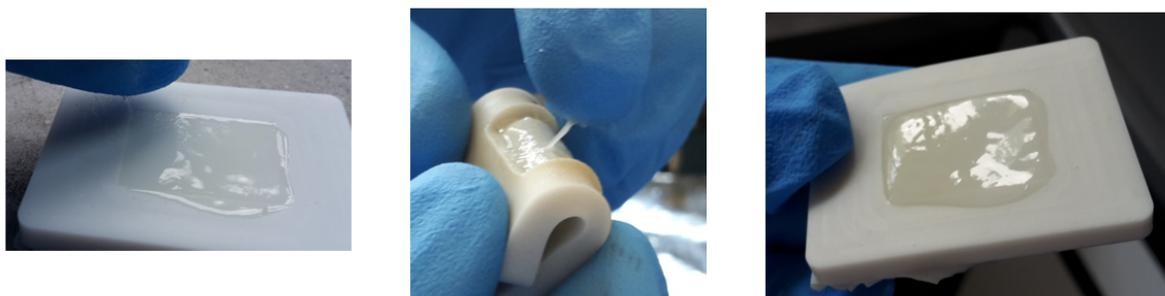
**Figure 2.15:** Examples of photocuring failures induced by the evaporation of the solvent.
