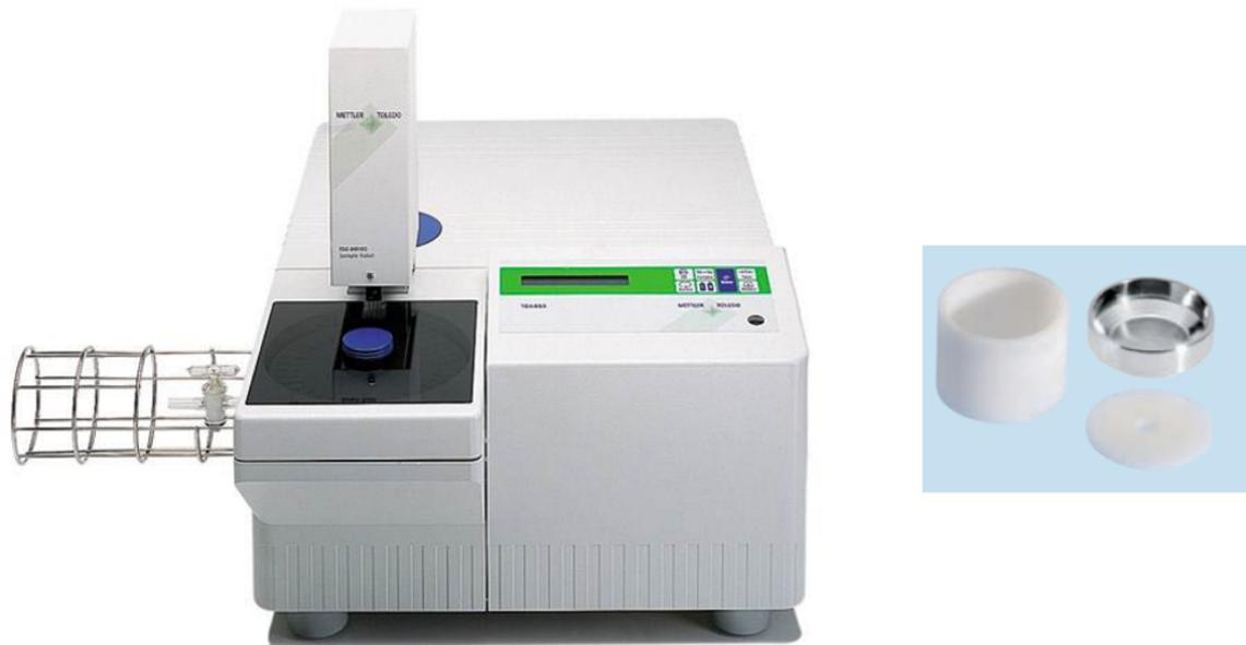
**Figure 3.10:** TGA apparatus and alumina crucible.
