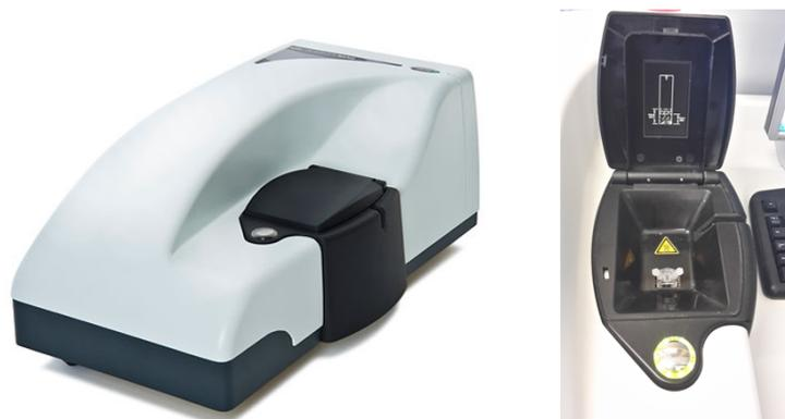
**Figure 3.13:** Z potential instrument [27].
