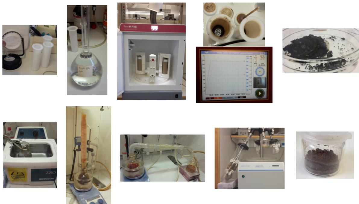
**Figure 2.5:** Experimental procedure followed for the synthesis of nGO.
