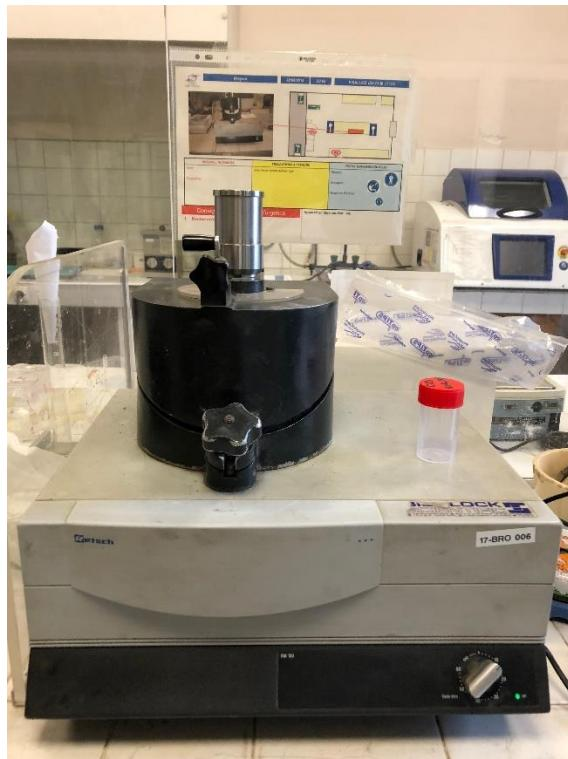
*Figure 4.5 RETSCH (RM100) crusher*
