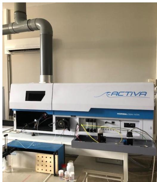
**Figure 4.10** Spectrometer ICP, Activia model from Horiba-Jobin-Yvon
