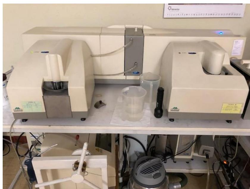
*Figure 4.7 particle size analyzer HYDRO 2000S*
