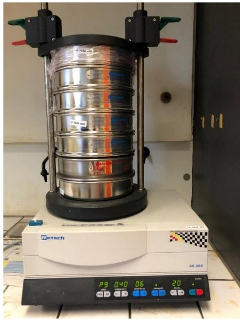
**Figure 4.4** RETSCH sieve shakers (AS200)
