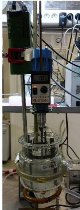
Figure 4.1 - The experimental device consists of the reactor, the rotor and the endoscopic probe.
