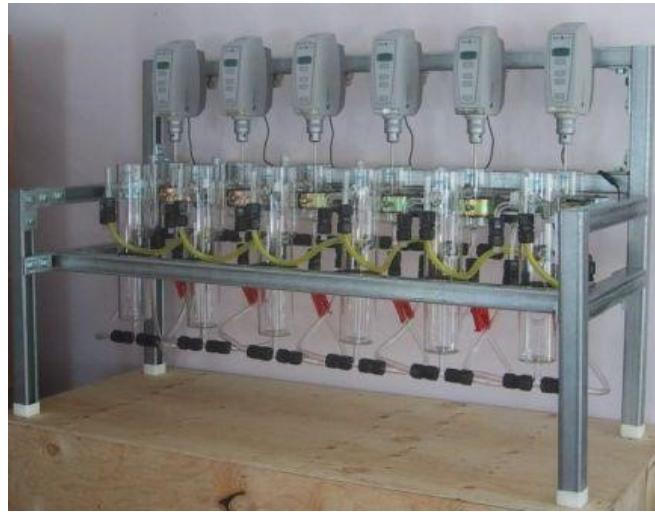
Figure 1.8 - A laboratory-scaled mixer settler [12]
