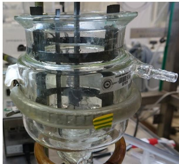
Figure 3.1 - The stirred tank reactor employed for the experiences.
