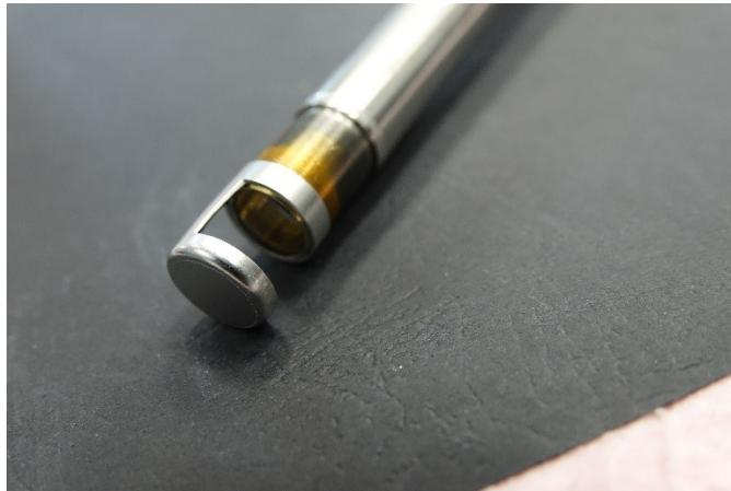
Figure 3.4 - The camera system of the endoscopic probe employed.
