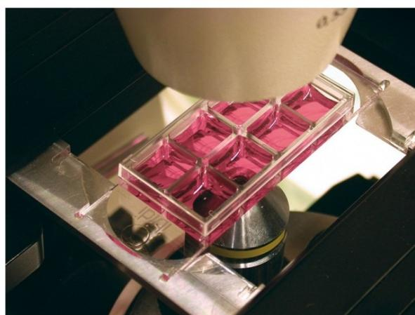
Fig. 3.9 Fluorescence Microscope with 8-well slides for live-cell imaging experiments [16]
