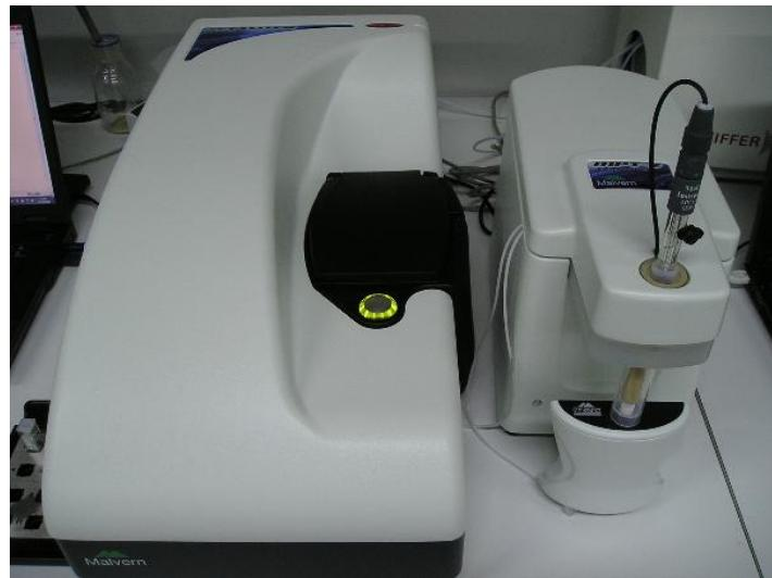
Fig. 3.5 DLS Experimental Apparatus with the automatic titration set-up [7]
