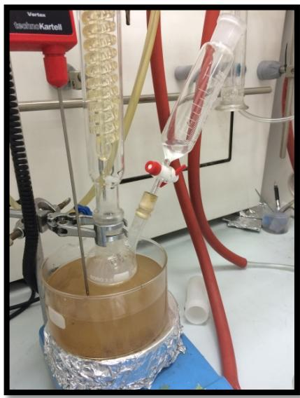
Fig. 3.1 Experimental apparatus for the sol-gel synthesis
