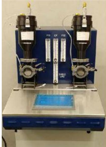
**Figure 2.4:** Powder feeder Optomec
