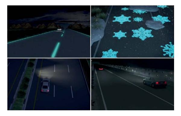
The Smart Highway adabts itself to the traffic, environment and people. By using photo-luminescent paint to mark out traffic lanes, there would be glow-in-the-dark road because the paint absorbs energy from sunlight during the day and release it after sunset so it can light the road during the night for up to 10 hours.
