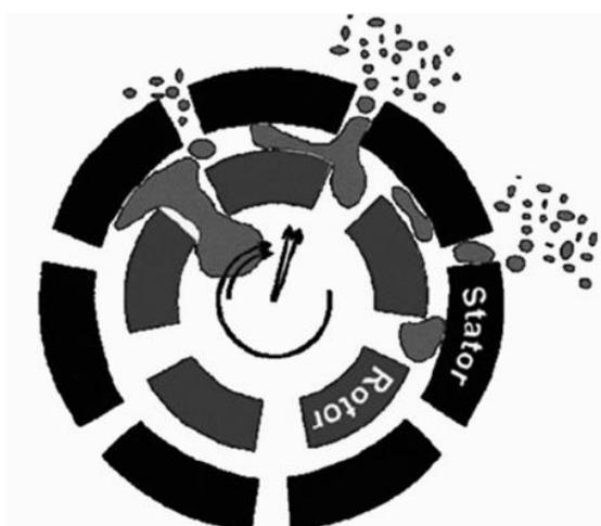
**Figure 1.12:** Rotor-stator shear by spinning shaft, inside view [25].
