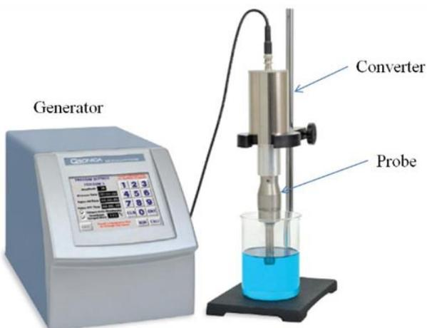
**Figure 1.14:** Ultrasonic equipment [27].
