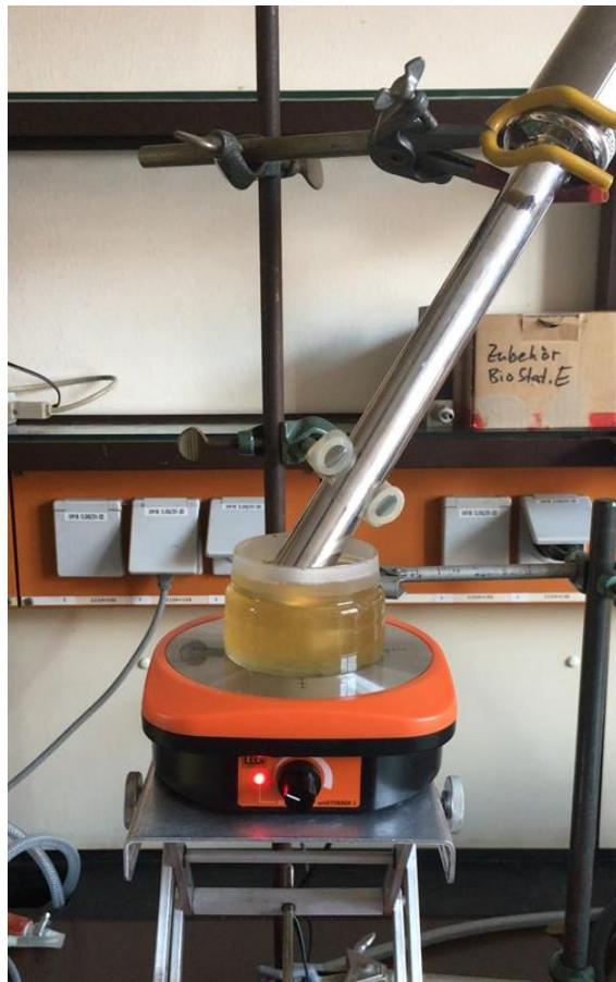
**Figure 5.3:** Picture of the experimental set-up for *in-situ* laser back-reflection measurements.
