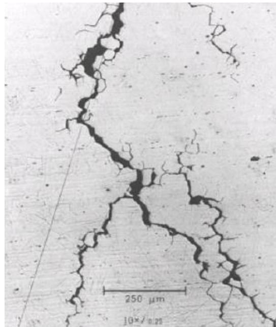
*Figure 10 Example of SCC of a ZTA in an inox steel which is inclined to it because of nitrogen*
