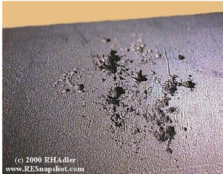
*Figure 8 Example of pit corrosion*
