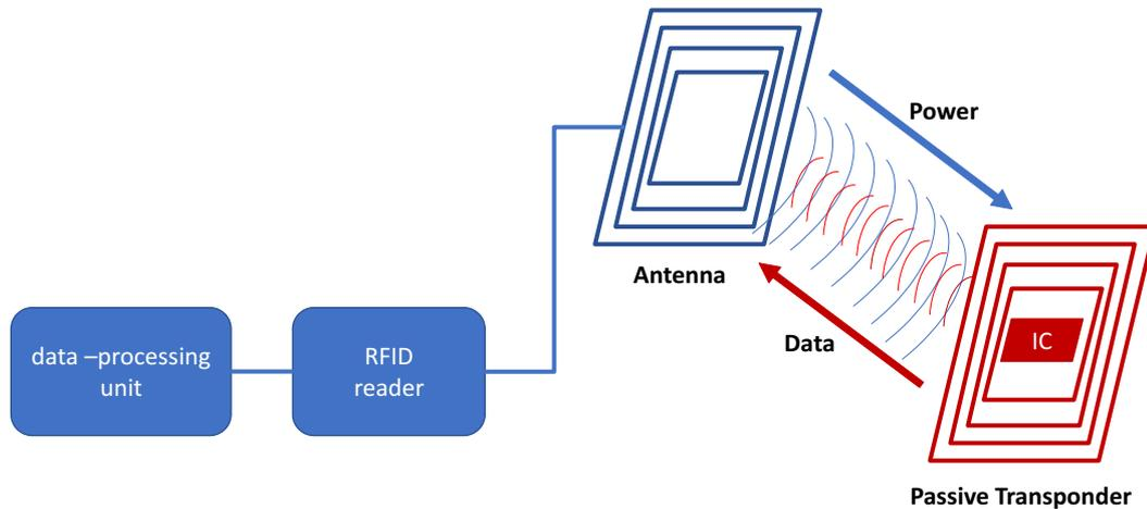
Figure 2.3: RFID technology with passive tag, overview. The RFID reader is powered by the data-processing unit and powers the passive tag sending energy through an antenna. The coiled antenna on the tag receives the energy and powers the chip (IC). The chip sends back radio-frequency wave through the antenna that is then read by the reader and processed by the data-processing unit.
