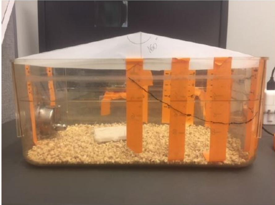
Figure 3.3: Picture of the cage showing the problem relative to the field of view of the camera. The white paper shows that a FOV of  $160^\circ$  is required to cover the whole area of the cage, walls included. The black marker line shows the hidden area in case of employment of a traditional camera.
