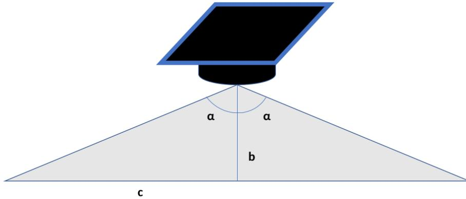
Figure 3.2: Support image to viewing angle problem. The black module indicates the camera. Since  $b = 3\text{cm}$  (the additional length due to the lid set on the walls of the cage) and  $c = 14.25\text{cm}$ , the minimum viewing angle  $2\alpha$  that allows to cover the whole area is  $156^\circ$ . According to this, a camera with  $FOV = 160^\circ$  was employed.
