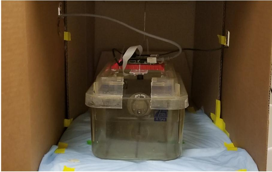
Figure 3.4: Illustration of home cage setup. The picture was taken during an experiment carried out at Johns Hopkins University School of Medicine. On the lid of the cage it is possible to notice the support with the camera module and the raspberry Pi. The whole cage is placed inside a paper box to reproduce the darkness of biological laboratories.
