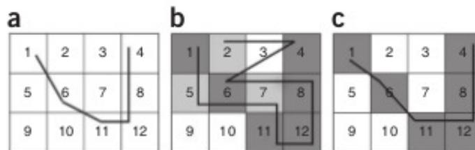
Figure 2.4: RFID system tested on arena with 12 antennas with one mouse moving. Picture was taken from Luca Catarinucci et al. paper [5]. (a) Real mouse path across the arena. (b) Reconstructed path based on raw data. Dark cells refer to ones rightly included in mouse’s path. Light-shaded cells refers to ones mistakenly included in mouse’s path. (c) Reconstructed path after data processing. Dark cells correspond to ones rightly included in mouse path.
