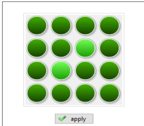
Figure 3.15: LED matrix created in LabVIEW® to let the user choose the electrodes for conducting the impedance measurements directly from LabVIEW® graphical user interface.
