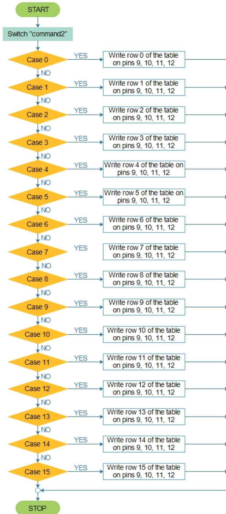
Figure 3.20: Flowchart of the "switch case" executed for the conversion of the second number read from the string (BLOCK 2).
