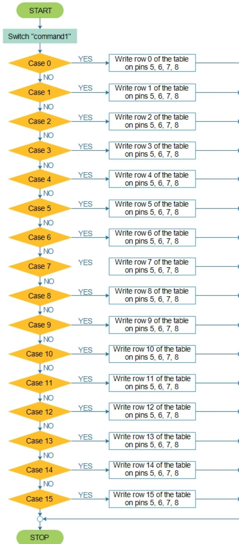
Figure 3.19: Flowchart of the "switch case" instruction executed for the conversion of the first number read from the string (BLOCK 1).
