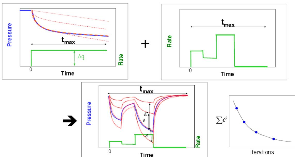
Figure 9: Deconvolution Process through Superposition<sup>[12]</sup>
