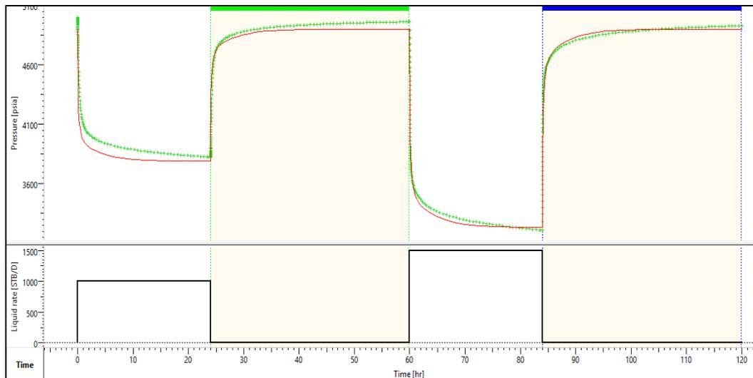
Figure 58: History plot showing the mismatch of the actual pressure data and deconvolved response after the deconvolution on all extracted periods (build-ups)
