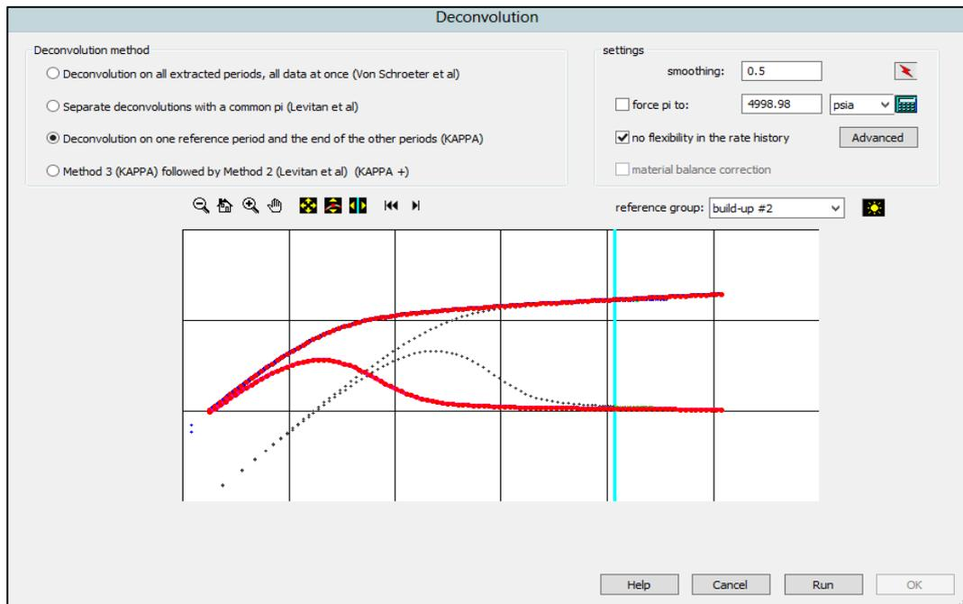
*Figure 59: Deconvolution option on Saphir showing the usage of the third deconvolution choice and the light blue line to locate the end of the both build-up periods, where the properties are the same*
