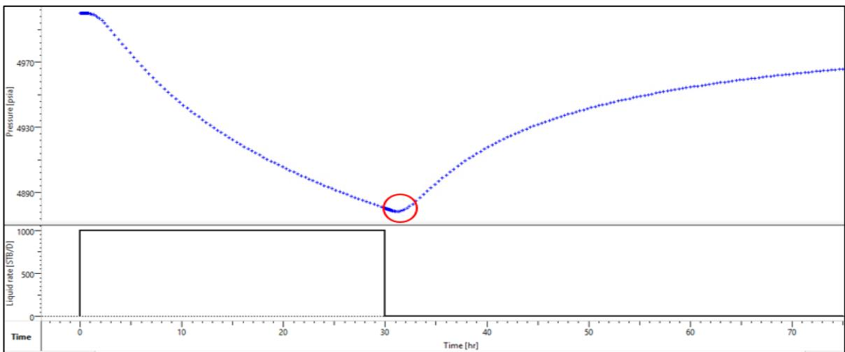
Figure 68: Pressure change with respect to time of the observational well with a time delay due to interference from an active well
