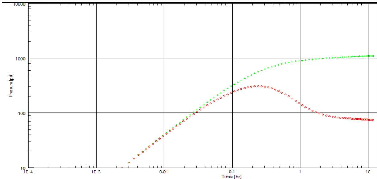
Figure 47: Log-log plot for the gap case showing normal and derivative pressure curves for the build-up phase
