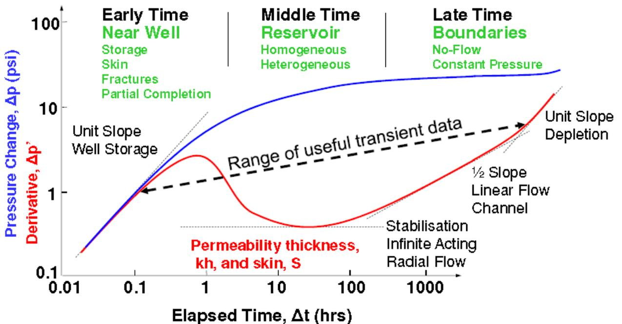
Figure 4: Log-log plot showing normal and derivative pressure curves, in addition to different well test models and different reservoir types<sup>[12]</sup>
