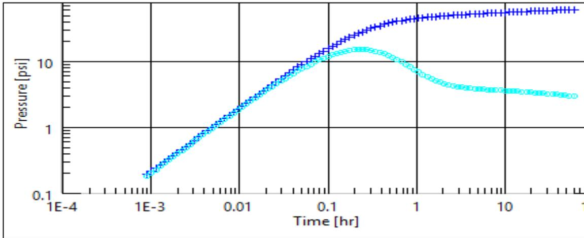
Figure 21: Log-log plot showing the deconvolved response equal to 60 hours
