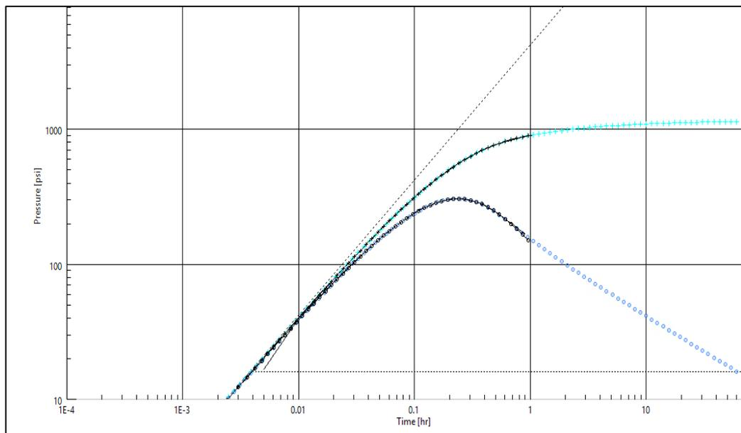
Figure 14: Log-log plot of the deconvolved response, in addition to the original build-up period of 1 hour
