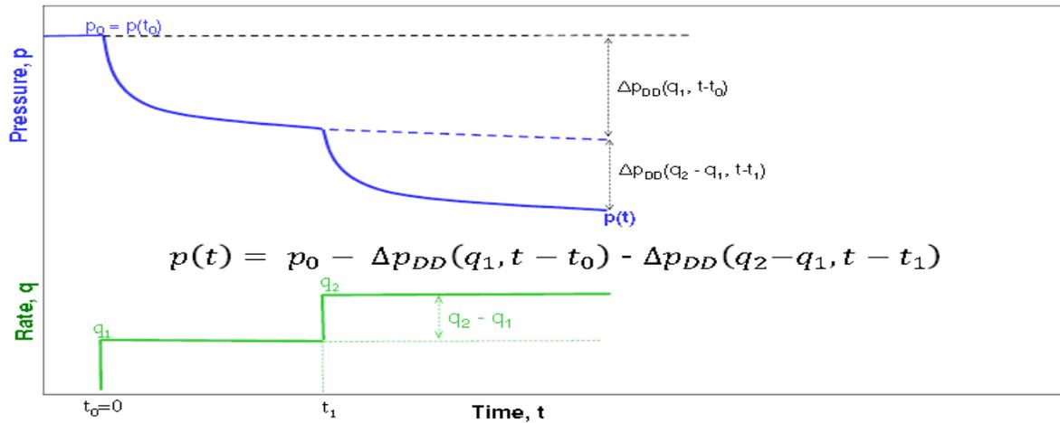
Figure 7: Superposition in Time for two rates<sup>[12]</sup>
