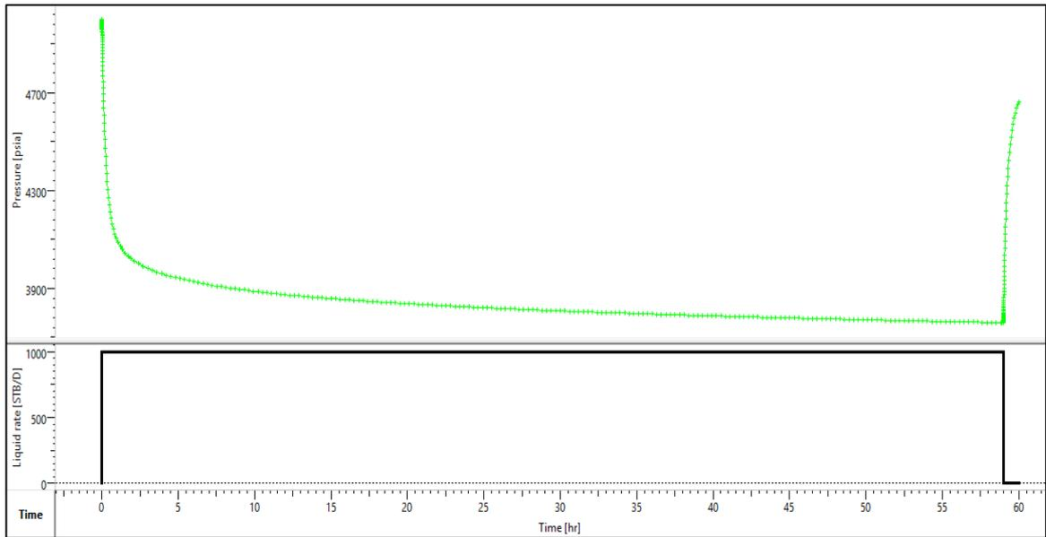
Figure 13: Pressure versus time plot, corresponding to a constant rate of 1000 BOPD for 59 hours, followed by a one hour build-up period
