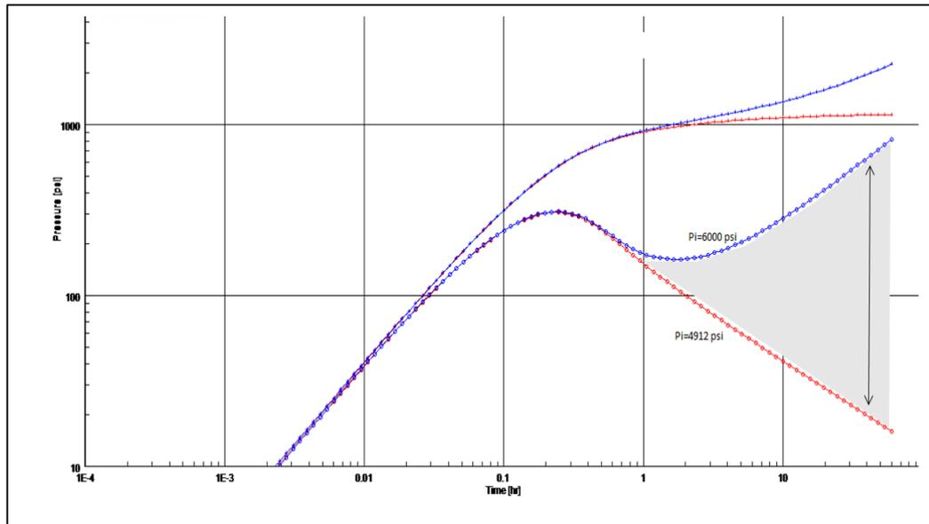
Figure 18: Log-log plot showing deconvolved response on build-up phase, and also showing range of possible shapes in the shaded area corresponding to different initial pressures
