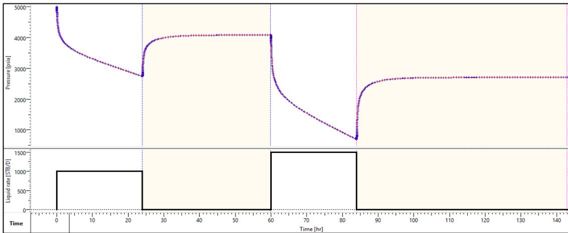
Figure 32: History plot of pressure versus time showing match between deconvolved response and pressure data under PSS
