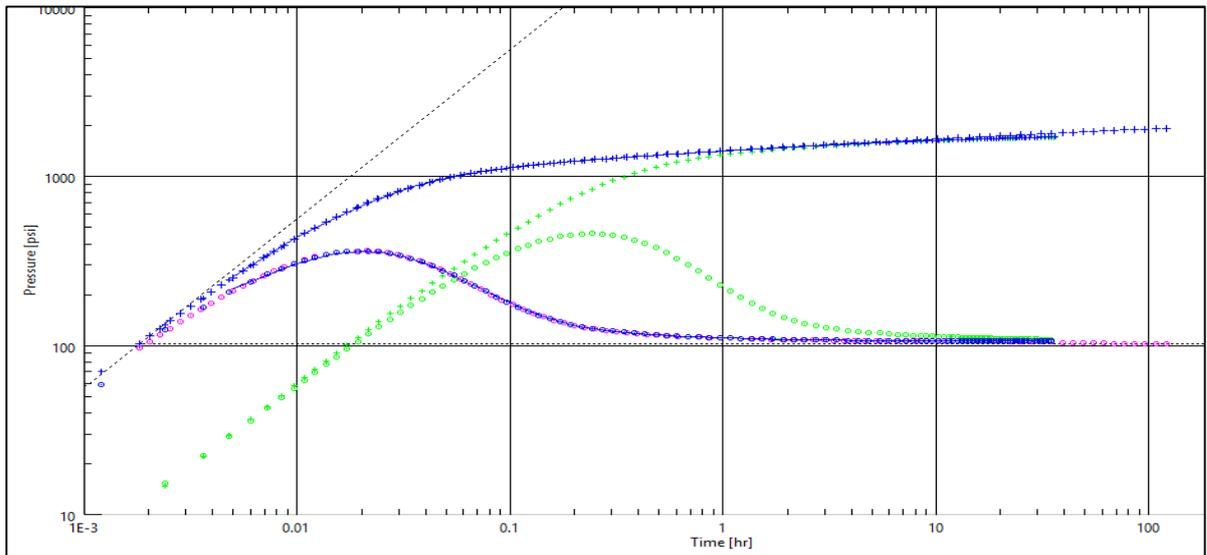
Figure 61: Log-log plot showing the normal and pressure derivatives and the deconvolved response (pink color) for the build up periods
