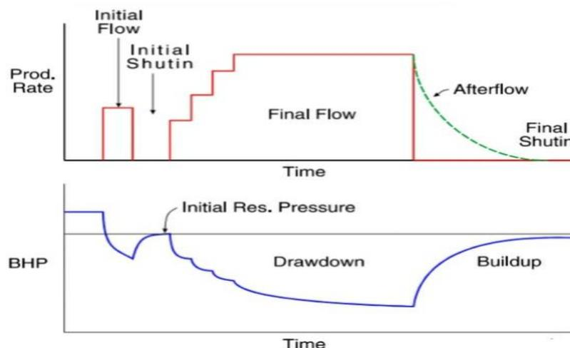
Figure 2: Pressure change with respect to time corresponding to specific rates<sup>[11]</sup>
