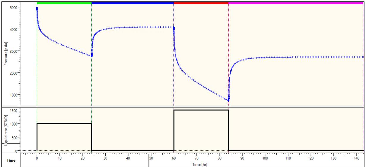
Figure 29: History plot of pressure versus time, with 2 flow periods of 1000 and 1500 BOPD respectively for the rectangular reservoir
