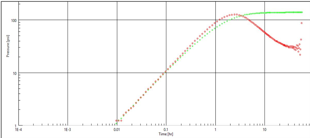
Figure 27: Log-Log plot with a permeability of 5 mD and resolution of 0.04 psi
