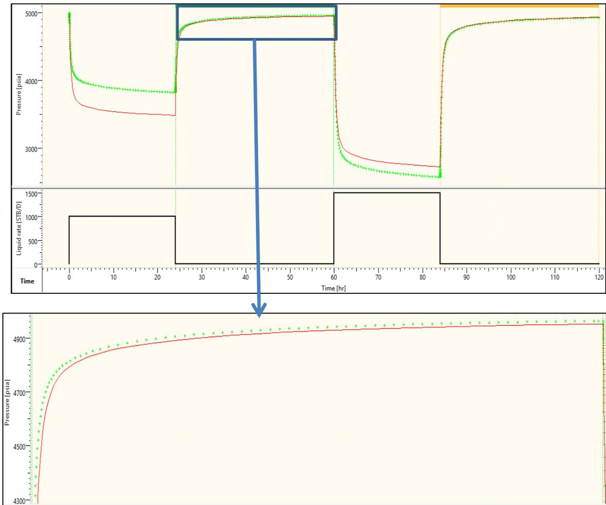
Figure 65: History plot of Pressure versus time showing the mismatch (in a zoomed way) between deconvolved response and actual pressure data for the change in skin case when deconvolution on all extracted periods was used
