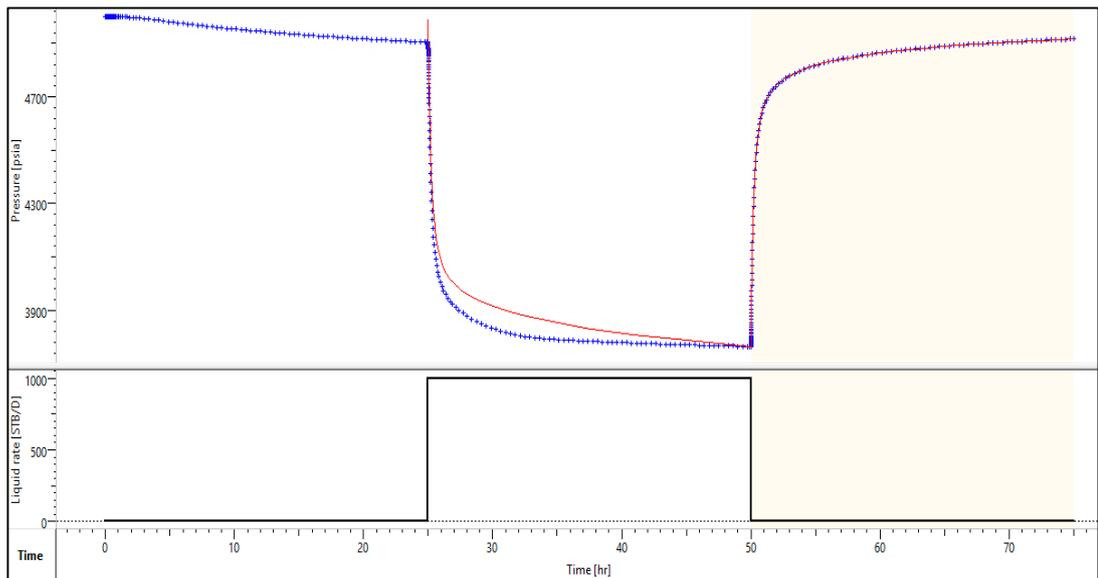
Figure 74: Pressure change versus time for well 1 after the change in test sequence of well 1, corresponding to a specific rate sequence for duration equal to 75 hours
