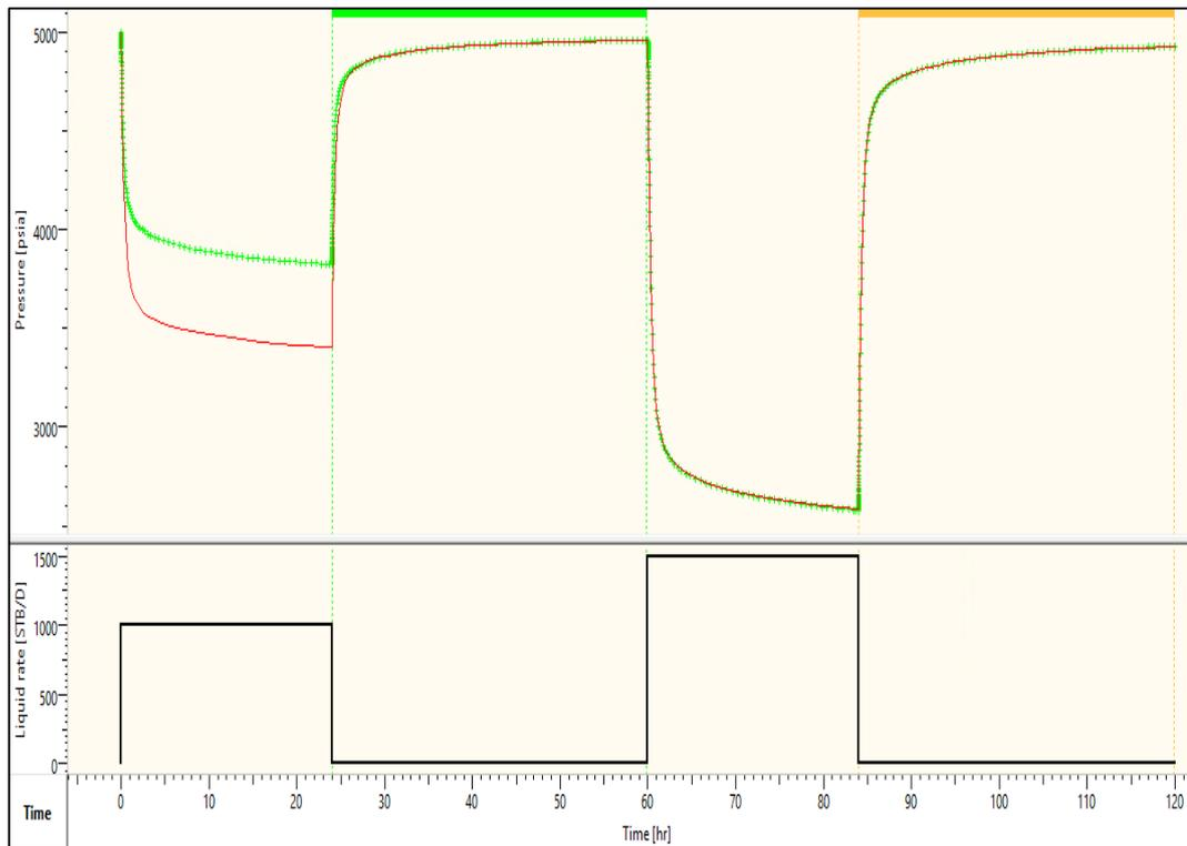
Figure 66: History plot showing deconvolution results and match on the drawdown and build-up periods corresponding to different rates
