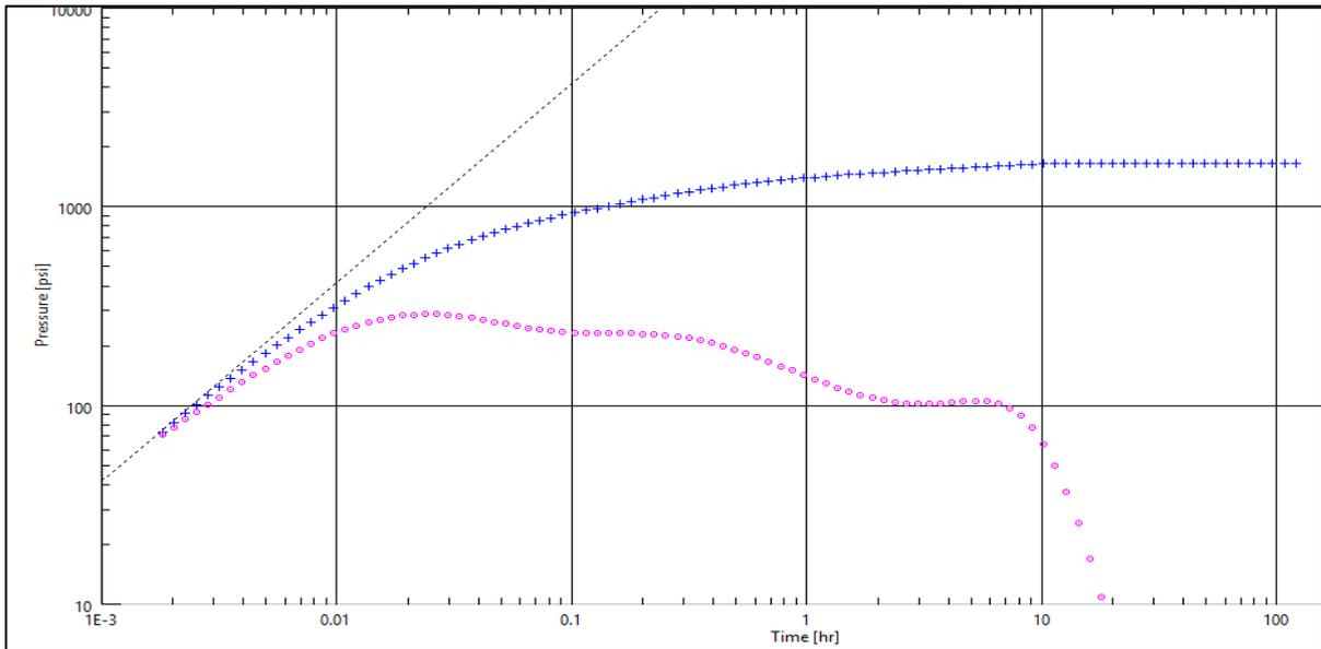
Figure 57: Log-log plot showing the results of the deconvolution extracted on all periods for changing wellbore storage case
