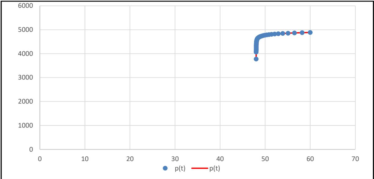
Figure 52: Match between pressure build up (blue) and deconvolved response (red) of the build-up of the Gap case after the modification in Figure 51
