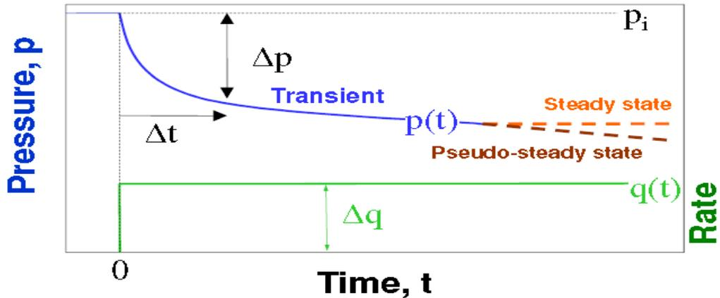
Figure 3: Pressure with respect to time for a certain constant rate with 2 different late time options<sup>[12]</sup>
