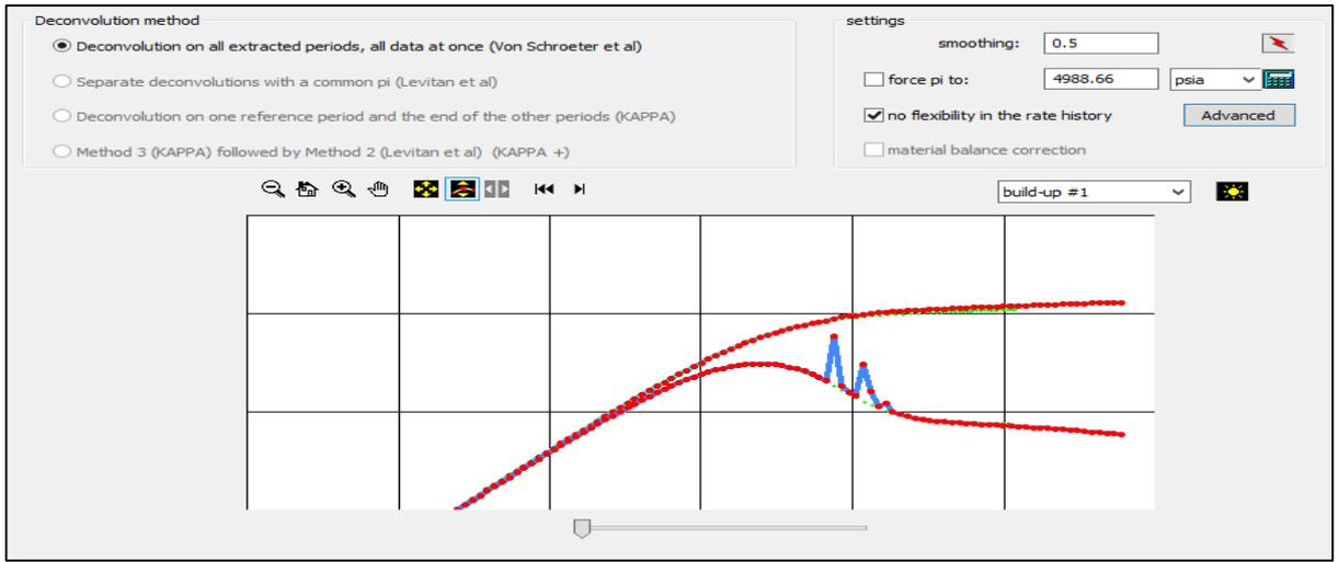
Figure 53: Deconvolution option on Saphir showing the adjustment of the deconvolved response points outside of the gap
