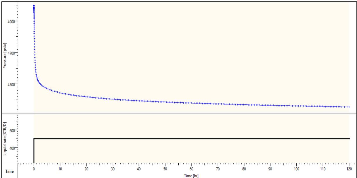
Figure 45: Pressure versus time plot for a constant average rate of 500 BOPD
