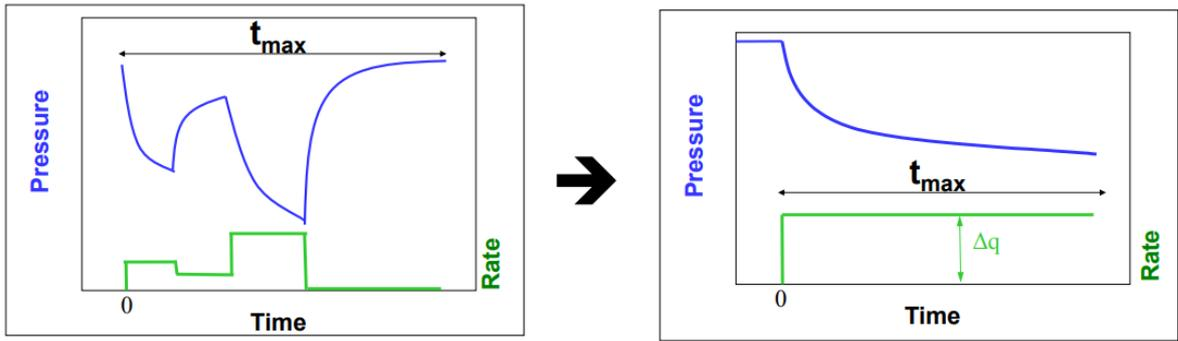
Figure 8: Deconvolution Principle<sup>[12]</sup>
