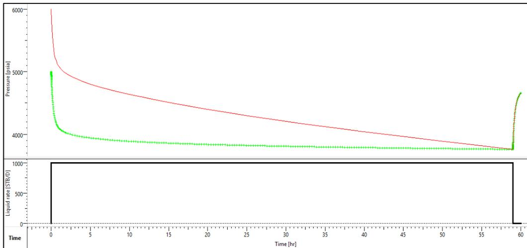
Figure 17: Pressure mismatch between deconvolved response and actual pressure data for  $P_i = 6000$  psi
