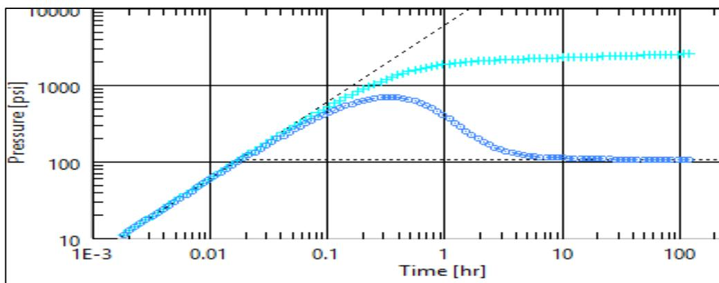
Figure 67: Deconvolution on a log-log plot where the response is equal to the whole duration of the test
