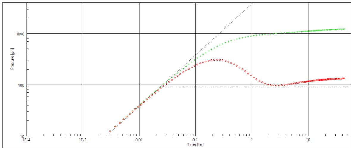
Figure 71: Log-log plot showing the normal pressure change and its derivative for the build-up phase of well 1, being interfered by active well 2
