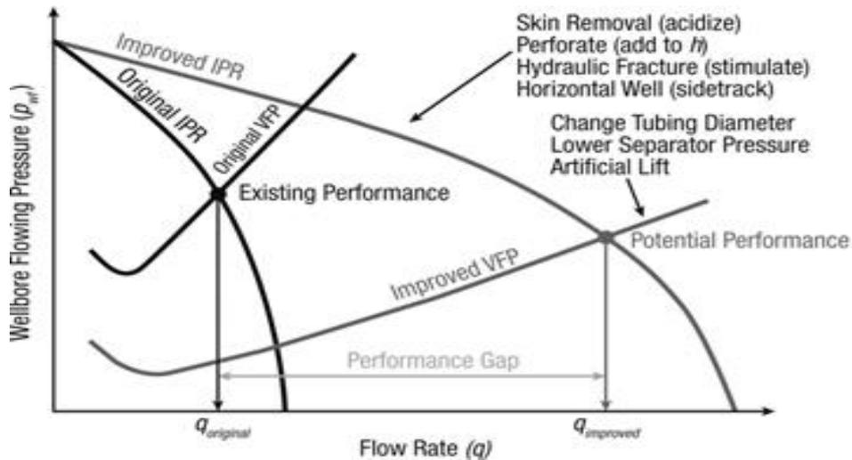
Figure 1: Well Performance showing IPR and VFP<sup>[9]</sup>
