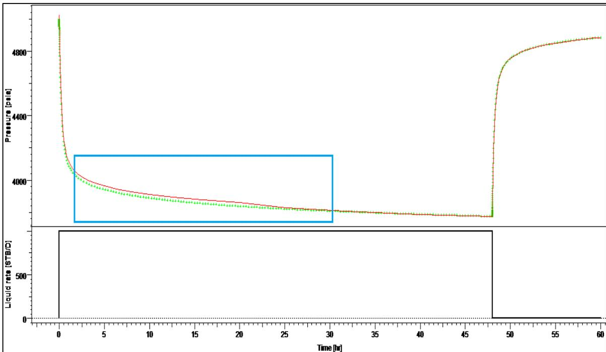
Figure 50: Pressure versus Time plot showing drawdown mismatch and the build-up match between the deconvolved response and actual pressure data
