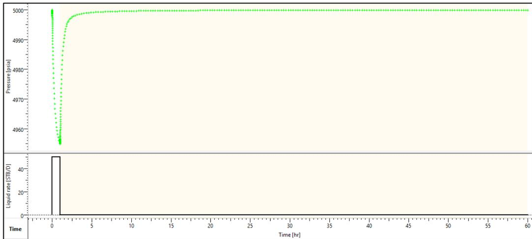
Figure 20: History plot of pressure versus time for the short production long build-up case
