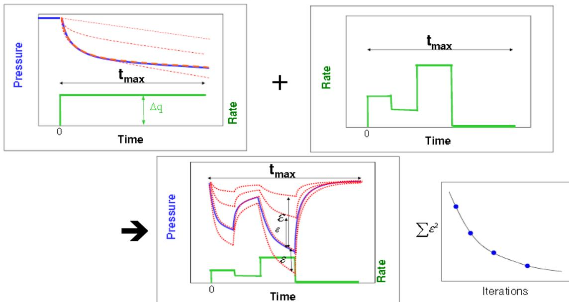
Figure 9: Deconvolution Process through Superposition<sup>[12]</sup>
