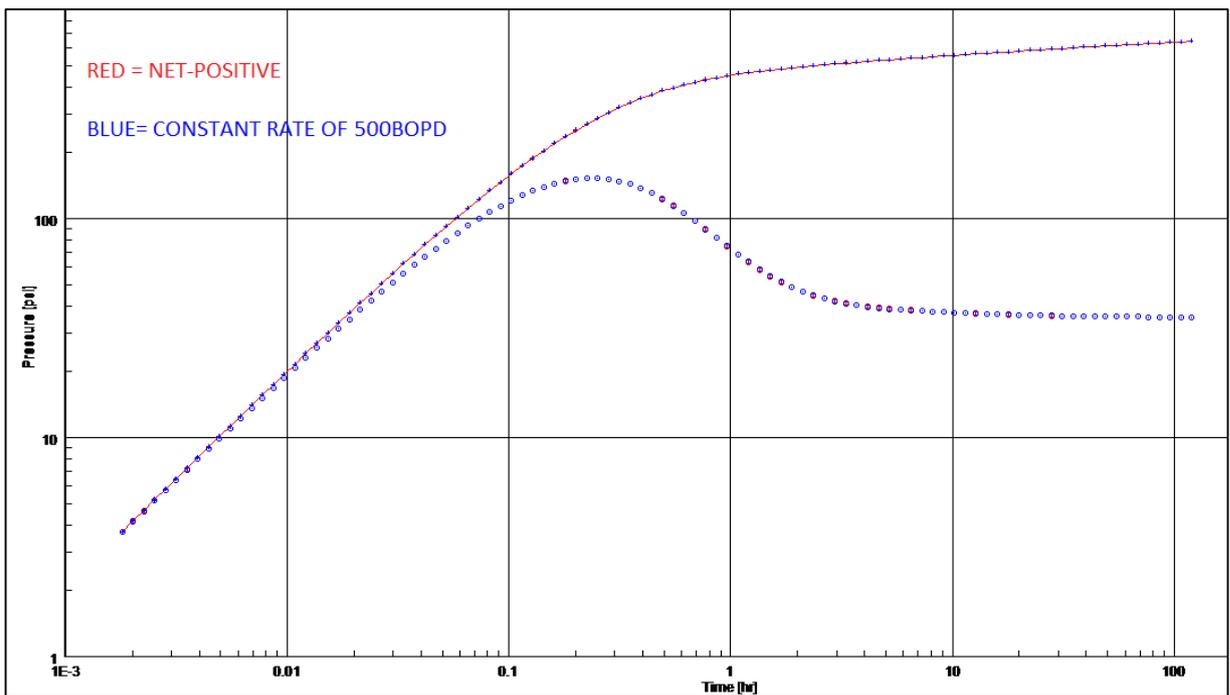
Figure 46: Comparison between net-positive case and constant rate of 500 BOPD on a log-log plot
