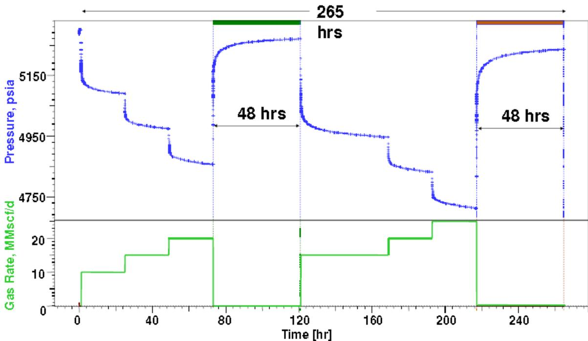
Figure 10: Pressure and Gas Rate versus time example<sup>[12]</sup>
