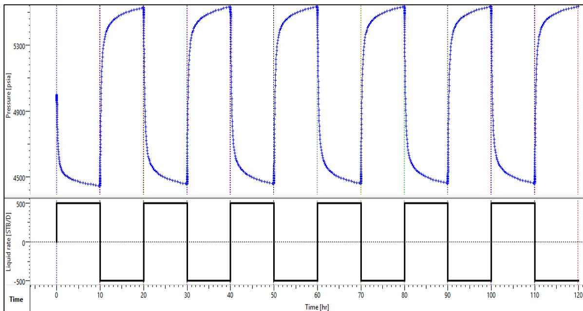
Figure 35: Harmonic pressure signals versus time with a net-zero rate of +500 and -500 BOPD along 120 hours
