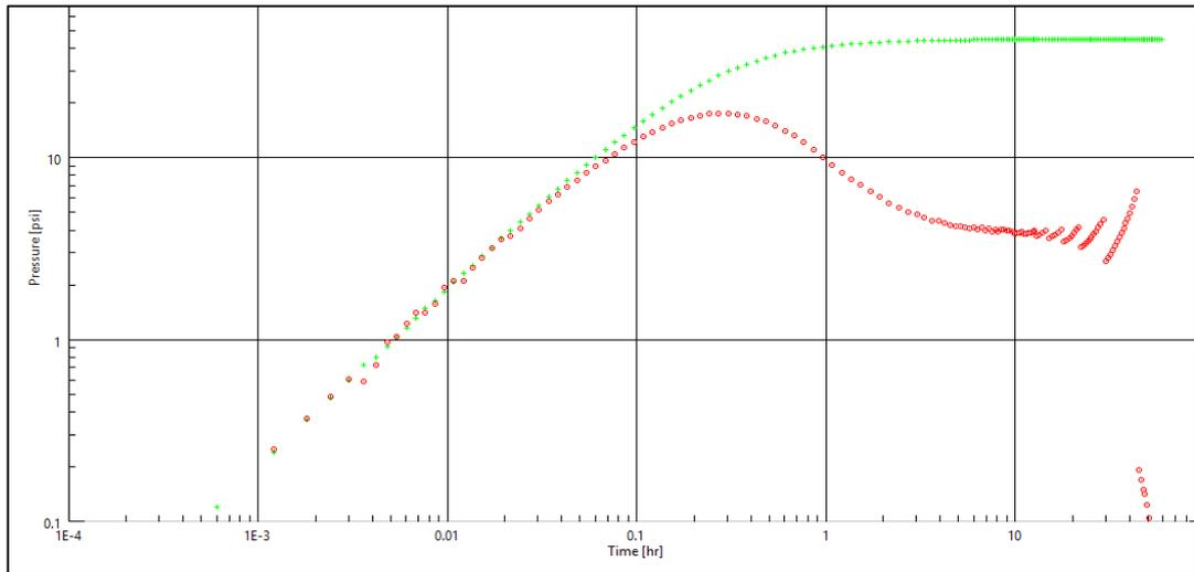
Figure 19: Log-log plot with scattered data of normal and derivative pressure curves with a resolution of 0.04 psi for the build-up phase
