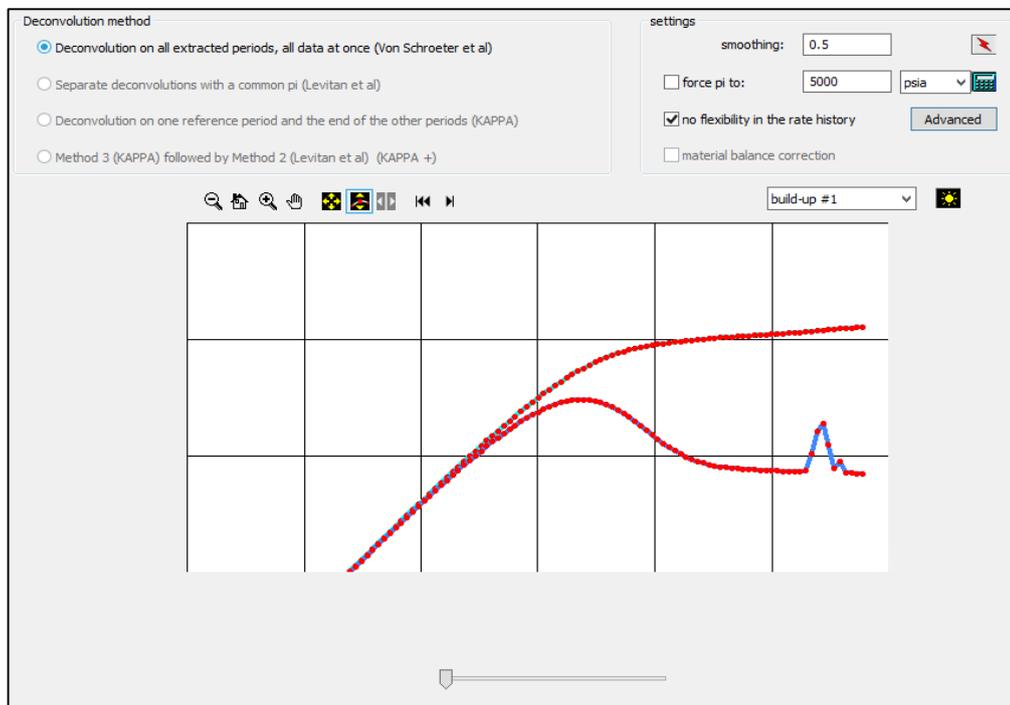
Figure 49: Deconvolution option on Saphir showing the change of the deconvolved response points inside the gap
