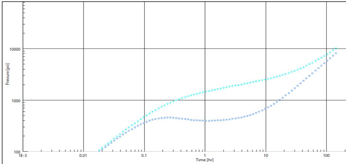
Figure 31: Deconvolved response of the build-up phases shown on a log-log plot in case of PSS
