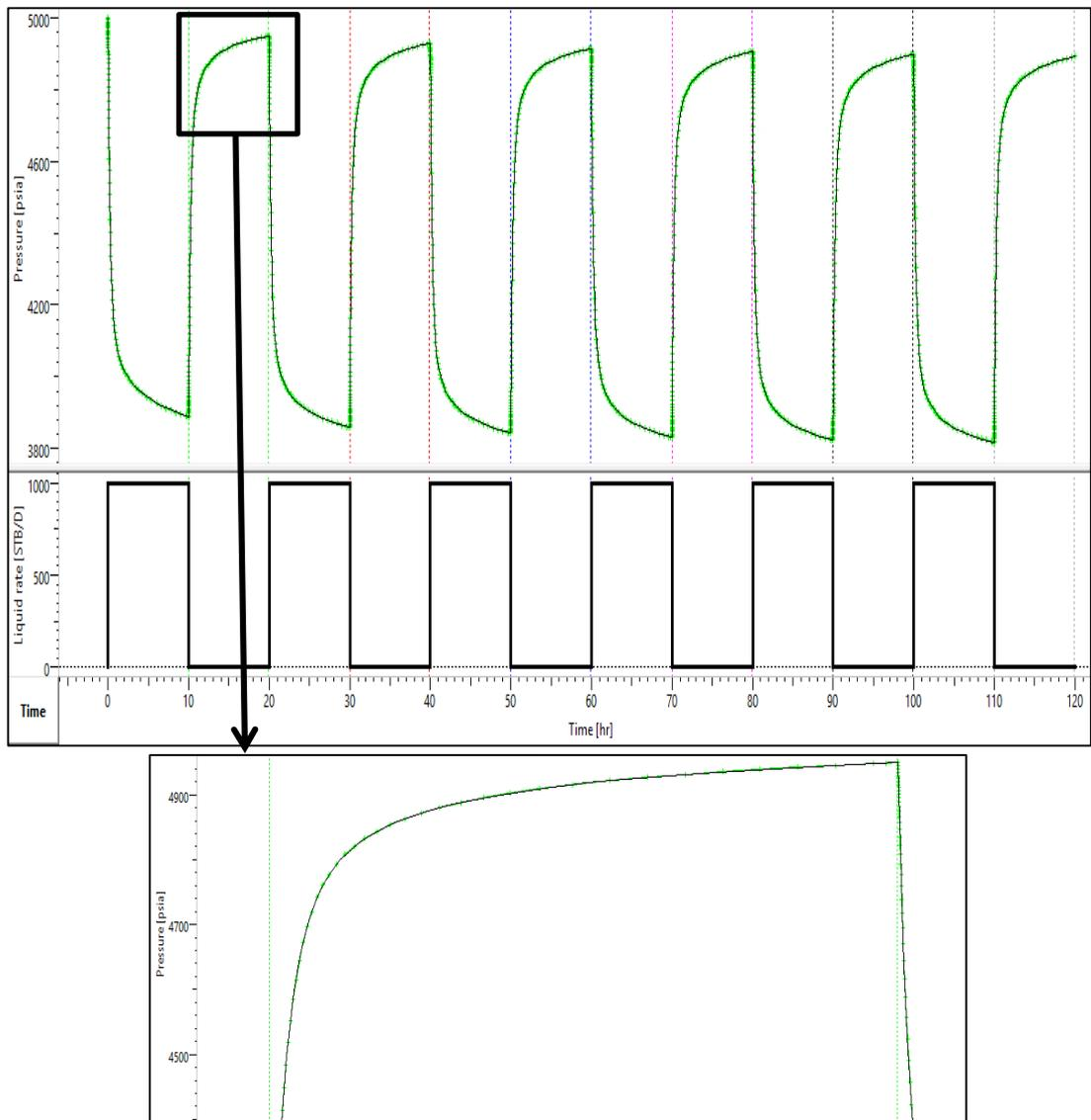
Figure 43: Pressure versus time plot showing match between deconvolved response and actual pressure data for net-positive case
