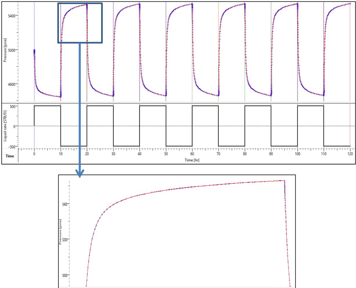
Figure 39: Pressure versus time plot showing the unchanged match even after the adjustments made on the deconvolved response after  $T=20$  hours
