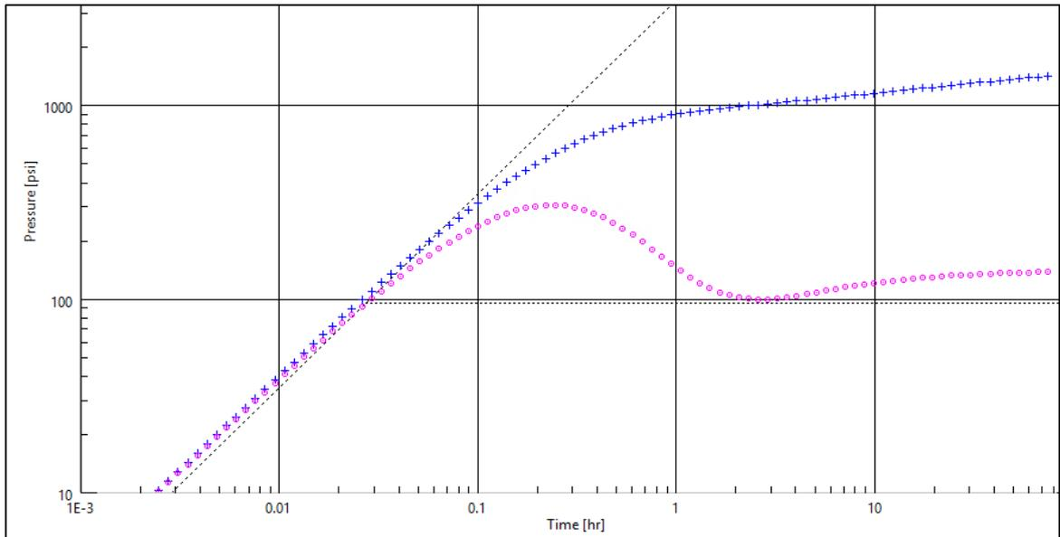
Figure 72: Log-log plot showing the results of deconvolution on the build-up phase of well 1
