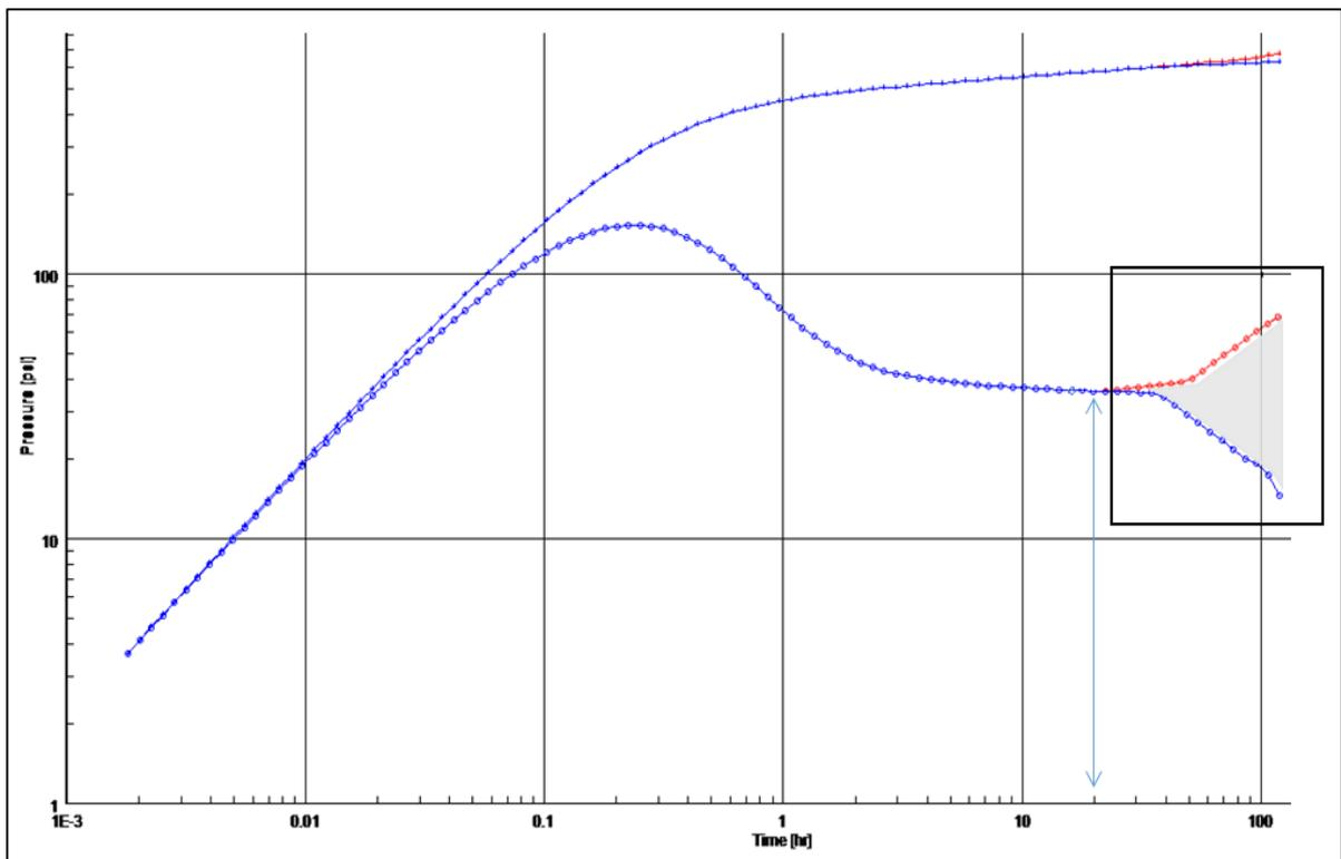
Figure 38: Log-log plot showing the changes made or that can be made on the deconvolved response after  $T=20$  hours in terms of a trumpet shape
