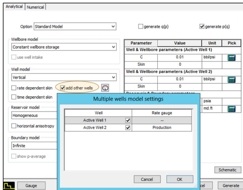
Figure 69: Test design on Saphir showing the addition of the other well
