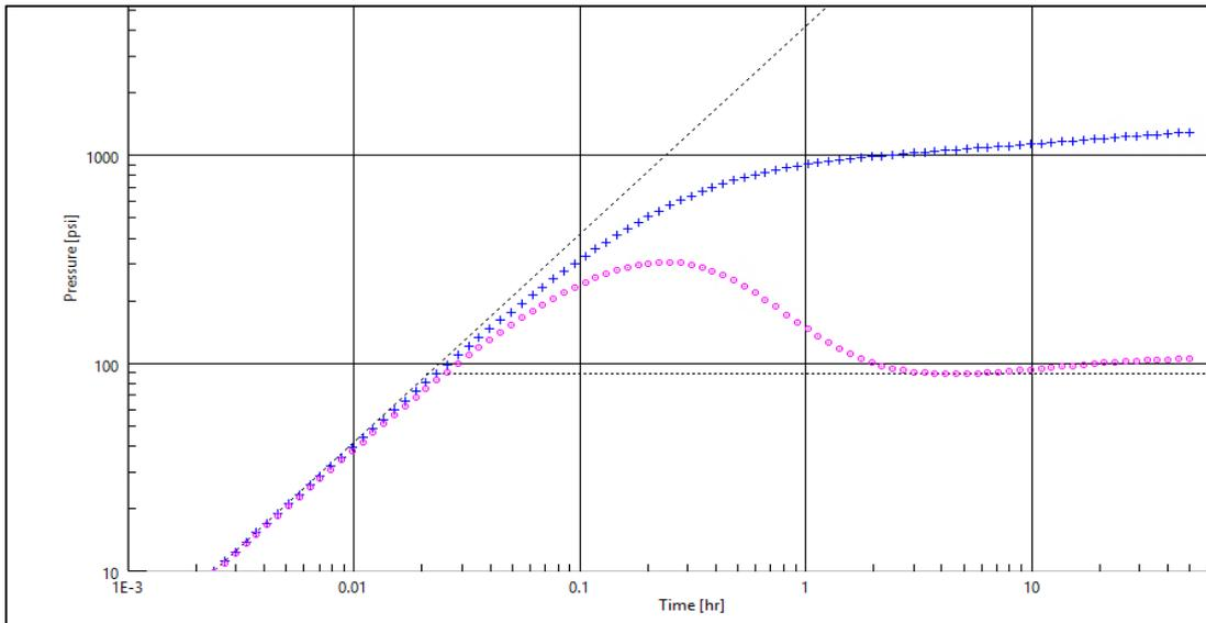
Figure 73: Log-log plot extracted for the build-up phase of well 1 after the change in the test sequence, showing the results of deconvolution
