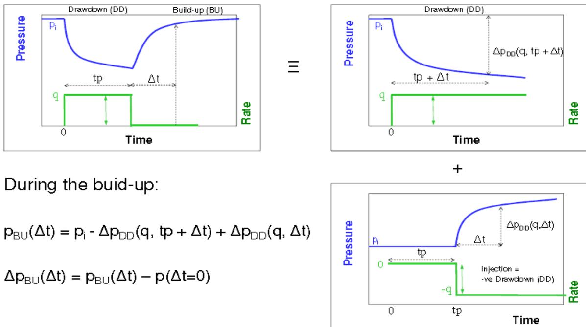
Figure 6: Superposition in Time for the build-up case with one constant rate<sup>[12]</sup>
