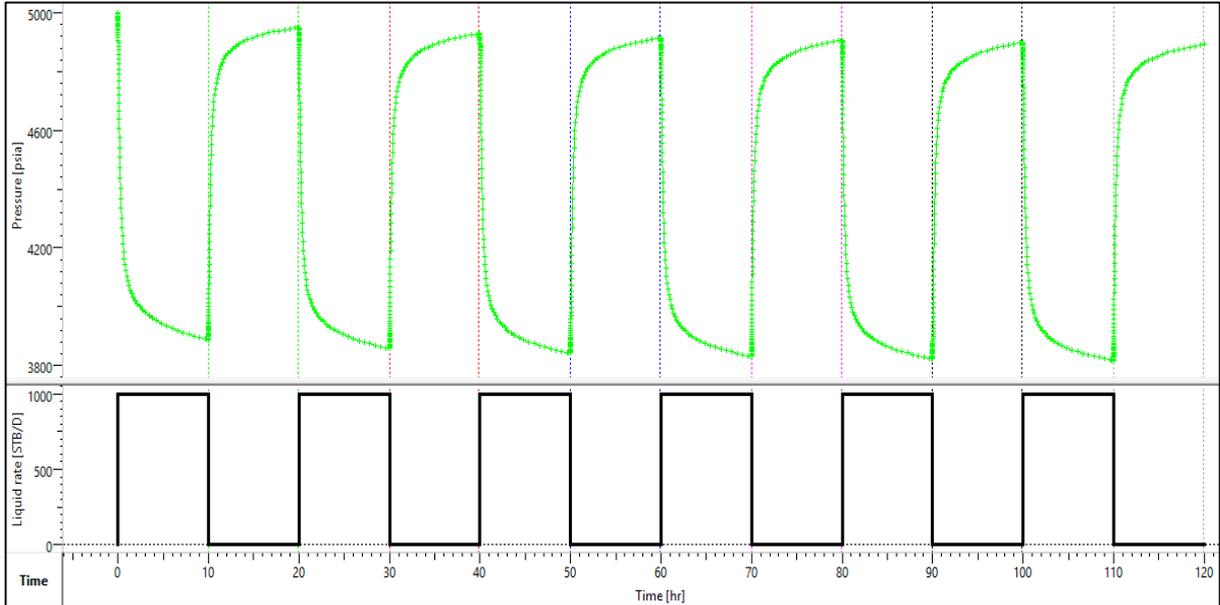
Figure 40: Pressure versus time plot for net-positive case
