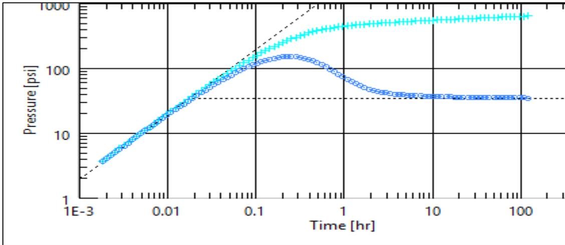
Figure 37: Log-log plot showing deconvolved response for the harmonic net-zero case with a total duration of 120 hours
