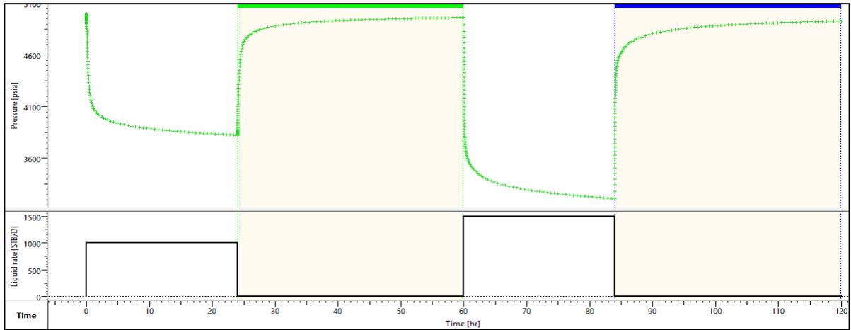
Figure 55: Pressure versus time plot showing two different flow periods with two build up periods with different wellbore storage effects
