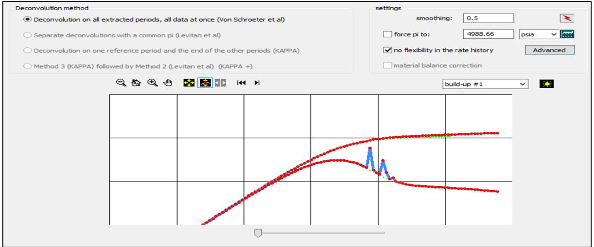
Figure 53: Deconvolution option on Saphir showing the adjustment of the deconvolved response points outside of the gap
