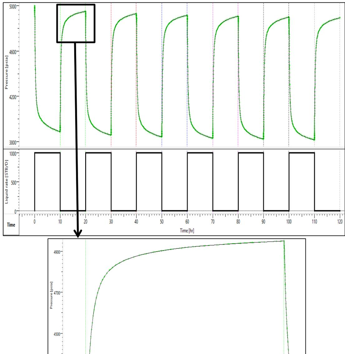
Figure 43: Pressure versus time plot showing match between deconvolved response and actual pressure data for net-positive case
