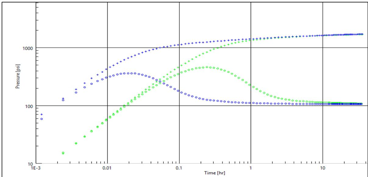
Figure 56: Log-log plot showing the difference in wellbore storage effects on the build-up periods with duration of 36 hours
