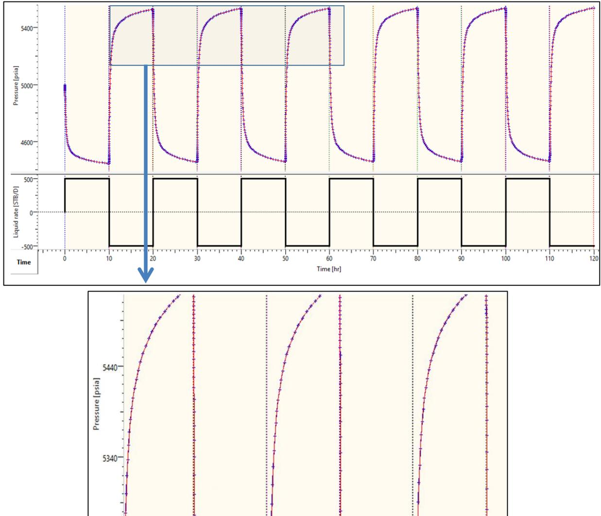
Figure 36: Pressure versus time plot showing match between deconvolved response and pressure data in a zoomed way
