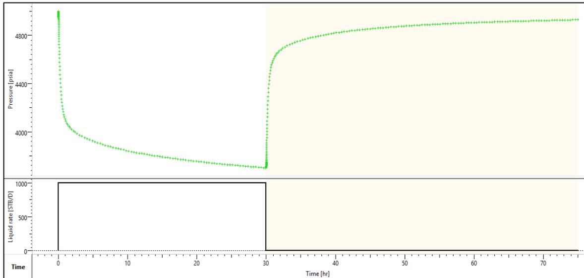
Figure 70: Pressure versus time plot extracted for the build-up phase of well 1
