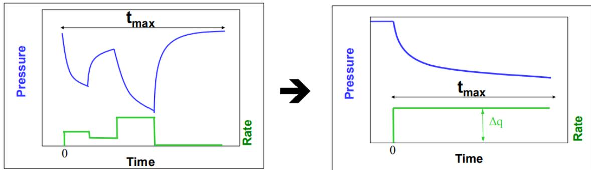
Figure 8: Deconvolution Principle<sup>[12]</sup>
