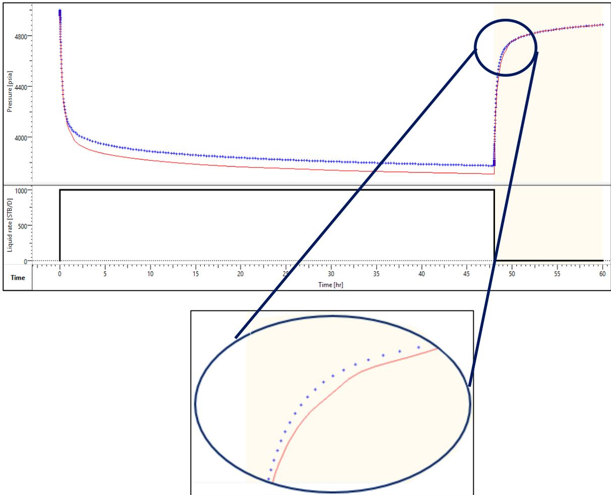
Figure 54: Mismatch of the actual pressure data and the deconvolved response in a zoomed way, due to the adjustment of the points in figure 53
