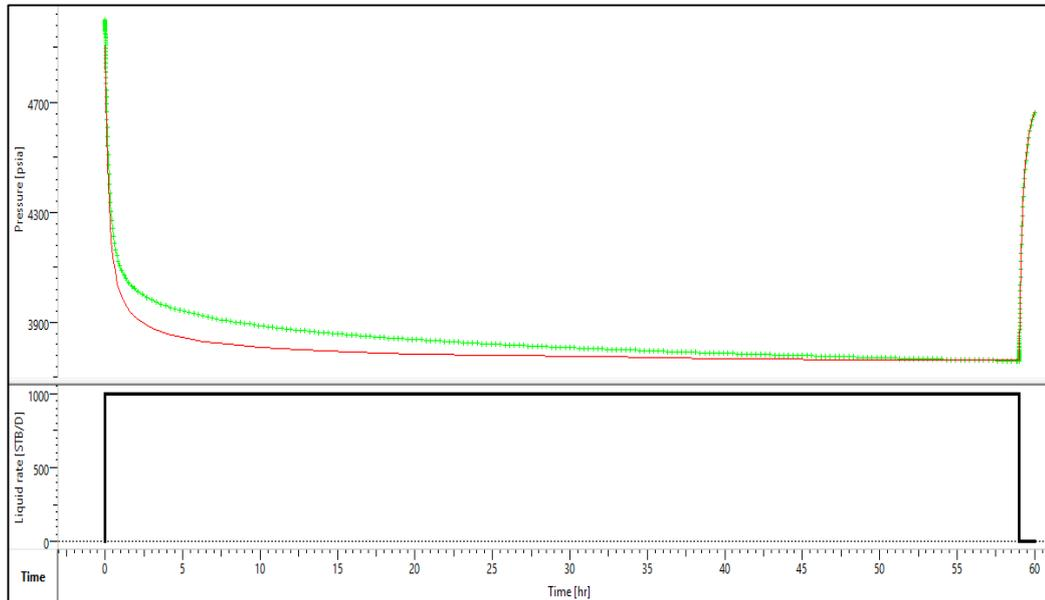
Figure 15: Pressure versus time plot showing the mismatch between original pressure data and deconvolved response
