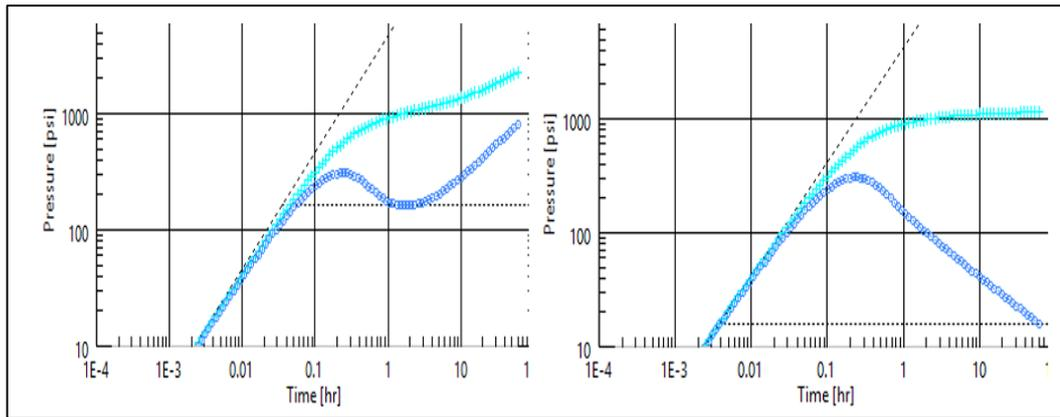
Figure 16: Log-log plot showing deconvolved responses for two different initial pressures  $P_i = 6000$  psi (left) and  $P_i = 4912$  psi (right)
