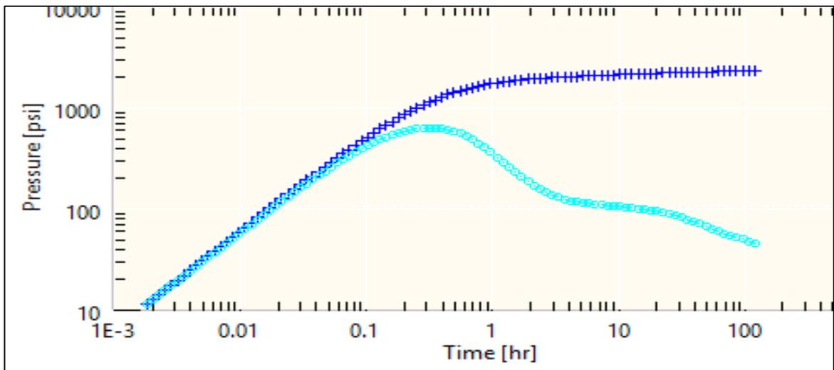
Figure 64: Deconvolved response on a log-log plot of the changing skin case, where deconvolution on all extracted periods was done
