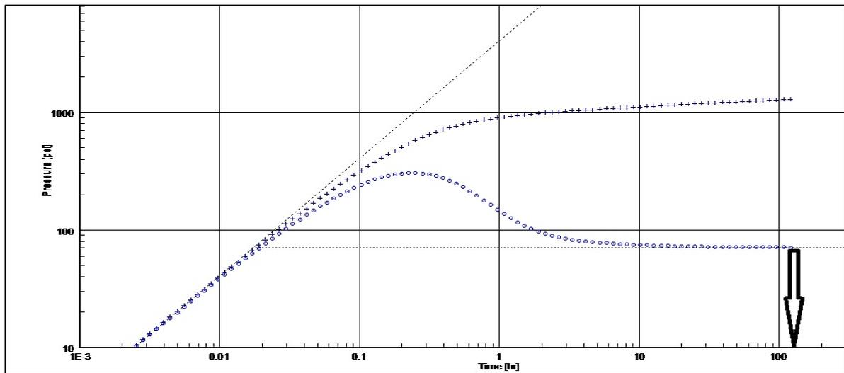
Figure 42: Log-log plot showing deconvolved response with the duration of 120 hours for net-positive case
