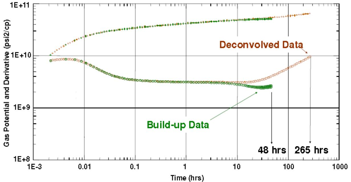
Figure 11: Example of a Deconvolution Response on a log-log plot for the case of Figure 10<sup>[12]</sup>
