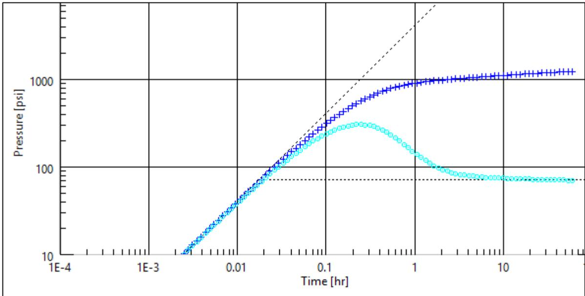
Figure 48: Deconvolved response on a log-log plot for the Gap case with a duration of 60 hours
