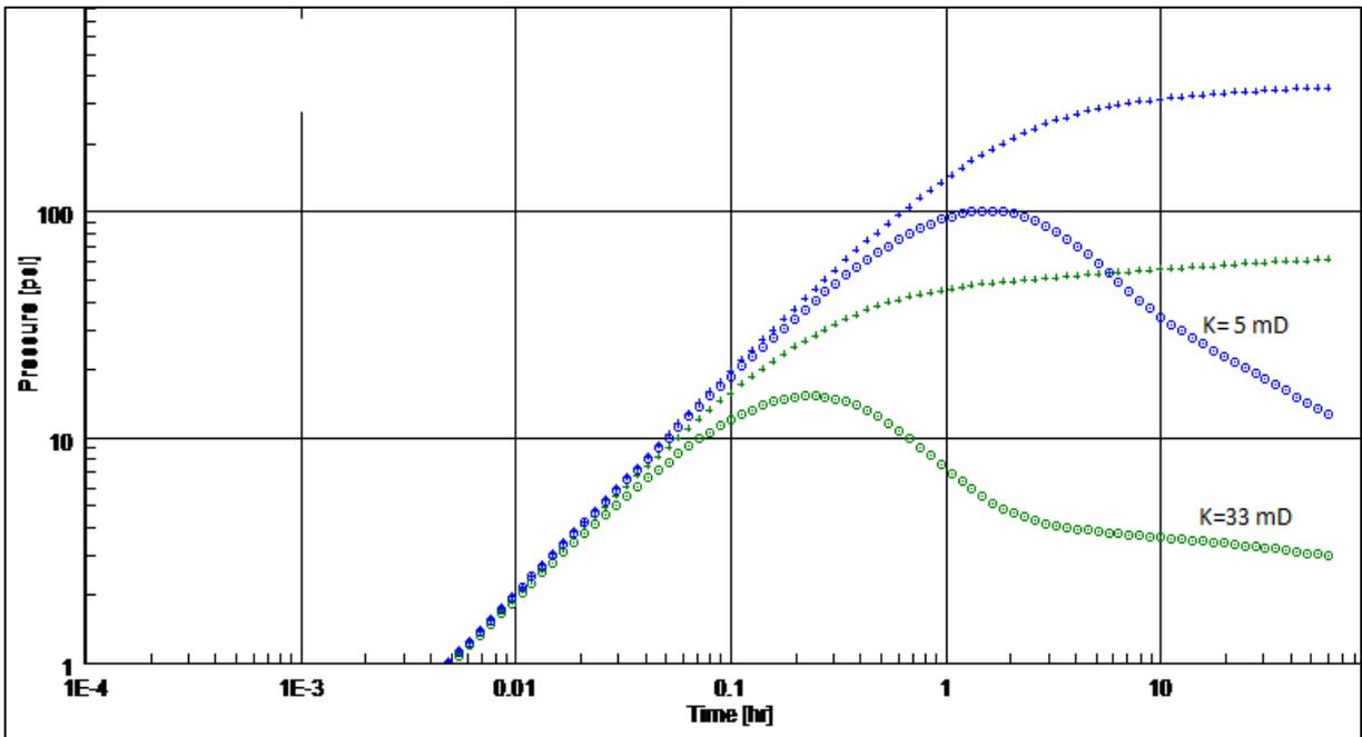
Figure 28: Comparison of the deconvolved responses of 2 different permeabilities on a log-log plot
