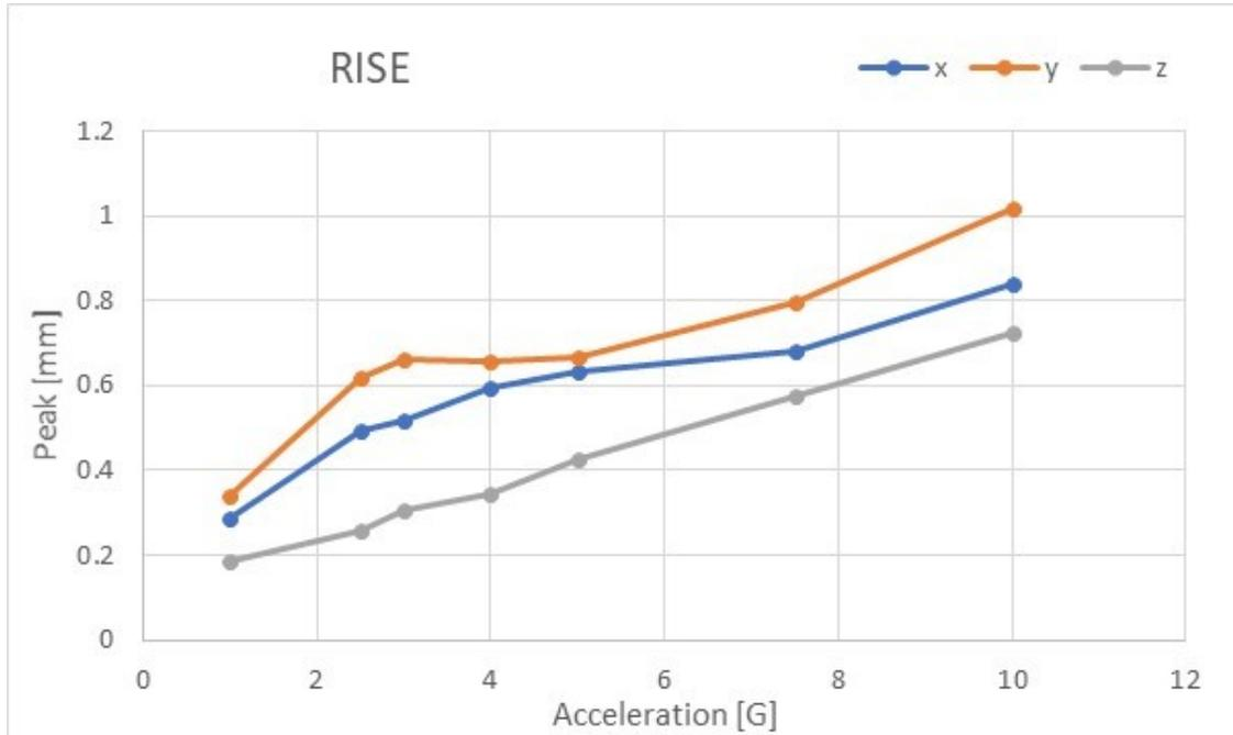
Figure 4.17. Carbon fibre arm, A-RISE controller, peak errors
