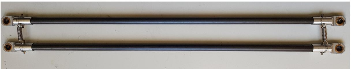
Figure 1.9. Forearm with peek coupling and spherical socket (WPS)
