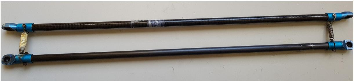
Figure 1.8. Forearm with aluminium coupling and spherical socket (GAS)
