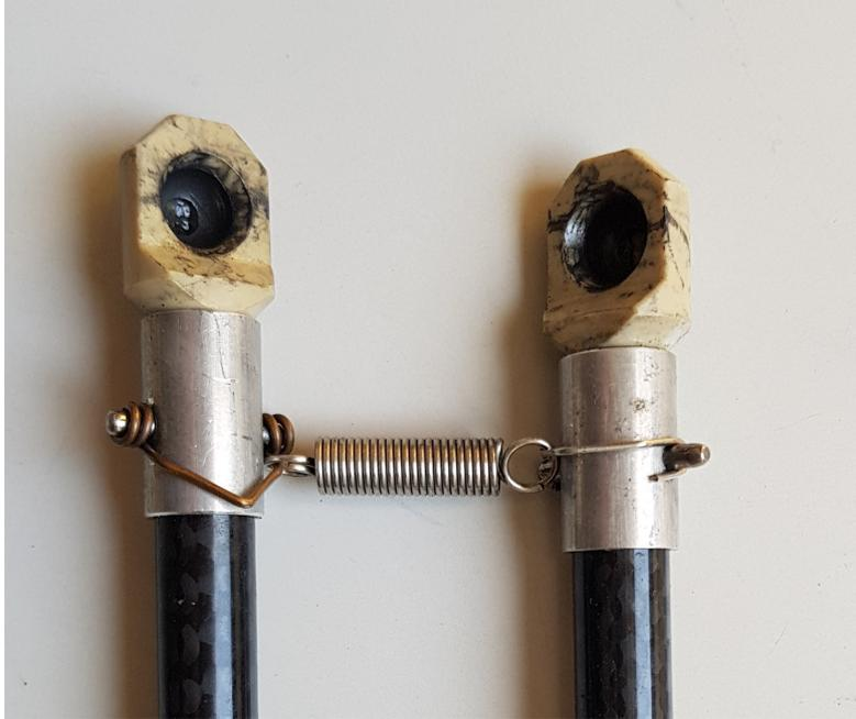
Figure 1.10. Forearm with aluminium coupling and conical socket (BAC)
