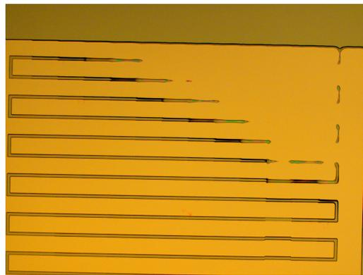
Figure 4.3: Incomplete development due to the presence of edge beads
