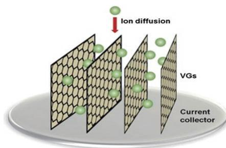
Figure 2.7: Vertically Oriented Graphene structure and ions diffusion.[3]
