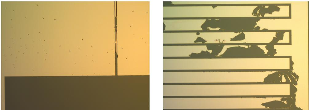
*Figure 4.5: Defects occurred during Gold lift-off*
