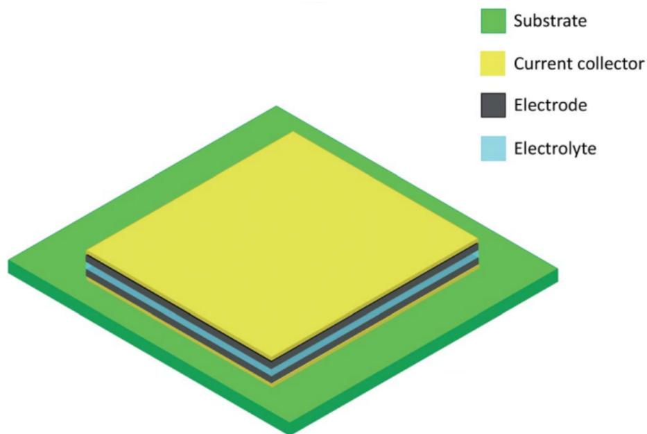
Figure 3.1: 2D in-plane architecture[5]
