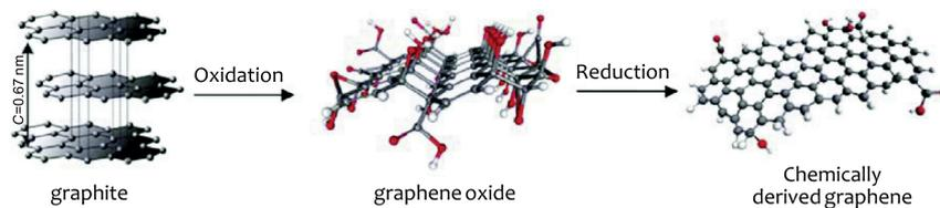
Figure 2.6: Graphene oxide reduction[2]
