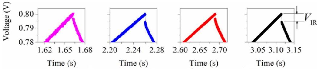
Figure 5.5: IR drops in galvanostatic charge/discharge measurements
