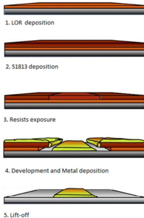
Figure 4.1: Bi-layer lift-off process [6]
