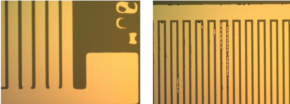
*Figure 4.6: Defects occurred during Palladium lift-off*
