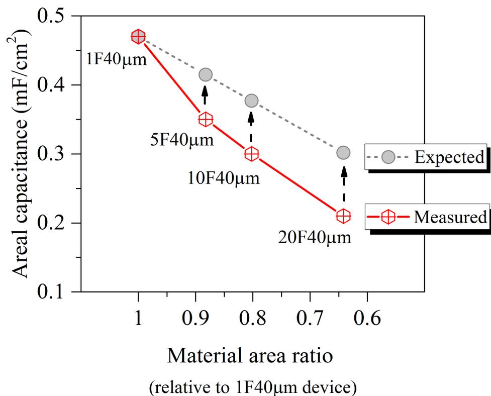
Figure 5.6: Areal capacitance of devices as function of electrode material area ratio
