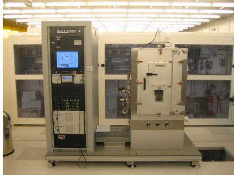
Figure 4.4: Lesker PVD 225 used for metal evaporation
