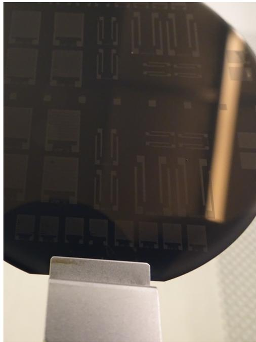
Figure 4.8: VG growth on wafer pattern with the second mask
