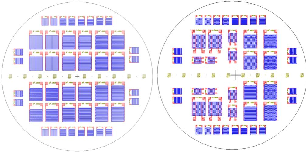
Figure 3.4: Masks designed using L-Edit
