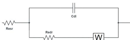
Figure 2.10: EDLC equivalent circuit
