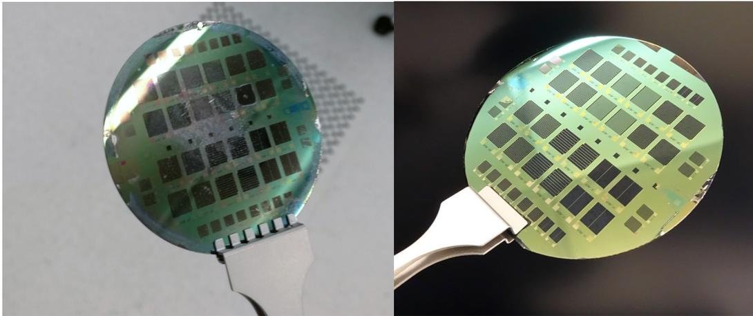
Figure 4.11: Left: rGO wafer; Right: VOG wafer
