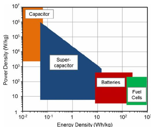
Figure 2.4: Ragone plot of different electrochemical energy storage devices [1]
