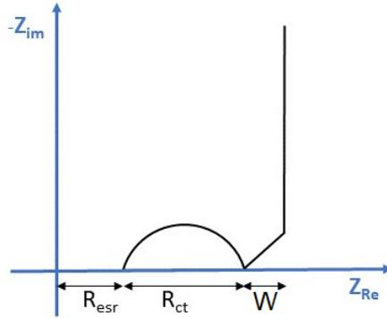
Figure 2.9: Example of EIS curve for an EDLC
