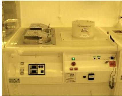
Figure 4.7: Laurell WS-400-6NPP-LITE/IND spinner and two BLE hotplates
