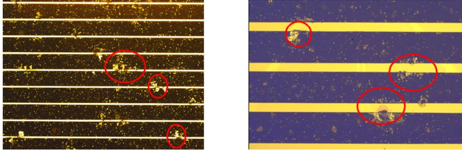
Figure 4.10: (a) Electrodes short circuit due to Al re-deposition (b) Non critical Al re-deposition
