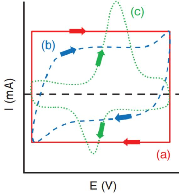
Figure 2.8: Cyclic voltammogram curves of (a) ideal capacitor, (b) EDLC, and (c) pseudocapacitive materials.[4]
