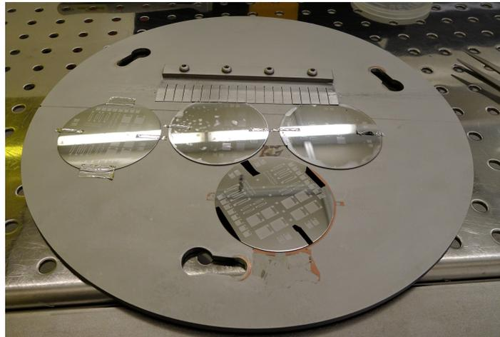
Figure 4.9: Four wafers after Aluminum evaporation
