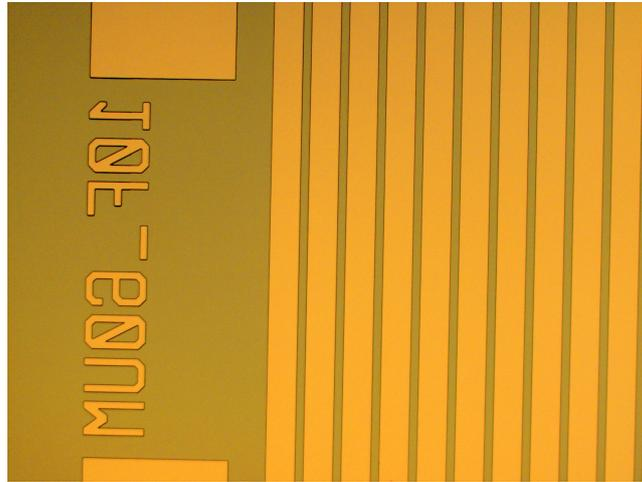
Figure 4.2: Detail of a micro-supercapacitors after development
