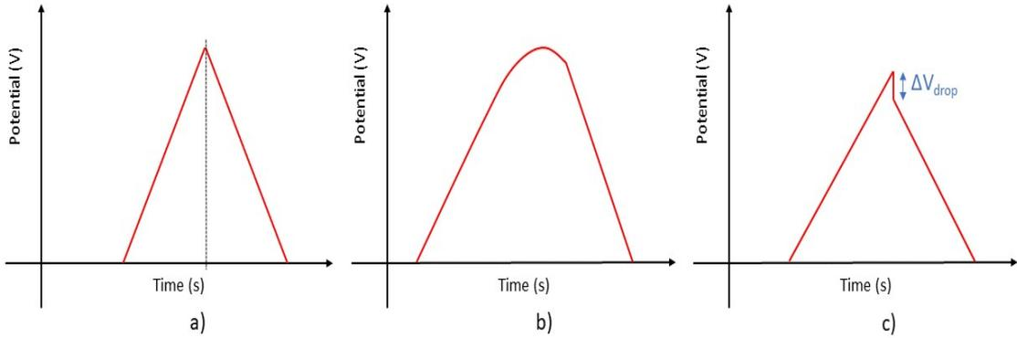
Figure 2.11: GCD curves of ideal EDLC and the effect of non ideal phenomena
