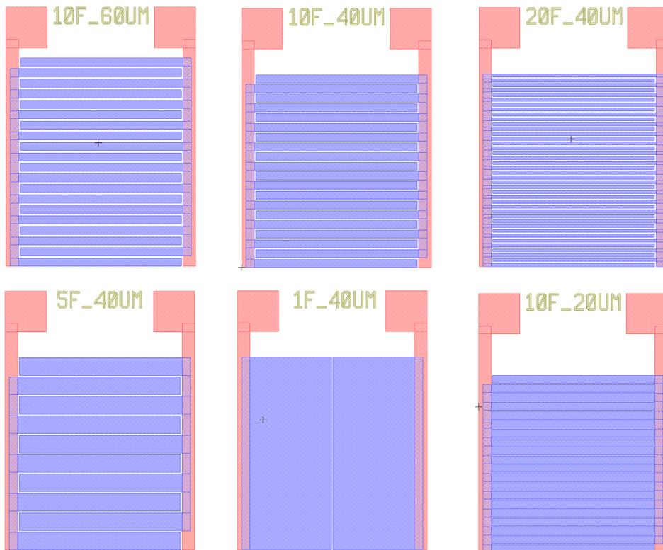
Figure 3.5: L-edit models of different device geometries
