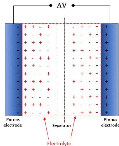
Figure 2.1: EDLC schematic
