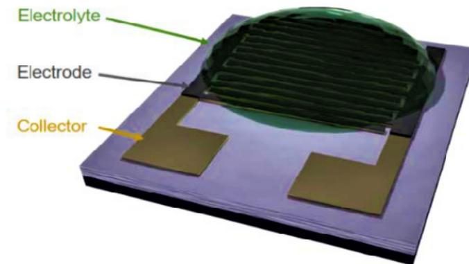
Figure 3.2: 2D interdigitated architecture
