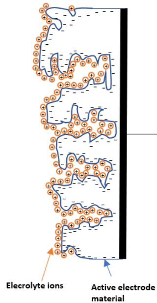
Figure 2.5: Representation of an EDLC's electrode with porous electrode materials
