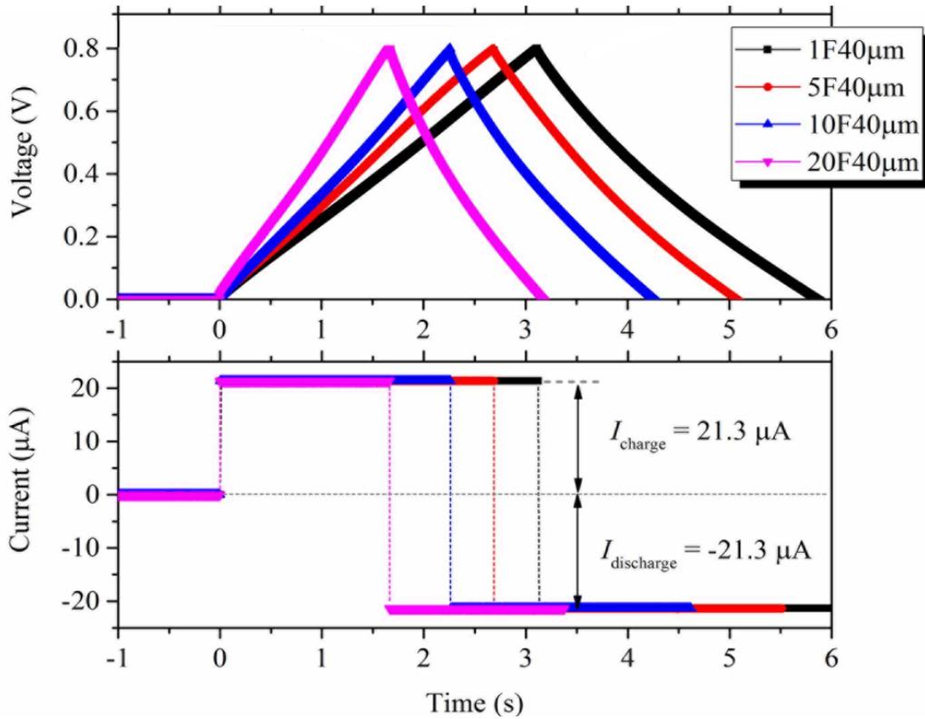
Figure 5.4: Galvanostatic charge/discharge measurements at current density of  $100 \mu\text{A}/\text{cm}^2$
