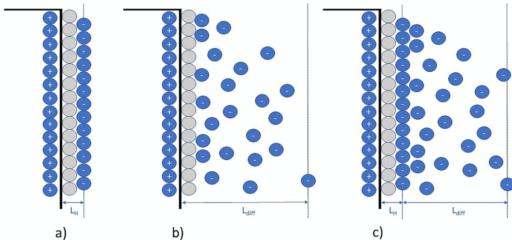
Figure 2.2: Representation of the EDLC Models: Helmholtz model a), Gouy-Chapman model b) and Stern-Grahame model c)
