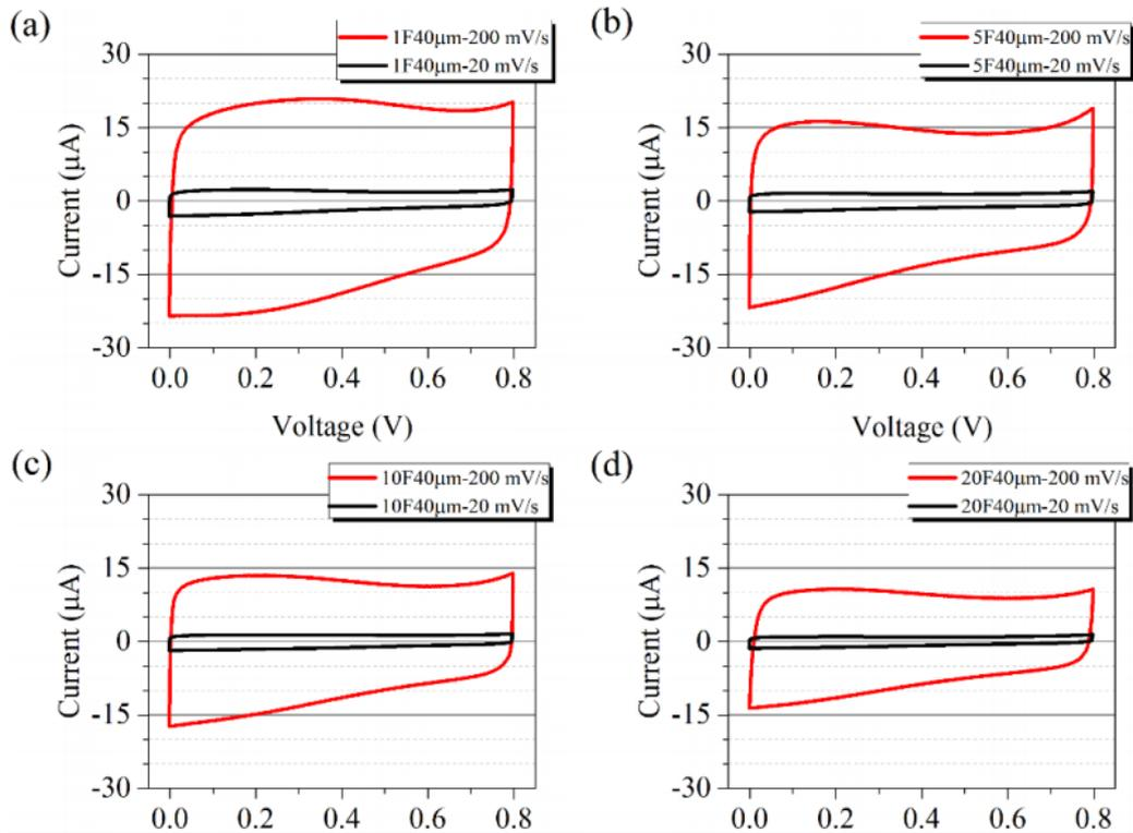
Figure 5.3: Cyclic Voltammograms of different device geometries: a) 1F40 $\mu\text{m}$ , b) 5F40 $\mu\text{m}$ , c) 10F40 $\mu\text{m}$ , d) 20F40 $\mu\text{m}$
