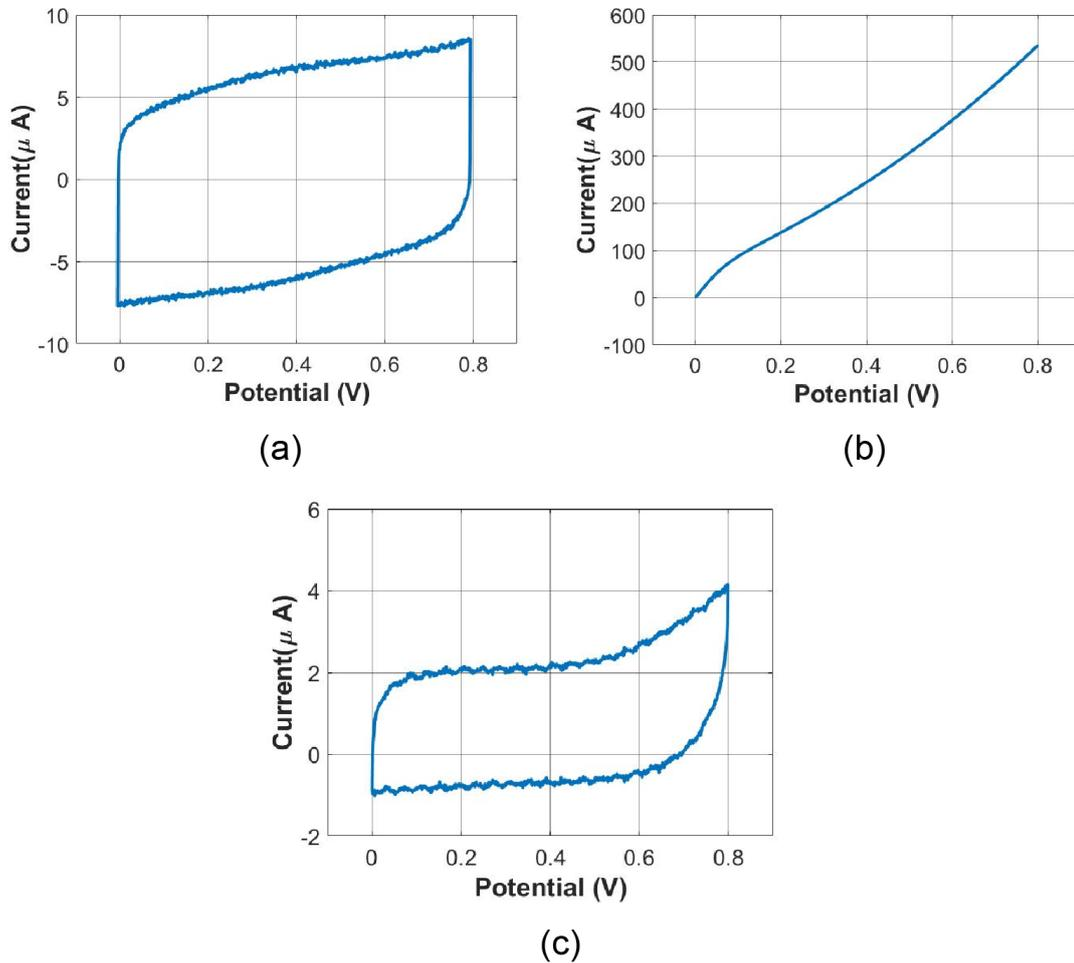
Figure 5.2: Cyclic Voltammograms of: (a) Ti/Au current collectors. (b) Pd sample. (c) Ti-Pd sample
