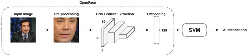
Figure 4.1: Face-based authentication system workflow.
