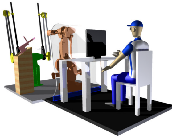
Figure 10: Off-line robot programming concept. Working in an office environment, the user can generate robot programs without interrupting production process [19]
