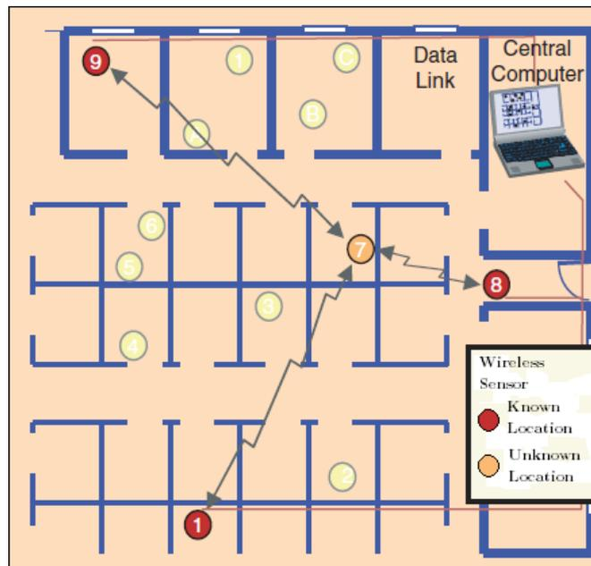
Figure 3. Localization Centralized Approach [8].
