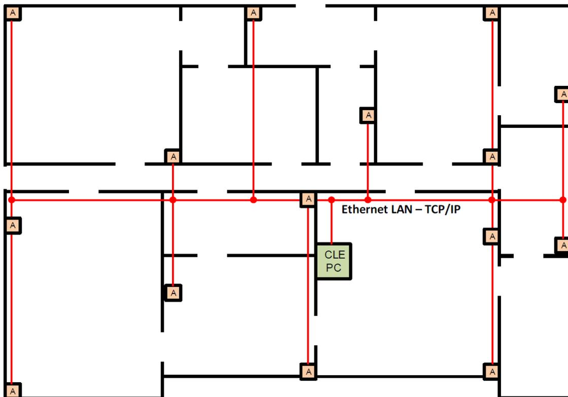
Figure 5. Typical expanded RTLS system with central location engine (CLE) [32].
