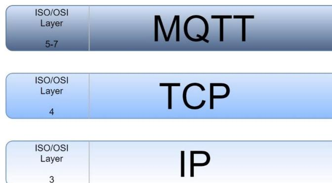
Figure 24. MQTT stack.
