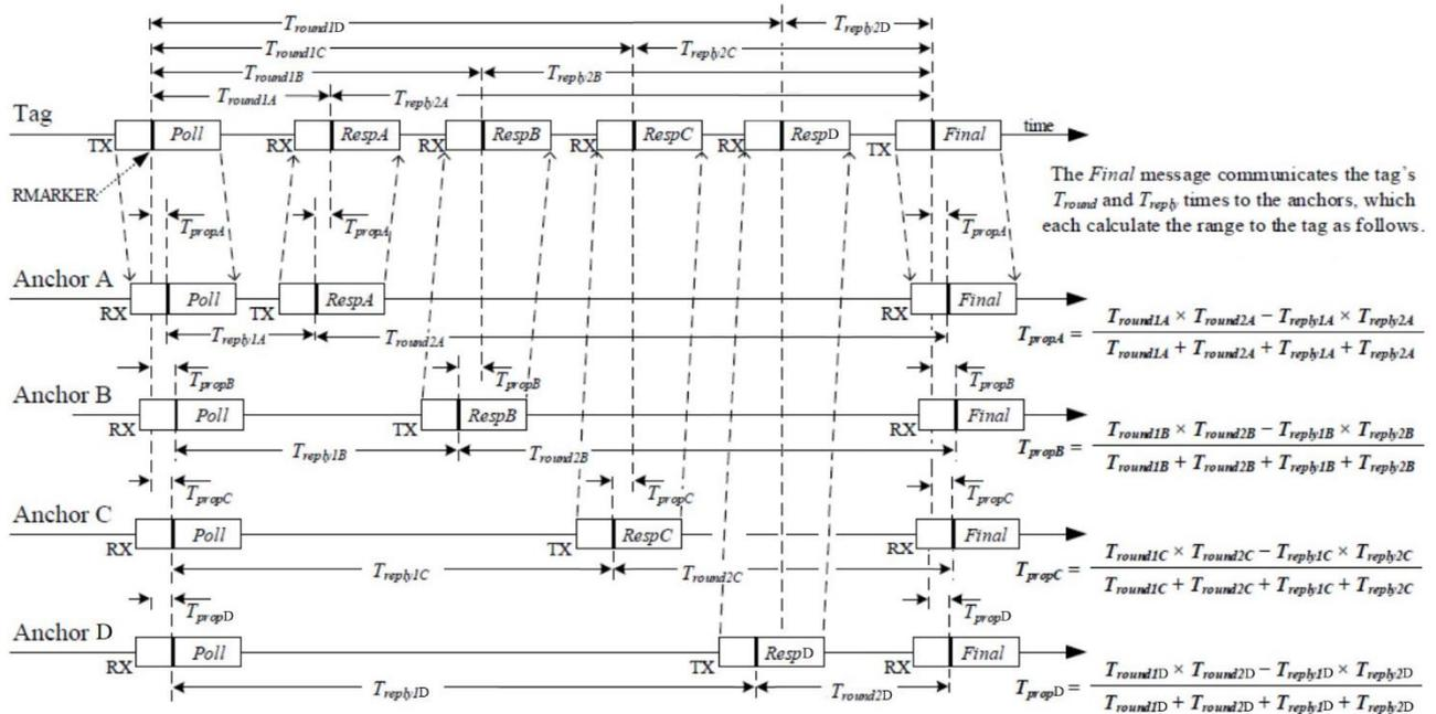
Figure 30. Two-way ranging to four anchors [17].
