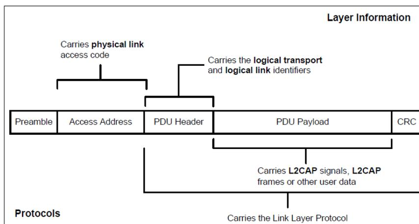
Figure 16. Entire BLE packet structure [24].
