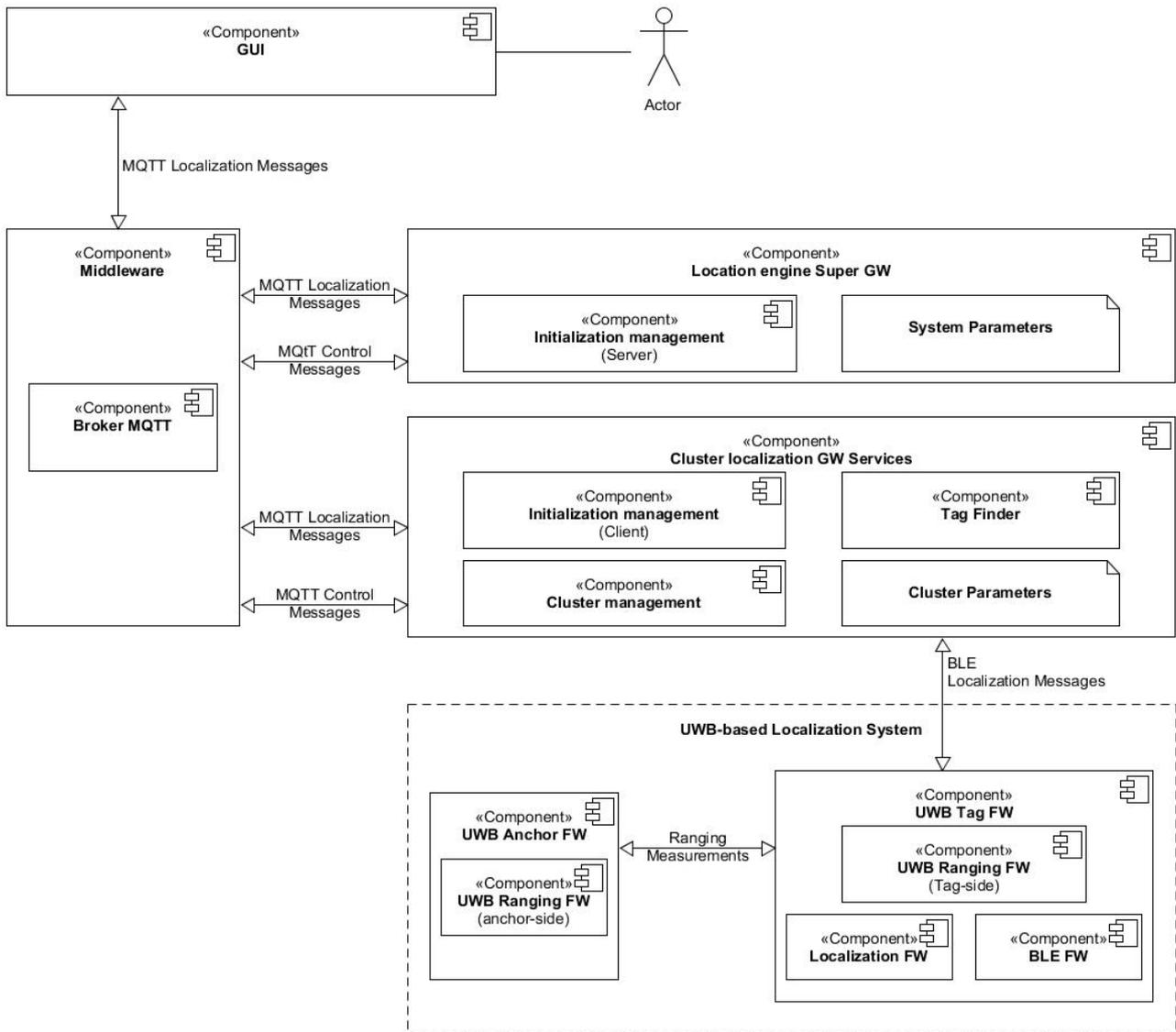
Figure 35. Large-Scale system Functional Architecture.
