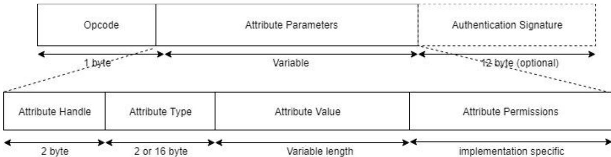
Figure 20. Example for GATT PDU structure [24].
