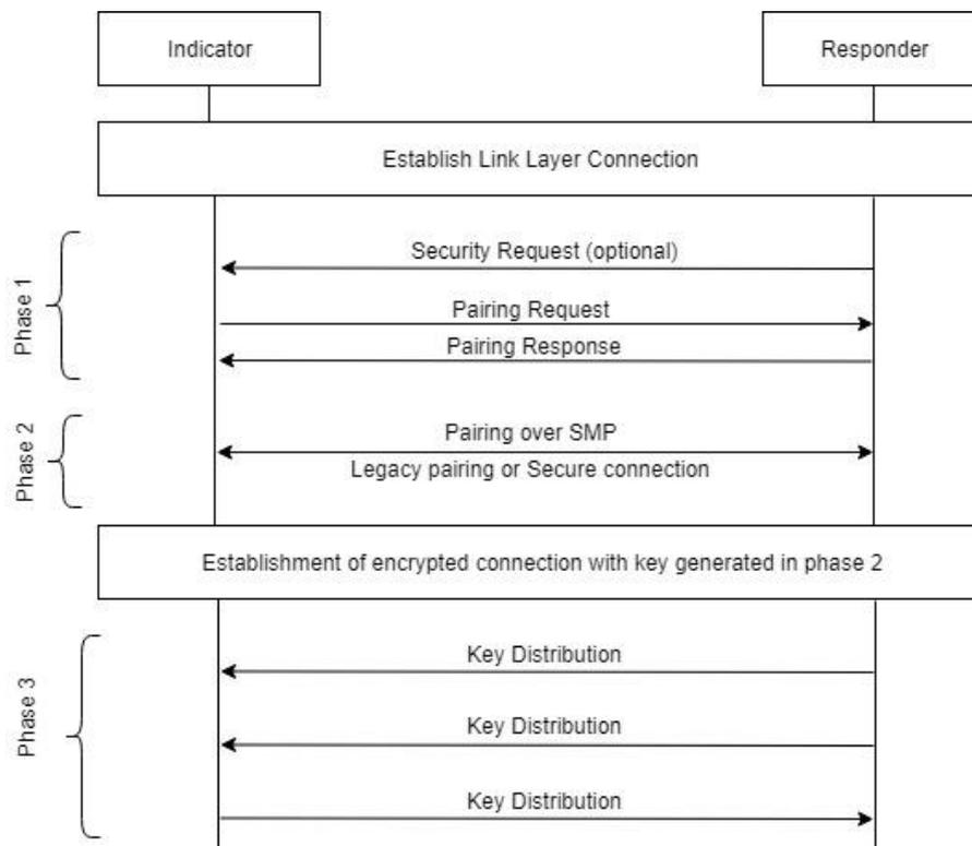
Figure 21. The BLE pairing phases [24].
