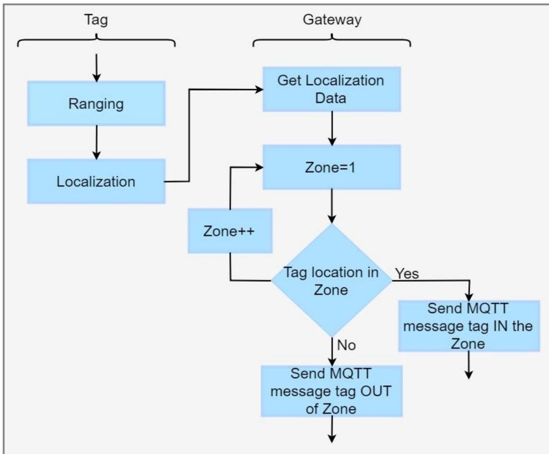
Figure 48. Zone control algorithm.
