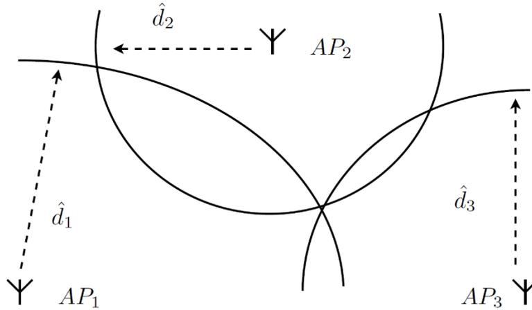
Figure 6. Example of using 2D trilateration for locating a tag. By estimating the distance between the tag and each of the three application points (TOF/RSS), the location of the tag can be estimated by finding the intersection of the three circles [1].
