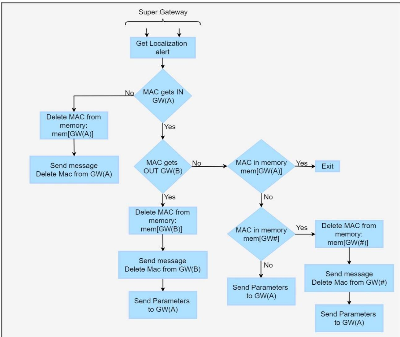
Figure 49. Switching algorithm.
