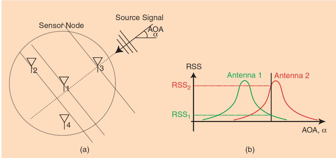
Figure 2. AOA estimation methods. (a) AOA is estimated from the TOA differences among sensor elements embedded in the node; a four-element Y-shaped array is shown. (b) AOA can also be estimated from the RSS ratio  $RSS_1/RSS_2$  between directional antennas [8].
