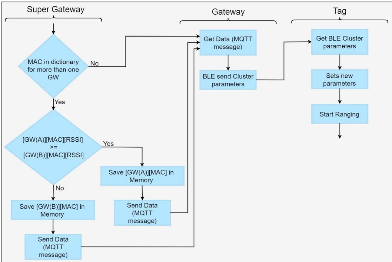
Figure 47. Cluster Assignment algorithm.
