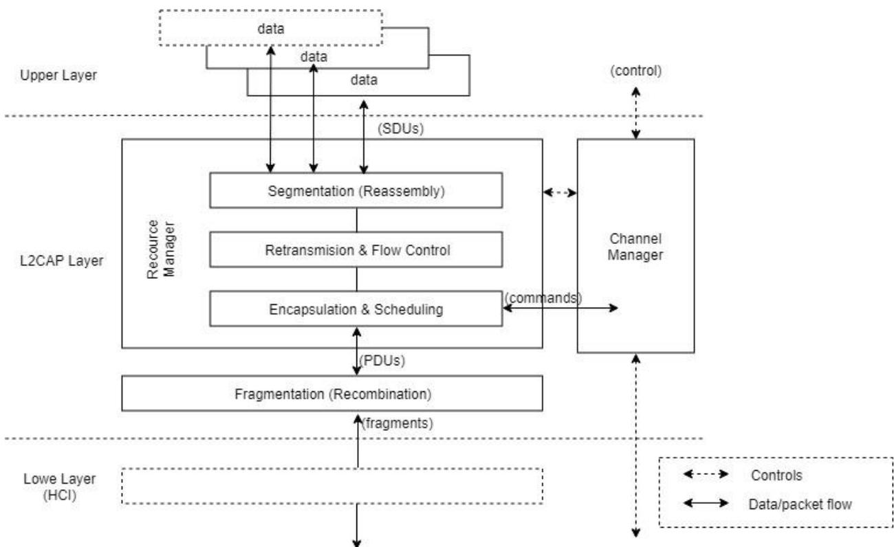
Figure 17. Illustration of the BLE L2CAP layer architecture [24].
