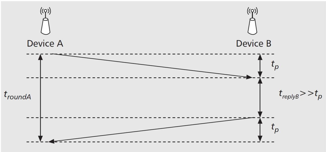
Figure 9. Exchange of message in two-way ranging [21].
