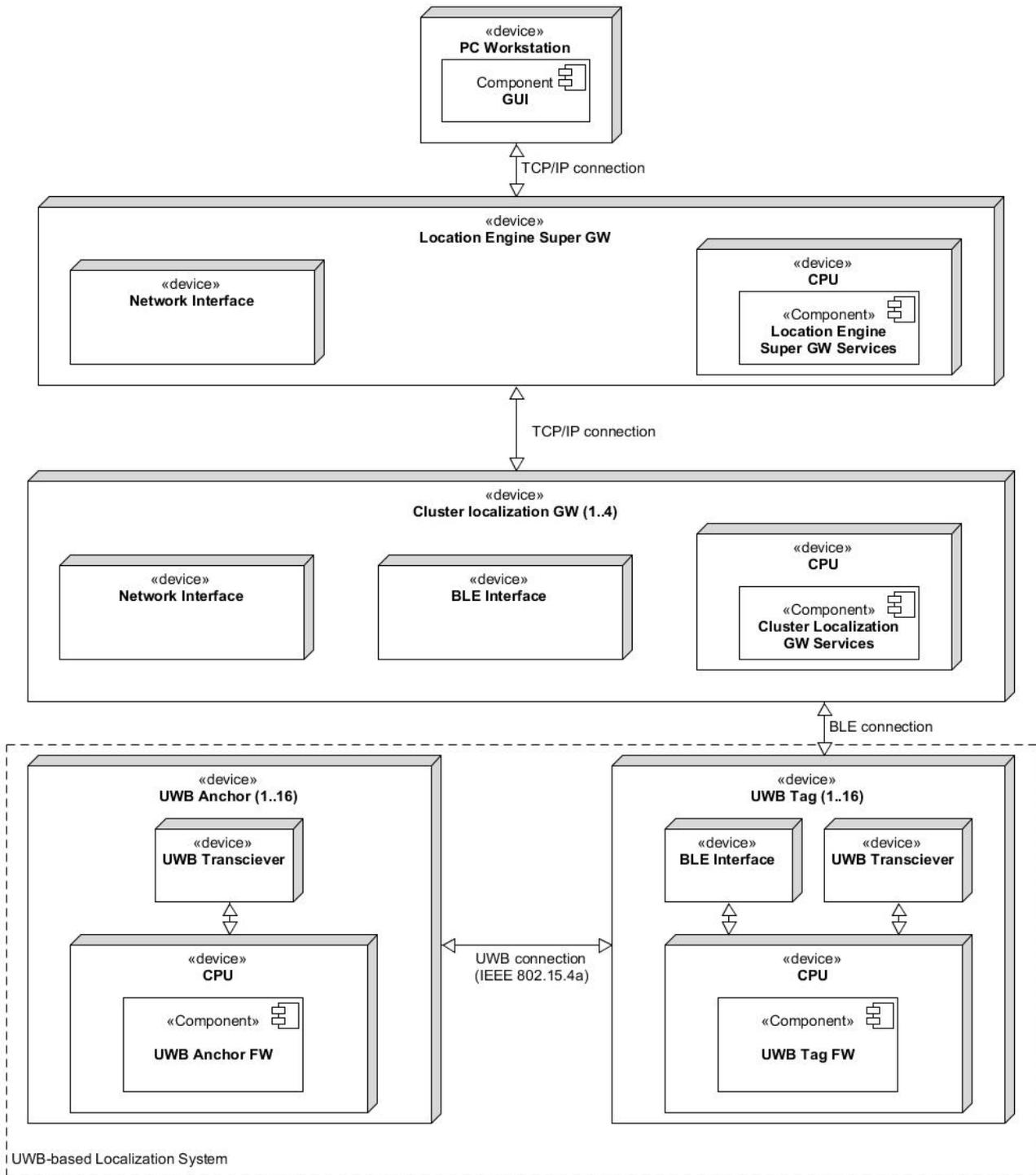
Figure 36. Large-Scale system Deployment Architecture.
