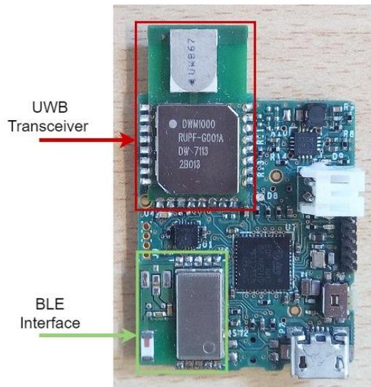
Figure 37. Custom ISMB Tag PCB.
