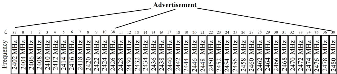
Figure 11. The BLE channel built-up.
