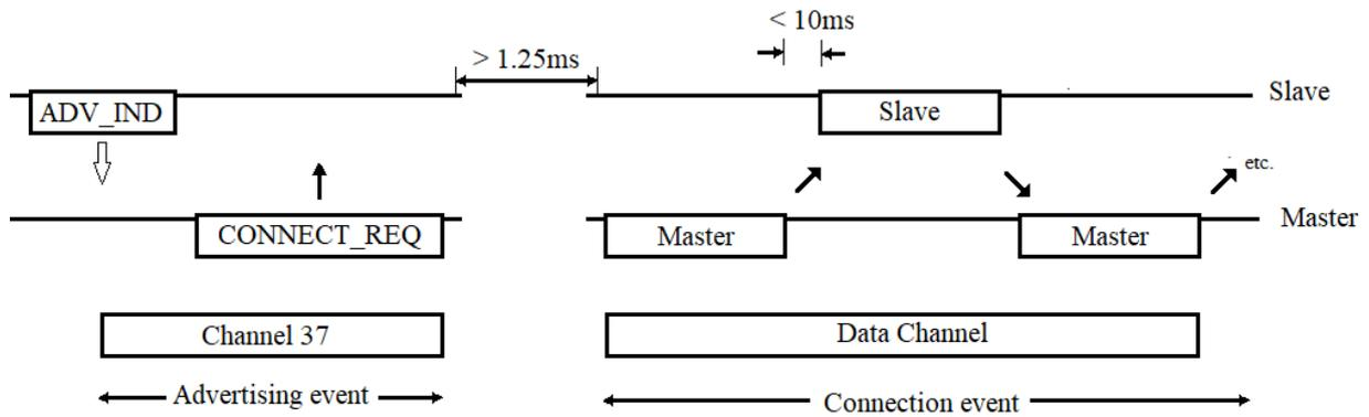
Figure 13. Illustration of a BLE connection event [24].
