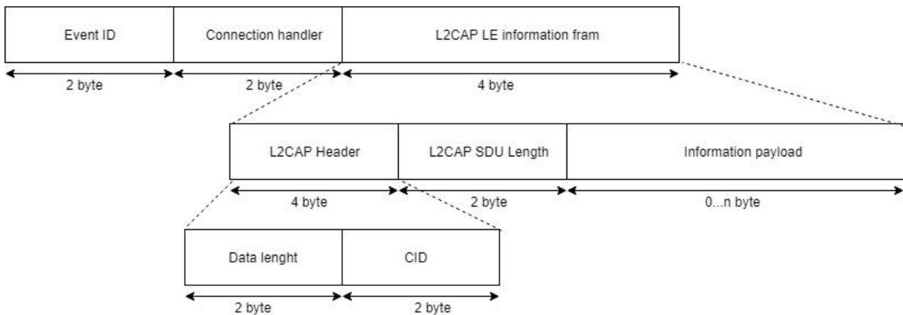
Figure 18. Structure of the L2CAP packet [24].
