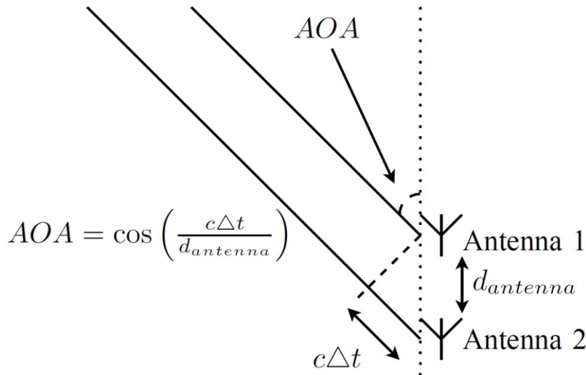
Figure 1. An angle of arrival system using two antennas. By utilizing the difference in the time of an arrival of a signal at the antenna pair ( $\Delta t$ ) along with the antenna spacing  $d_{antenna}$ , the arrival direction can be estimated [1].
