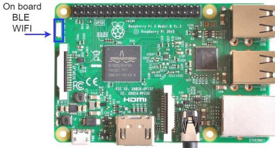
Figure 39. Raspberry Pi 3 Model B.
