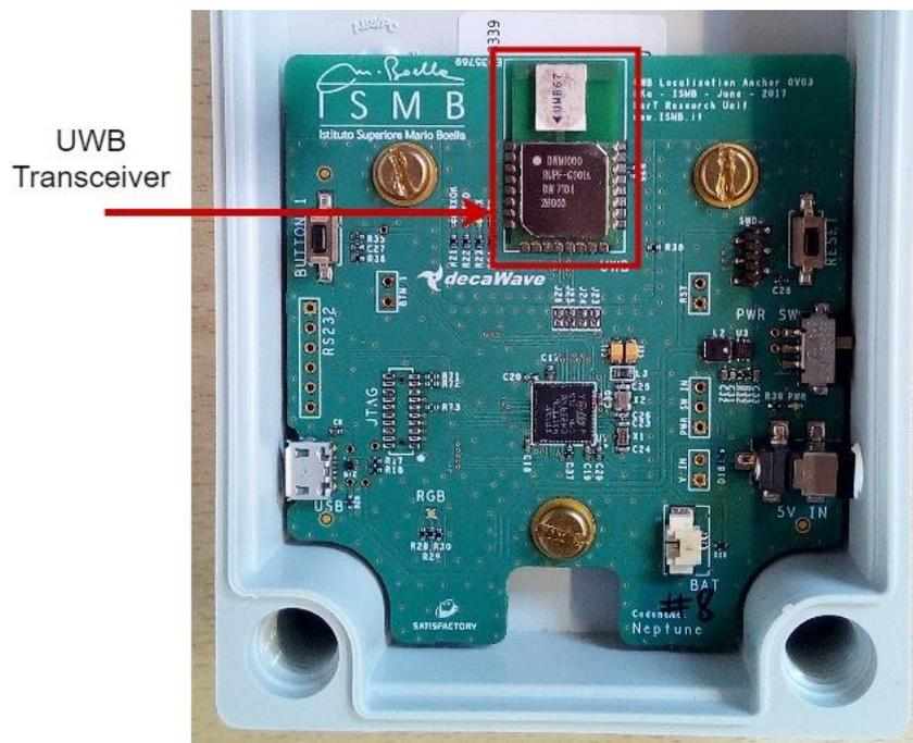
Figure 38. Custom ISMB Anchor PCB
