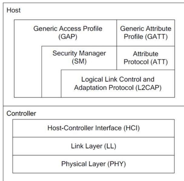
Figure 10. The BLE protocol Stack [25].
