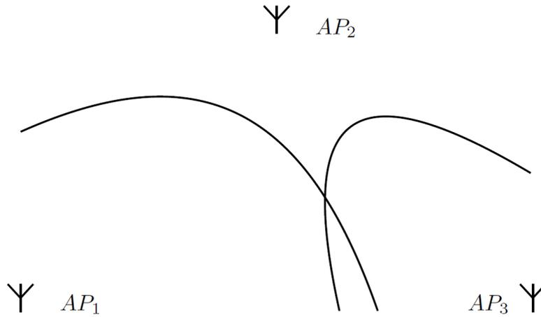
Figure 7. Example of using 2D multilateration for locating a tag. Application point two is taken as the system origin and two hyperbola traced using the time difference of arrival values and the intersection point of these two is the location of the tag. [1].
