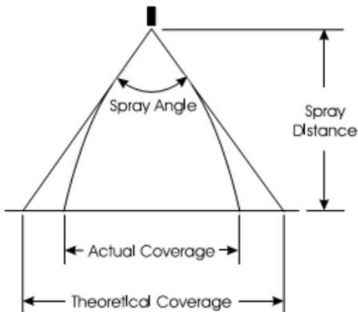
Figure 15: Actual vs theoretical coverage area (Relab Spray & Purification Technology Ltd.).
