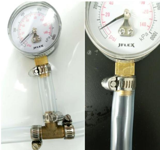
*Figure 17: Pressure meter sub-assembly.*
