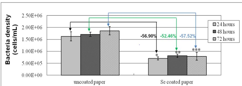
Figure 9: *E. coli* density on both uncoated and coated paper towels after 24, 48 and 72 hours (Wang, 2015, p.93).
