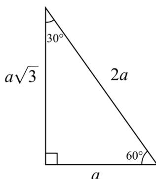
Figure 14: Spray aperture angle, one side. Note that the nozzle is supposed to be at the top of the triangle, and that the real spray shape will be the cone obtained by revolving the above image around its vertical axis.
