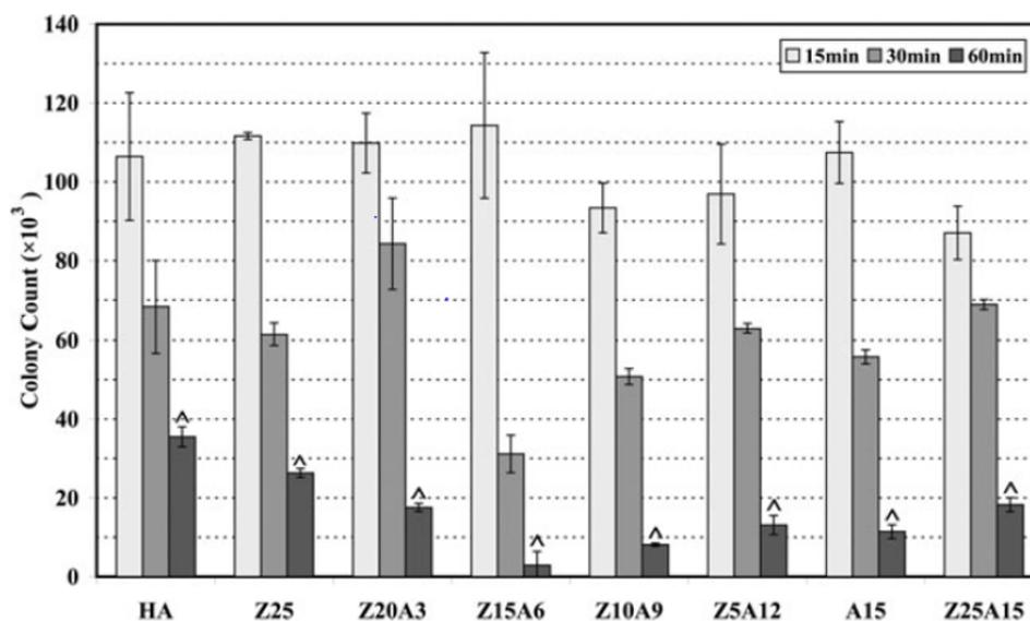
Figure 3: Antimicrobial solution used vs. Colony count after 15, 30 and 60 minutes of incubation (Samani et al., 2013, p.228).
