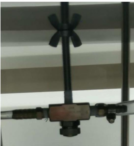
Figure 16: Threaded rod and nozzle used in the prototype.
