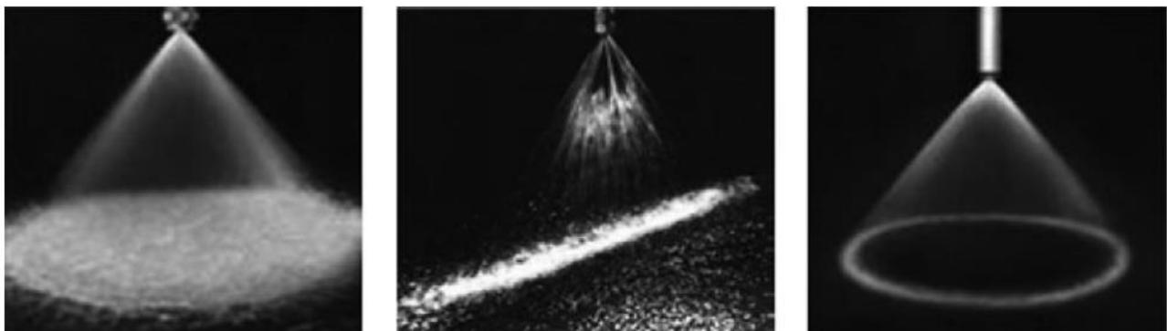
Figure 13: Full cone, flat fan and hollow cone. Respectively from left to right.
