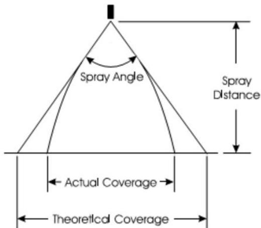
Figure 20: Actual vs theoretical coverage area (Relab Spray & Purification Technology Ltd.).
