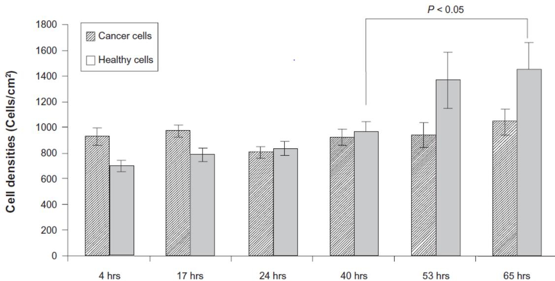
Figure 5: Densities of cancer cells and healthy cells on Se-coated Ti substrate after 4, 17, 24, 40, 53 and 65 hours after culturing (Tran et al., 2010, p.357).
