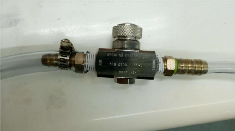
Figure 18: *Spraying System Co. Air atomising nozzle used for the experiments.*
