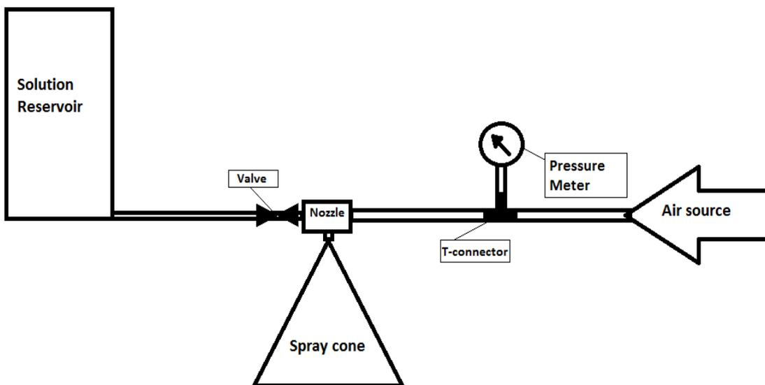
Figure 21: Schematic of the gravity-fed spray coating prototype.
