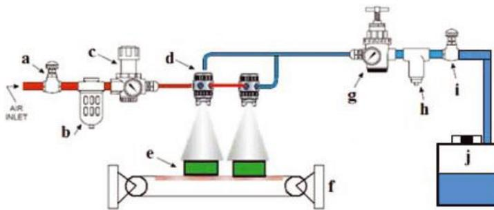
Figure 10: Sketch of industrial spray system, comprising shut-off valves for both air and liquid, air filter, gauges, nozzles, a conveyor belt and a tank (Andrade, 2012, p.330).
