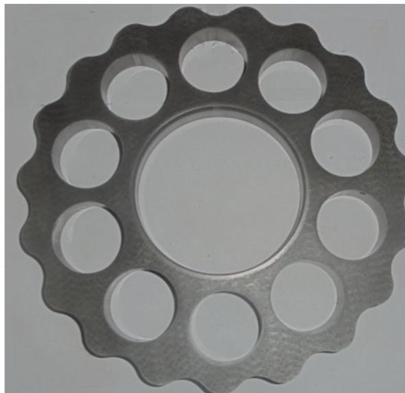
Figure 4.2: Tested cycloidal drive: cycloidal plate
