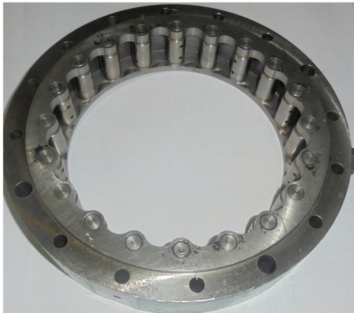
Figure 4.4: Tested cycloidal drive: housing with pins
