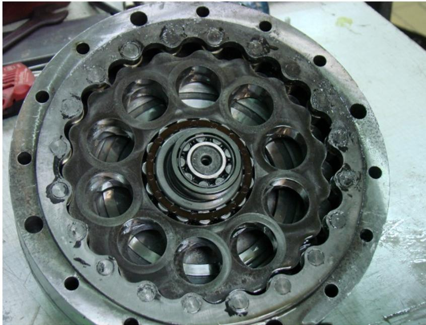
Figure 4.1: Tested cycloidal drive: cyclo gearbox
