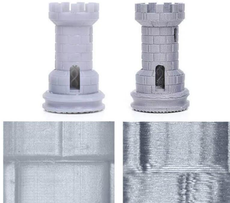
*Figure 2-4 Comparison between 3D printed objects from a SLA printer (Left) and a FDM printer (right)[31]*
