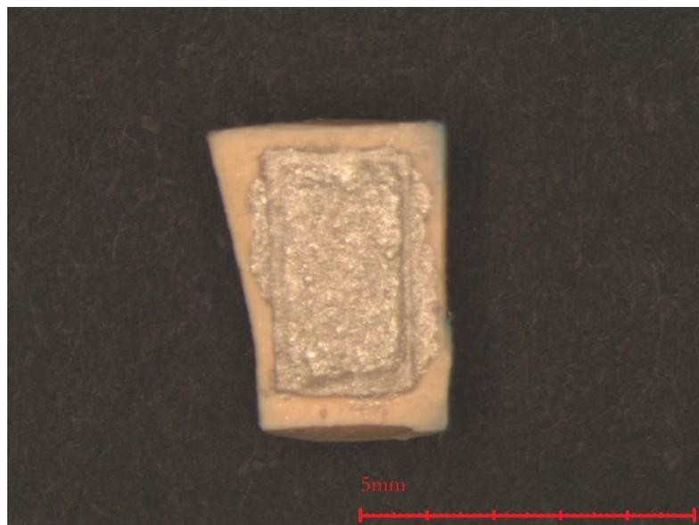
*Figure 4-13 Sample of 3D printed BTMFs/PVDF hybrid material with silver electrodes for dielectric testing*
