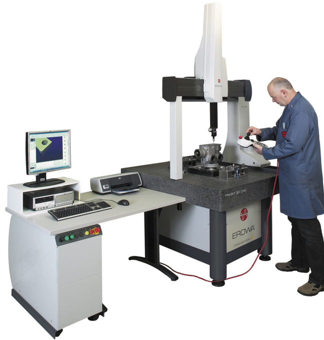
Figure 1.7: An employer analysing the dimensions of an object by using CMM [9]
