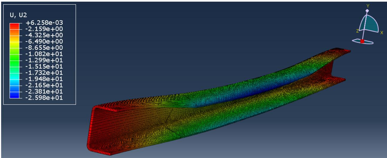
Figure 6.10: Vertical displacement of the composite floor beam.
