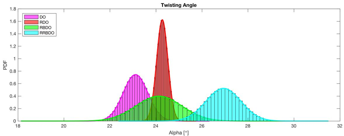
Figure 6.27: Probability distribution functions' comparison of twisting angle results.
