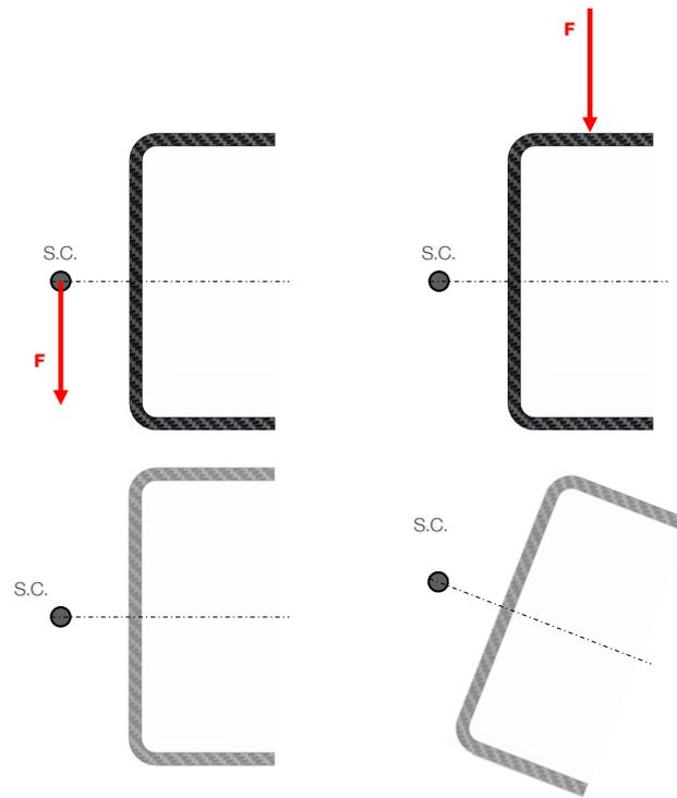
Figure 6.6: Shear centre effect on C shaped beams.
