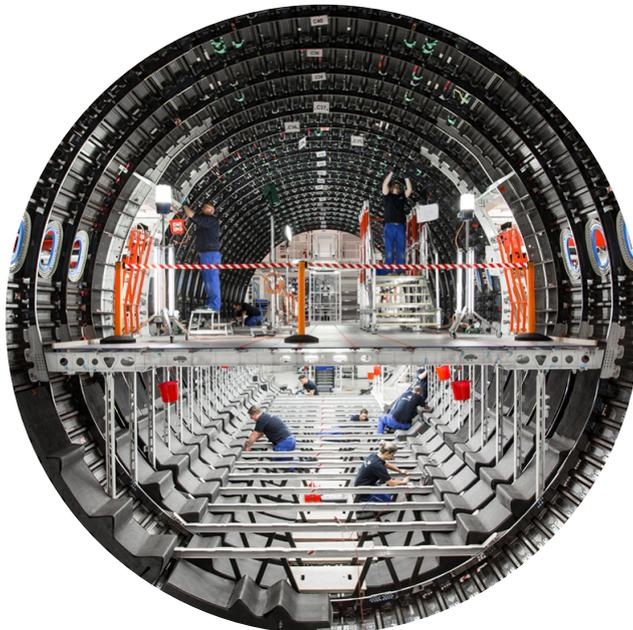
Figure 6.1: Airbus A350 floor beam structure in Aluminium-Lithium.
