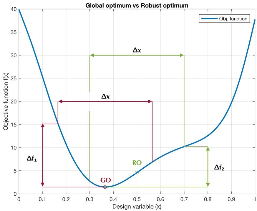
Figure 2.2: Differences between global optimum and robust optimum.
