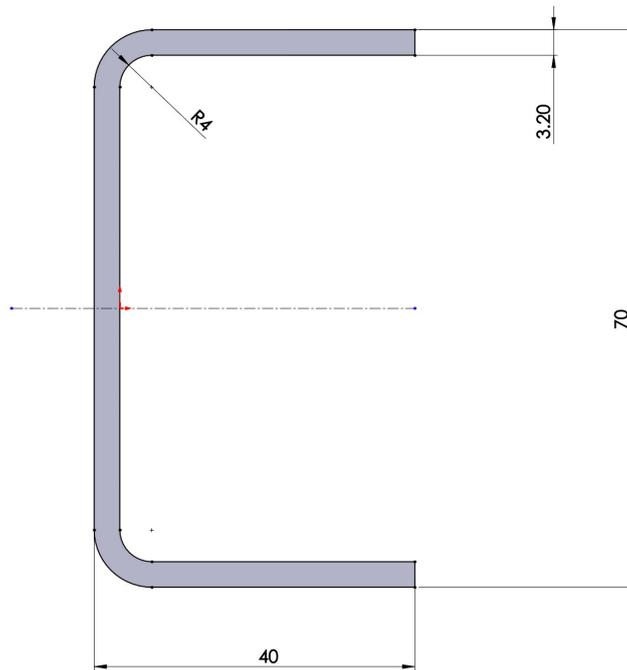
Figure 6.5: Nominal geometry of the cross-section.
