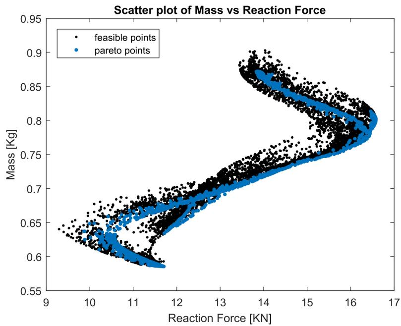
Figure 6.18: Scatter 2D plot of Mass vs Reaction Force, showing Pareto front.
