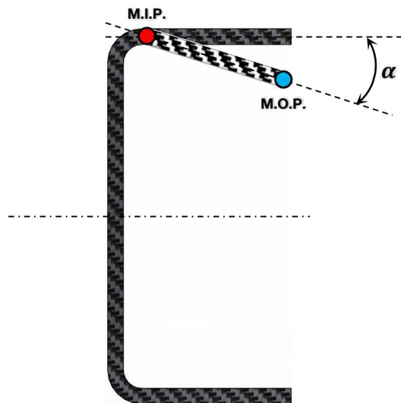
Figure 6.14: Middle section upper flange's rotation ( $\alpha$ ) computed via Middle Inner Point (M.I.P.) and Middle Outer Point (M.O.P.) locations.
