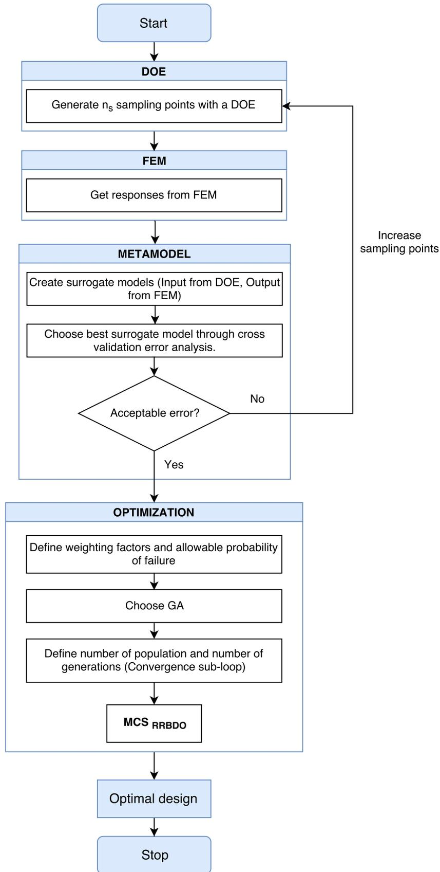
Figure 5.8: Robust and Reliability-Based Design Optimization flowchart.
