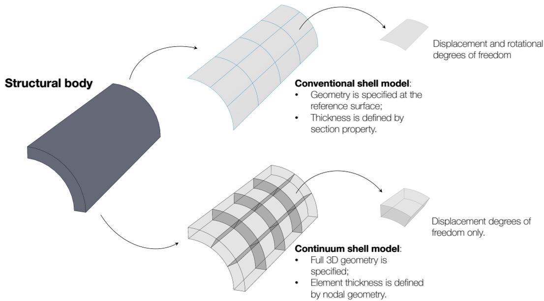
Figure 6.9: Conventional shell model vs Continuum shell model.
