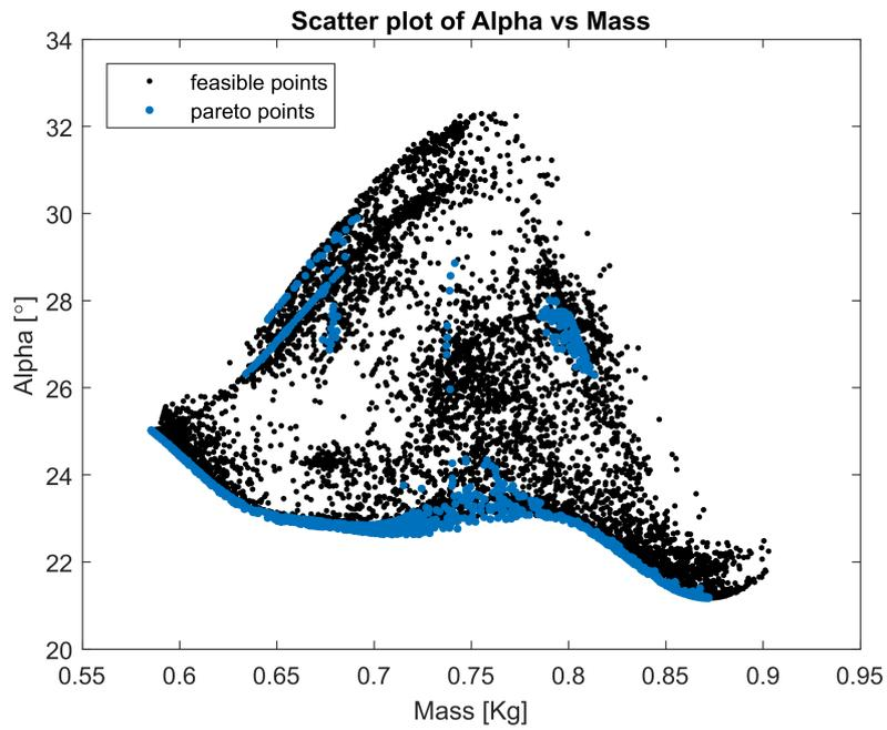
Figure 6.17: Scatter 2D plot of Twisting angle vs Mass, showing Pareto front.
