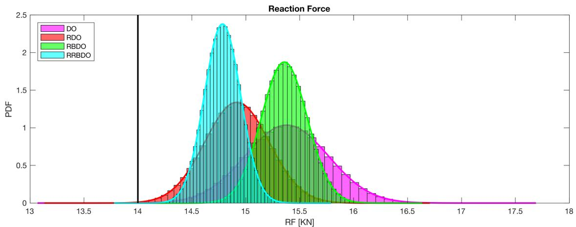
Figure 6.25: Probability distribution functions' comparison of reaction force results, showing limit state value.
