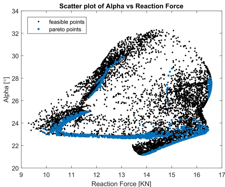
Figure 6.16: Scatter 2D plot of Twisting angle vs Reaction force, showing Pareto front.
