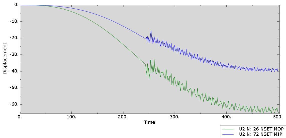
Figure 6.13: Step 3: Vertical displacement of the middle section's upper flange (border points).
