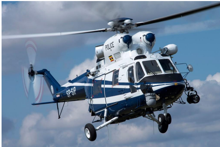
Figure 11 – PZL Kania Police layout with Winch and Searching Lights.
