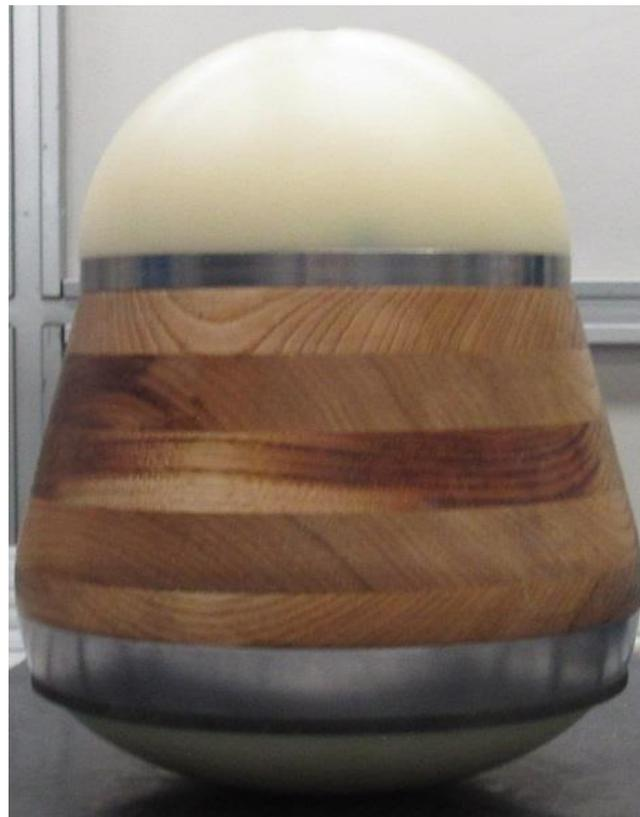
*Figure 24 : 10,2 kg headform used in the tests*
