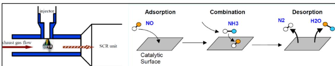
Figure 36 – Catalytic evolution inside SCR catalyst
