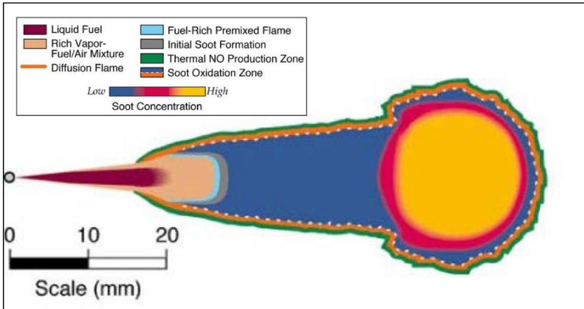
Figure 7 - Quasi-steady diesel combustion plume “Courtesy Dr. John E. Dec (Sandia national laboratories)”
