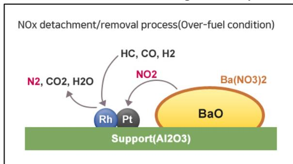
Figure 43 – Nox detachment/removal process
