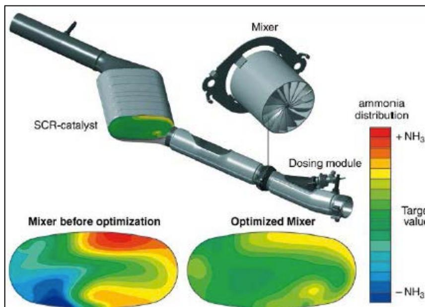
Figure 38 – Mixer for SCR system
