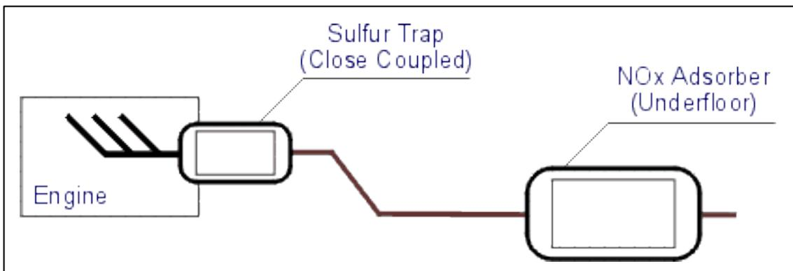
Figure 45 – Sulfur trap + NOx adsorber “www.Dieselgate.com”
