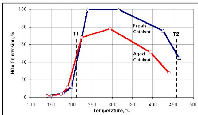
**Chart 23 – Temperature Vs. NO<sub>x</sub> conversion b/w fresh and aged catalyst “www.DieselNet.com”**
