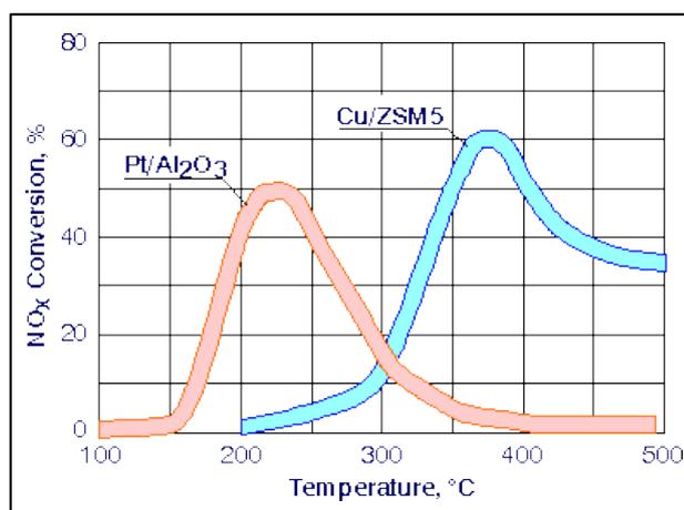
Chart 22 – Temperature Vs NO<sub>x</sub> base on the PGM
