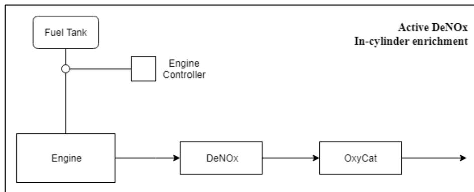
Figure 40 – Active DeNOx (In-cylinder enrichment)
