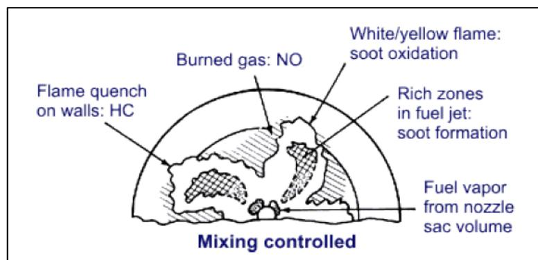
Figure 3 - Mixing controlled phase "Spessa's notes"
