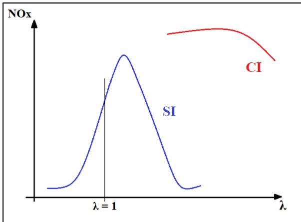
Figure 17 - NO<sub>x</sub> Vs  $\lambda$  compared SI and CI engines
