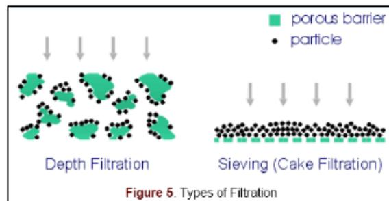
Figure 49 – Mechanism of DPF filtration
