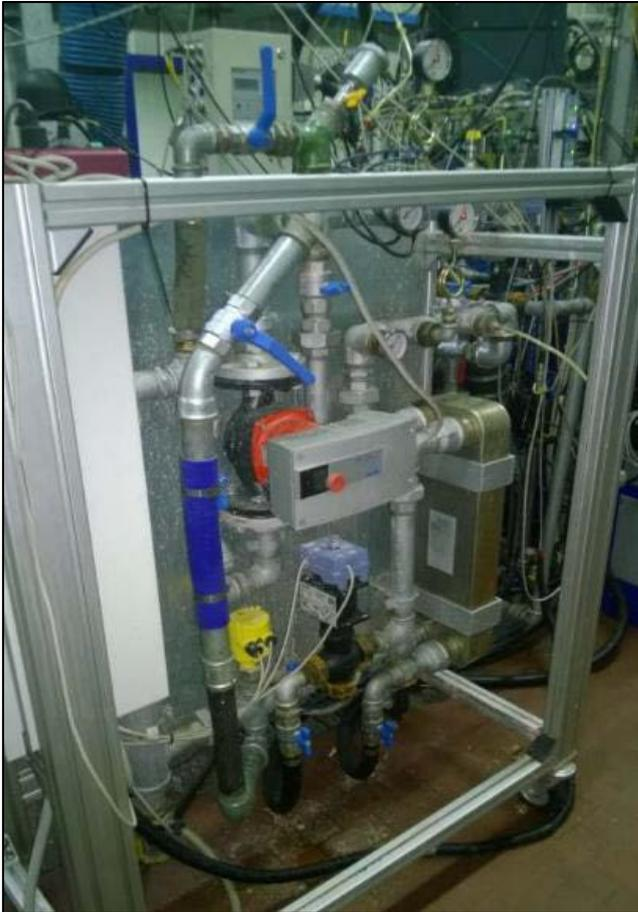
**Figure 63 – Engine cooling fluid system**
