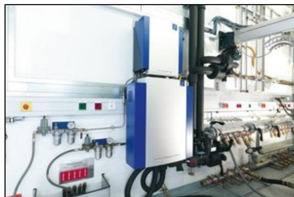
Figure 60 – AVL fuel measurement system KMA 4000
