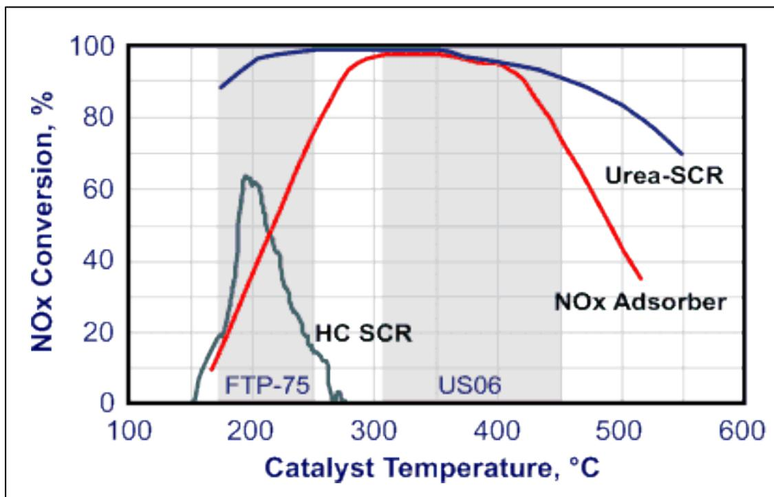
Chart 24 – Catalyst’ conversion efficiency b/w HC SCR, NOx adsorber, Urea-SCR
