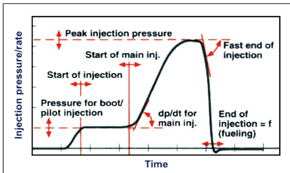
Figure 14 - Injection pressure shape “www.DieselNet.com”
