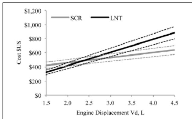
Chart 25 – Engine displacement Vs. SCR and LNT cost “Millo’s notes”
