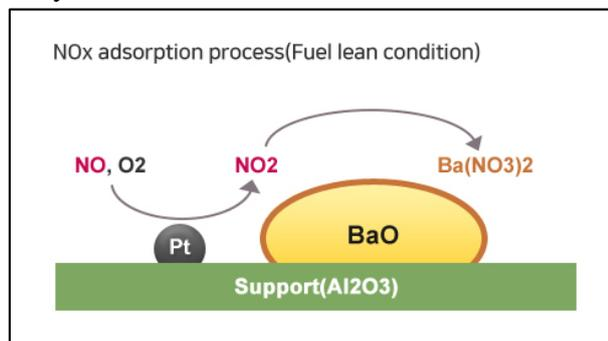
Figure 42 – Nox adsorption process
