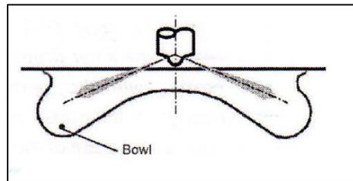
Figure 11 - Injection inside the piston bowl
