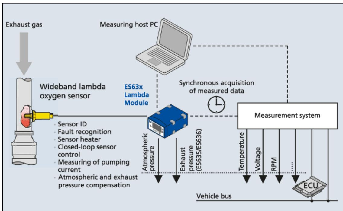
Figure 57 – Scheme of the interconnection b/w the measuring host PC, ECU and lambda sensor
