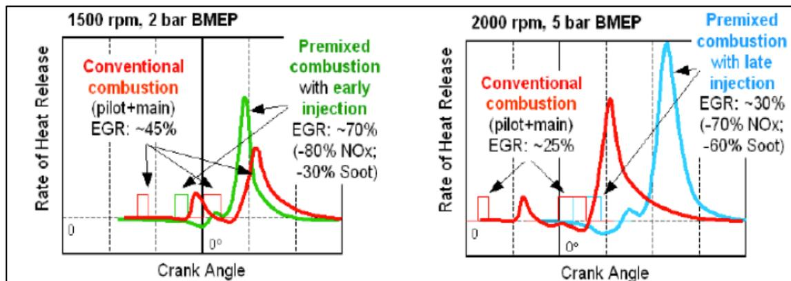
Chart 32 – Rate of Heat release difference b/w Conventional combustion and premixed combustion with early or late injection “Millo’s notes”
