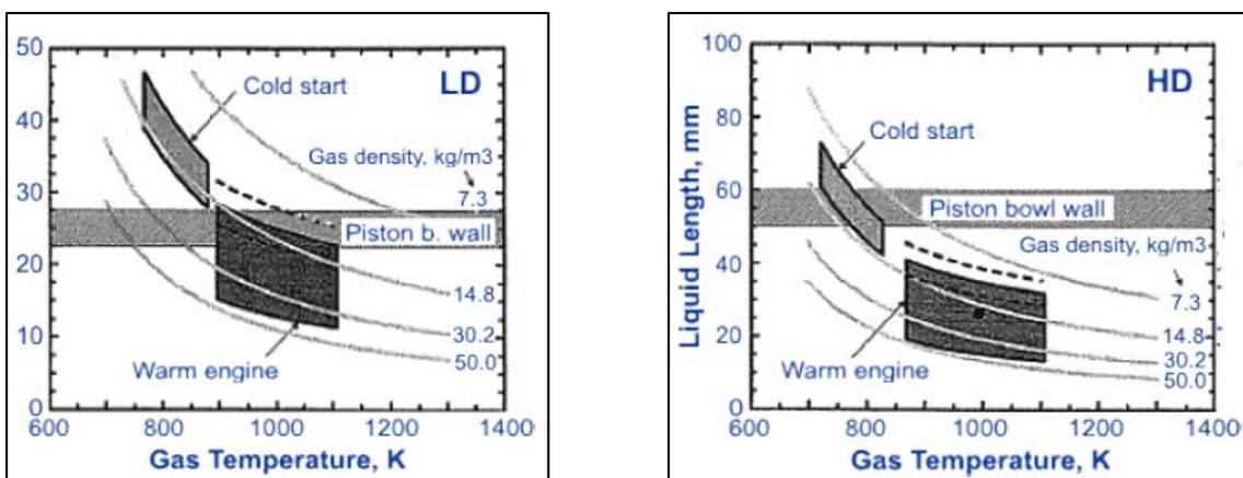
Figure 10 - Liquid length for LD and HD applications “[3]”
