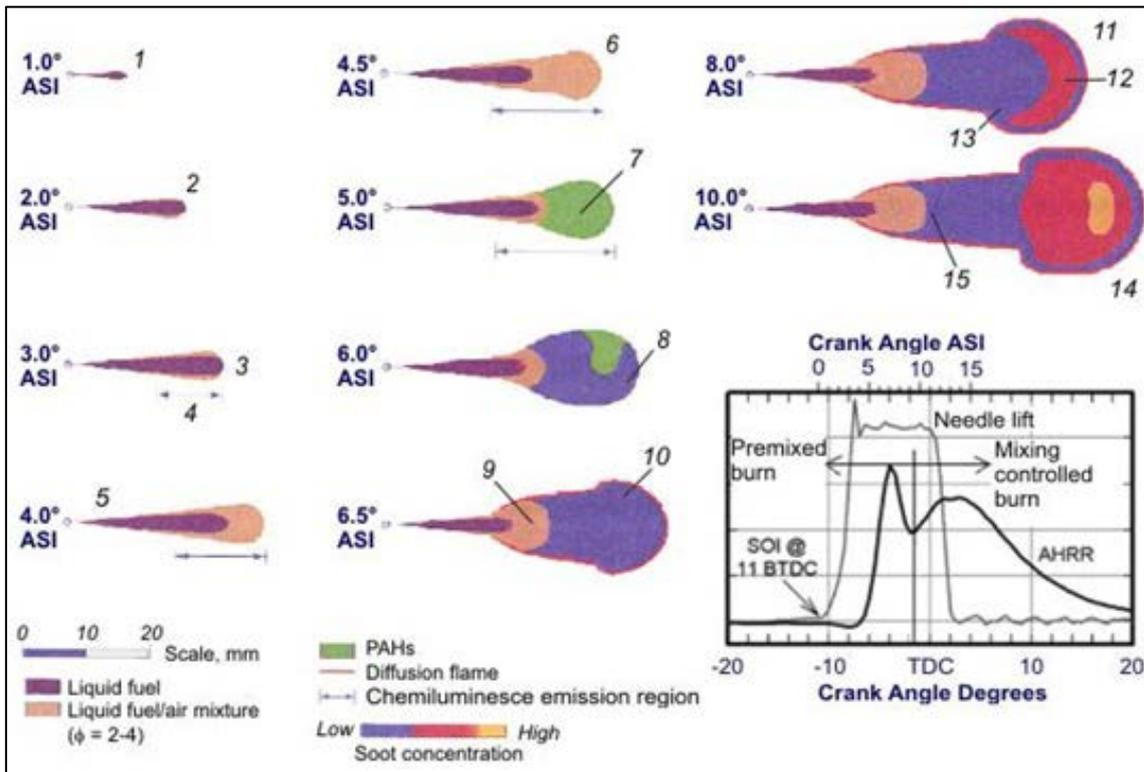
Figure 8 - Combustion plume evolution “www.DieselNet.com”
