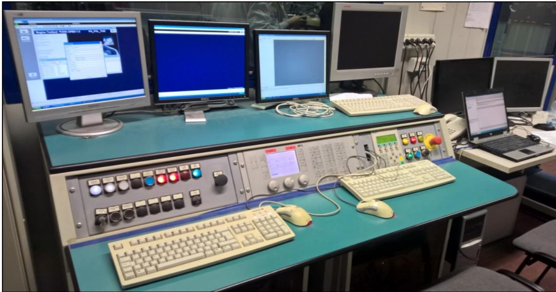
Figure 58 – Engine test bed
