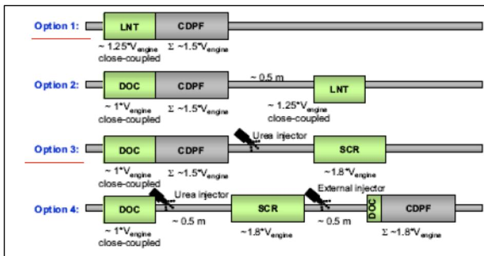
Figure 46 – Different catalyst layouts “[13]”
