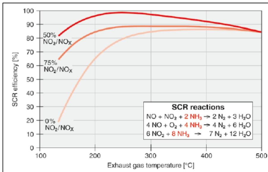
Chart 19 – SCR efficiency Vs. Exhaust gas temperature
