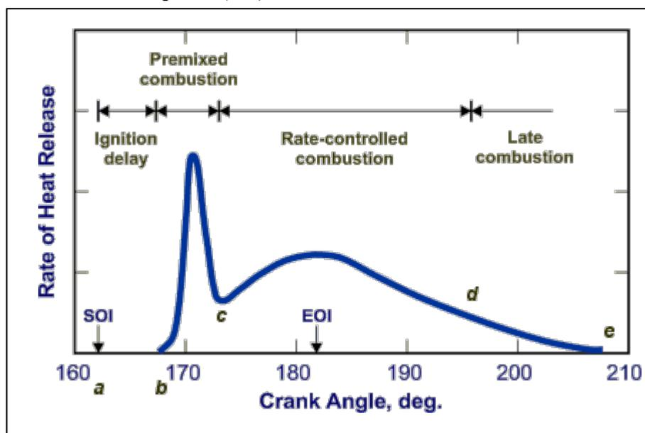
Figure 1 - Rate of Heat Release “www.DieselNet.com”
