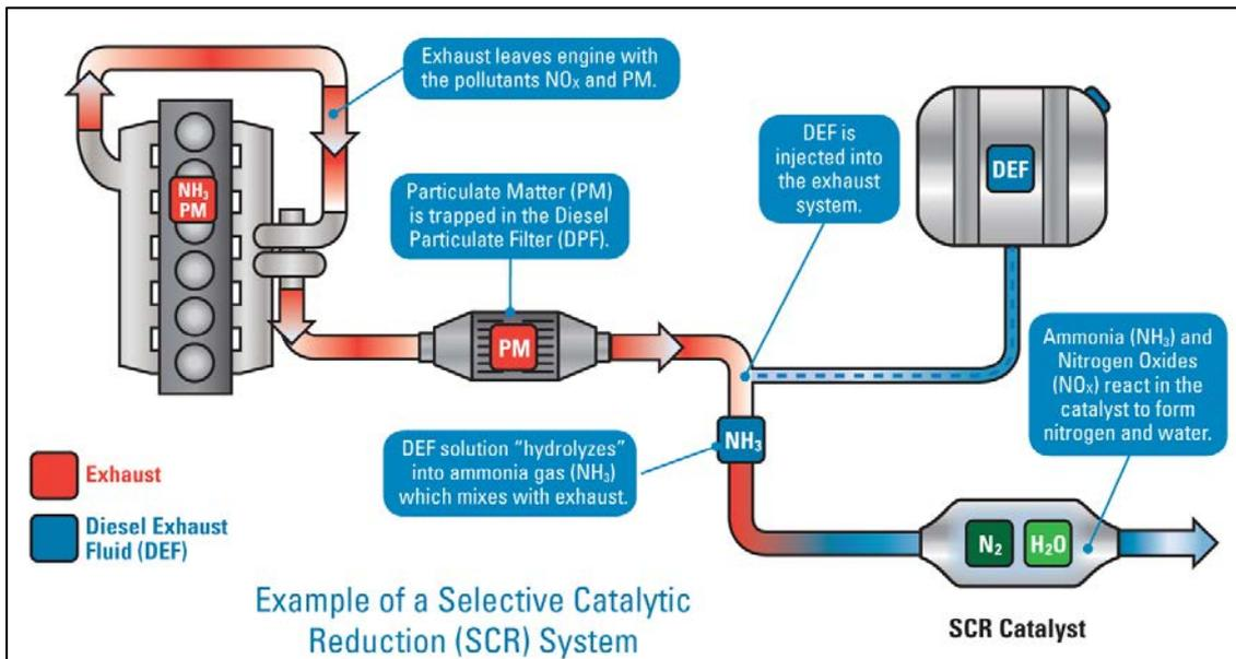
Figure 37 – SCR layout system “www.ThePinsta.com”
