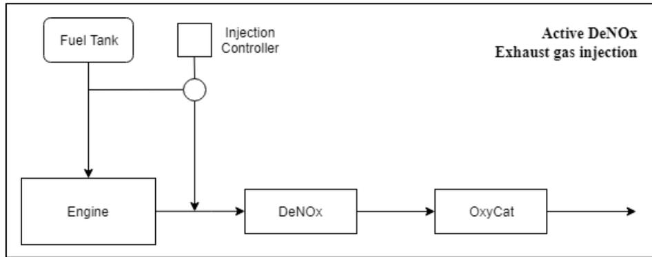
Figure 41 – Active DeNOx (Exhaust gas injection)
