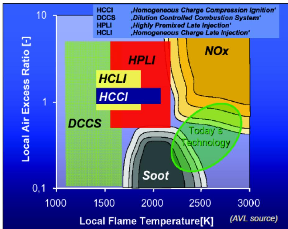
Figure 51 – Different combustion modes on the Kamimoto diagram “AVL”
