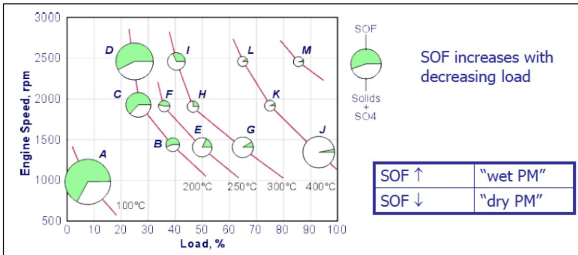
Figure 25 – Composition of soot as a function of load “www.DieselNet.com”
