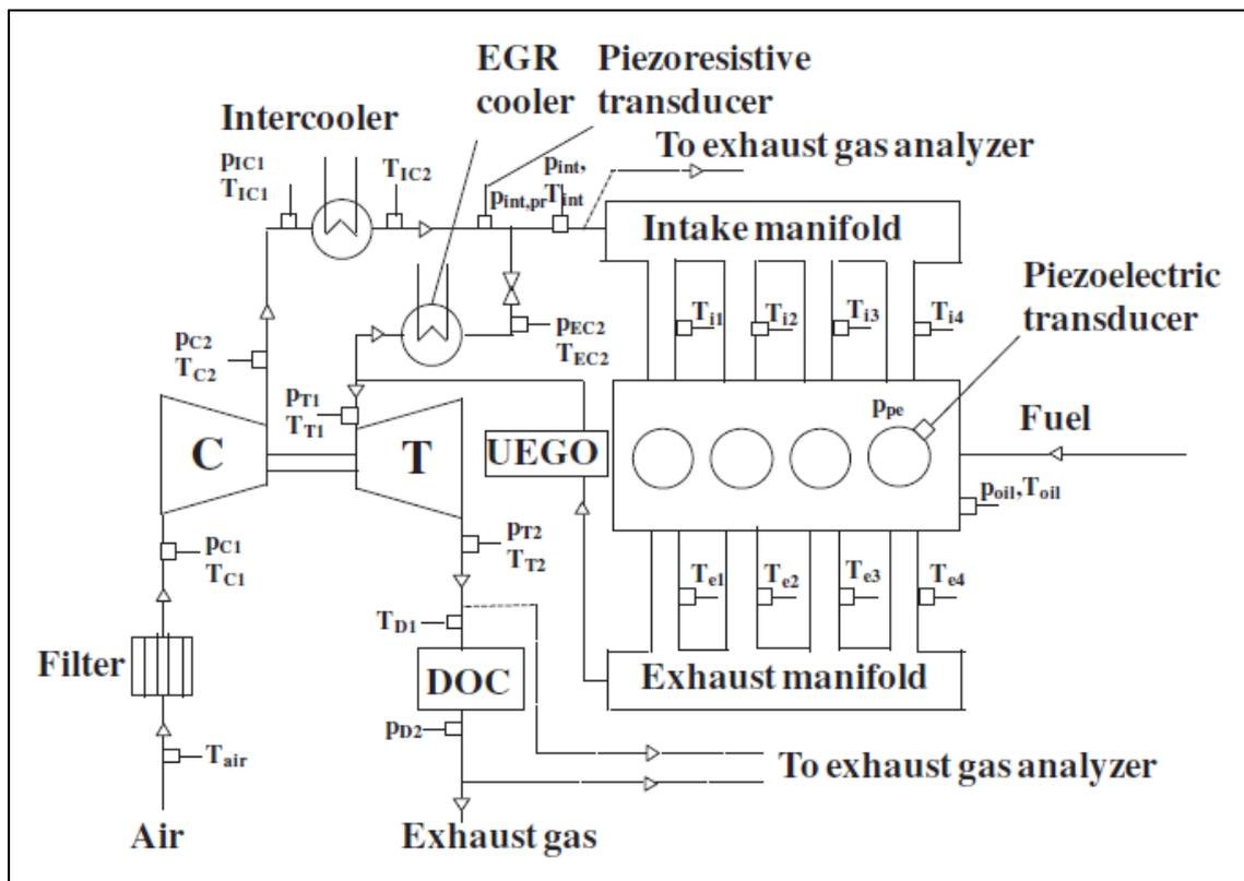
Figure 55 – Scheme of engine instrumentation “[23]”
