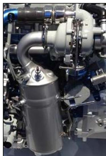
Figure 34 – DOC + DPF mounted on engine
