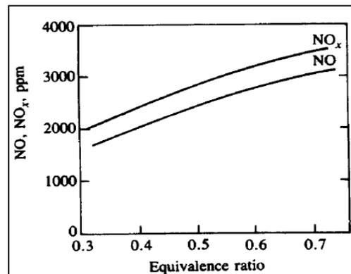
Figure 16 - NO<sub>x</sub> Vs Equivalence ratio
