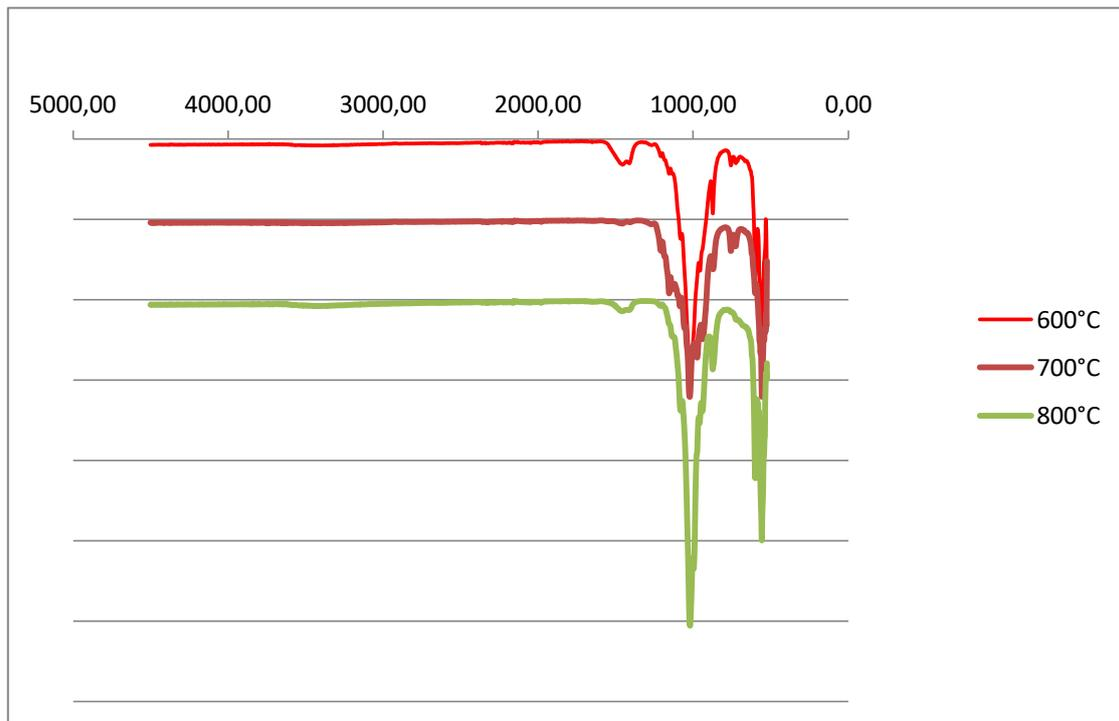
**Fig. 3.15** FTIR curves for sample 3 sintered at 600°C, 700°C and 800°C.
