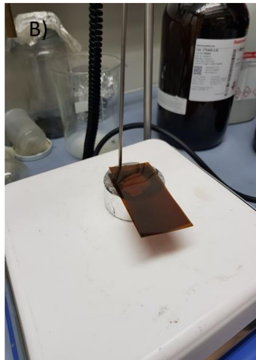
Figure 3. A) PEEK powder with a layer of UPILEX on the heating plate; B) PEEK between two UPILEX's layers before compression
