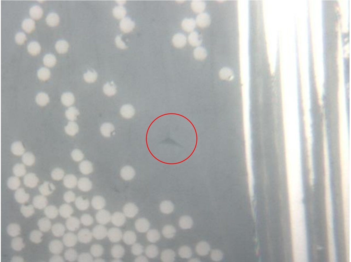
Figure 33. Example of internal footprint; the fibers are they are aligned at 90° or 0°
