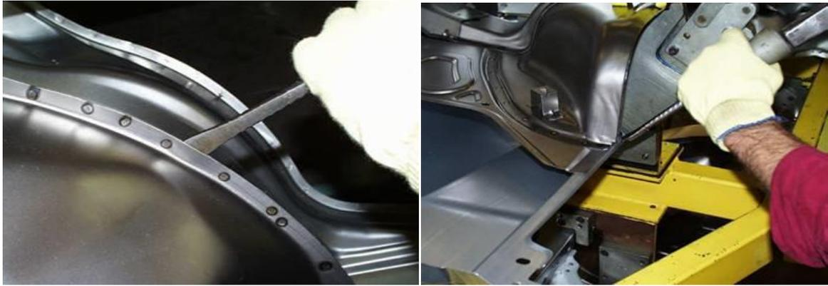
*Figure 28. Hammer and chisel check*
