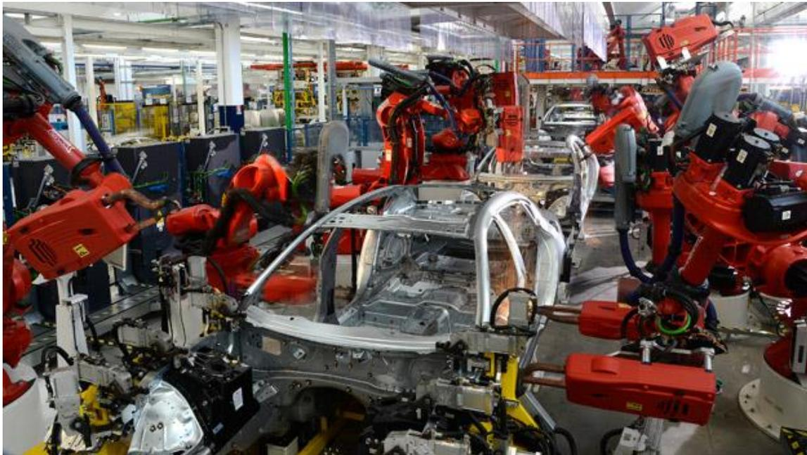
*Figure 5. Resistant Spot Welding in automotive production*
