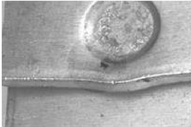
*Figure 16. Excessive indentation*
