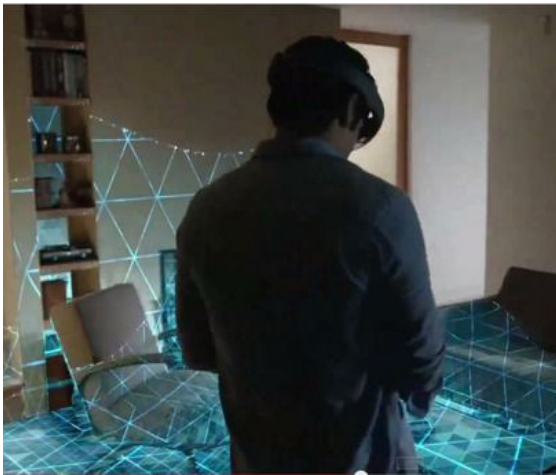
Figure 4.27 Microsoft HoloLens SLAM process. (Image: 36Kr)
