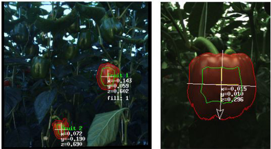
Figure 1.34 Machine vision to recognise ripe peppers. (Image: Sweeper-robot)
