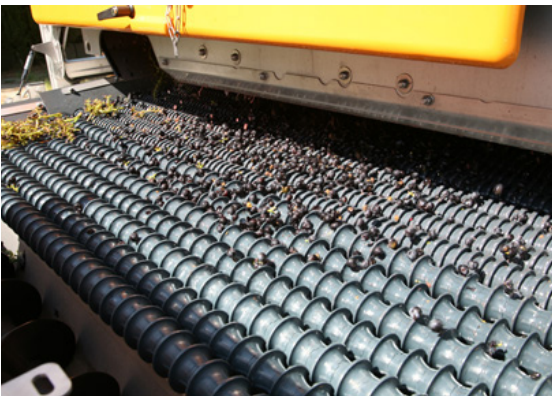
Figure 3.4 Machine sorting ripe berries. (Image: Pellenc)
