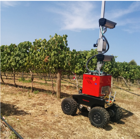
Figure 3.5 Vinbot monitoring grapes on vines. (Image: VINBOT)
