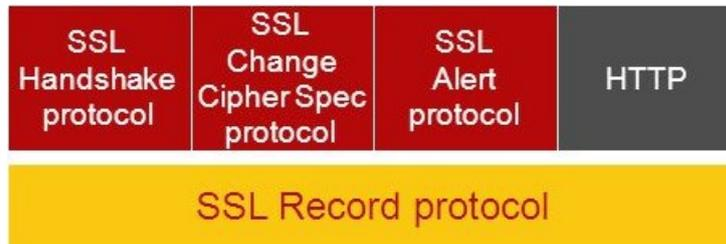
Figura 2.4: Sottoprotocolli SSL/TLS
